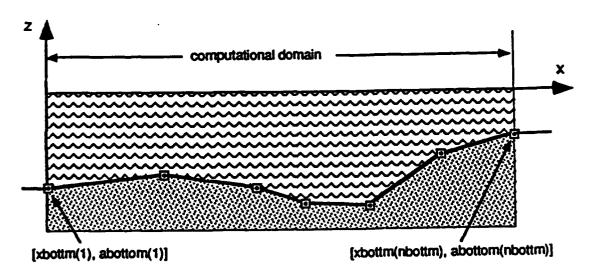
Figure 3. Schematic of the nodes of the polygonal bottom description
