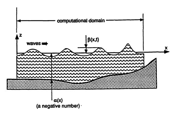
Figure 1. A typical flow for simulation by GNWave
