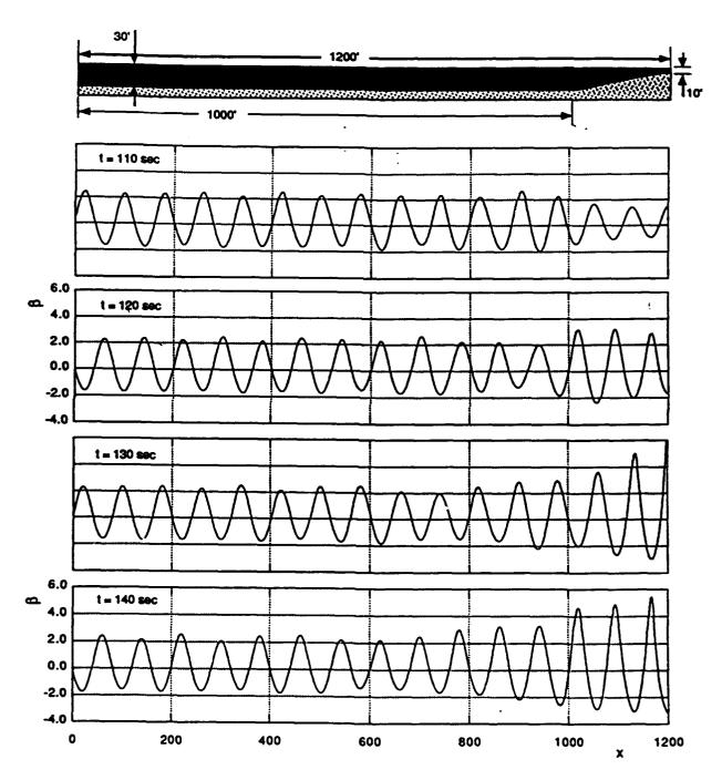
Figure A3. Waves approaching sluice gate (shown at 10-sec intervals)
