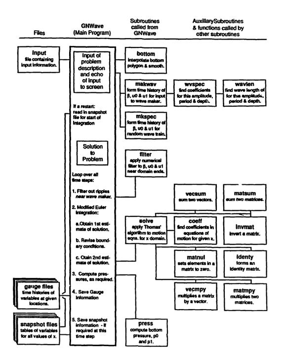
Figure 2. Program level flow chart for GNWAVE
