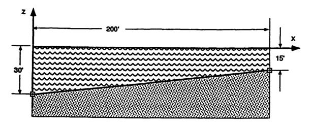
Figure A9. Configuration for test of open boundary condition
