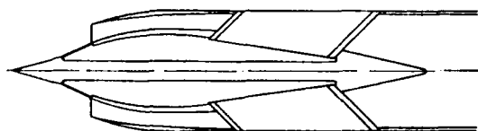
c) Double cone inlet with boundary layer bleed at the cone surface ( \theta_c = 15, 25^\circ )
