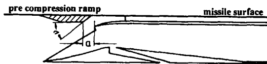
Fig. 32 Geometry of the pre compression ramp
