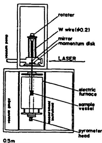
Figure 2. A schematic drawing of the viscometer.
