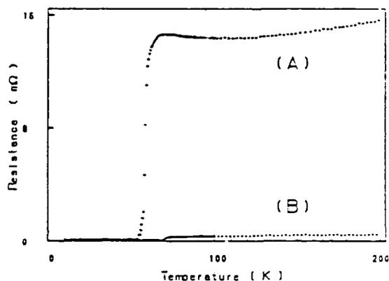
Figure 2. Temperature vs. resistance of the parallel (A) and perpendicular (B) to c-axis for  $\text{EuBa}_2\text{Cu}_3\text{O}_{7.8}$ .
