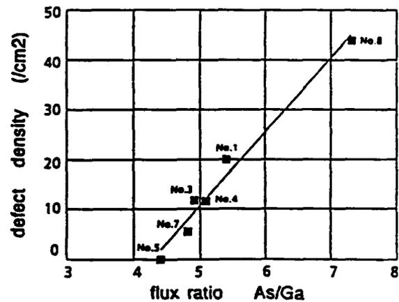
Figure 2. The density of a specific type of defect with varied flux ratio As/Ga.
