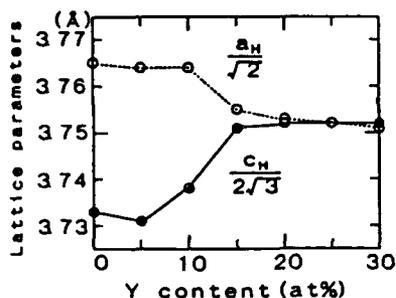
Figure 1. Lattice parameters of Nd<sub>1-x</sub>Y<sub>x</sub>AlO<sub>3</sub>.
