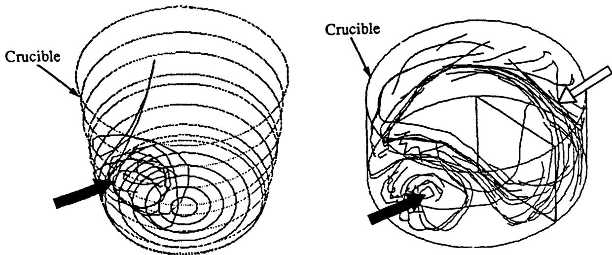
Figure 1. Particle paths from the rotating viewpoint on the crucible: (a) experimentally obtained and (b) numerically calculated.
