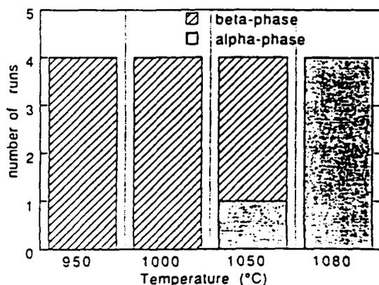
Figure 1. Dependence of phase appearance of  $BaB_2O_4$  crystal on crystallization temperature
