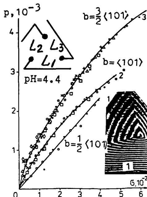
Figure 1. The dependence of the slope of the growth hillock  $p$  on the supersaturation  $\sigma$  for sector 1 for all the studied crystals. Right insert: surface interferogram, upper insert: the center of dislocation step source.
