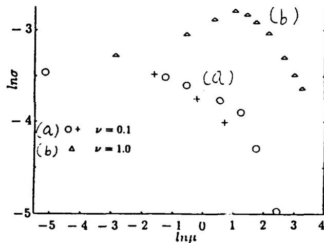
Figure 2. Double logarithmic plot of the stability parameter  $\sigma = v d_0 / 2 D p^2$  versus the strength ratio  $\mu = 2 D p b_0 / d_0$ .
