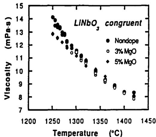
Figure 3. The temperature dependences of the viscosity of  $\text{LiNbO}_3$  doped MgO.
