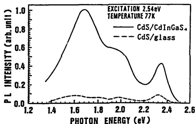
Figure 1. Photoluminescence spectra of CdS/CdInGaS<sub>4</sub> and CdS/glass.
