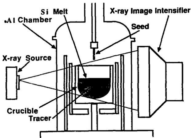
Figure 1. A schematic drawing of experimental setup.
