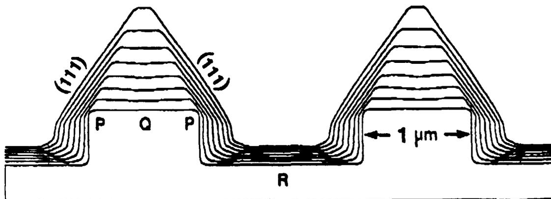
Figure 1. MOVPE growth on GaAs(001) pattered substrate.
