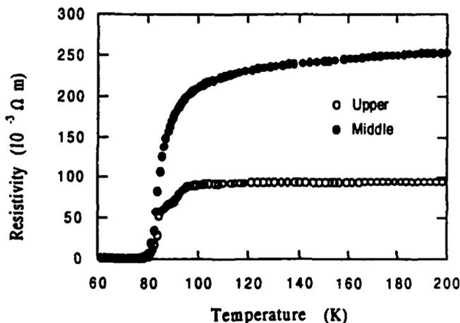
Figure 2. Temperature dependences of resistivity of single crystals.
