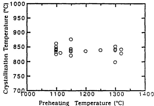
Figure 2. Preheating temperature effect on crystallization temperature of  $BaB_2O_4$
