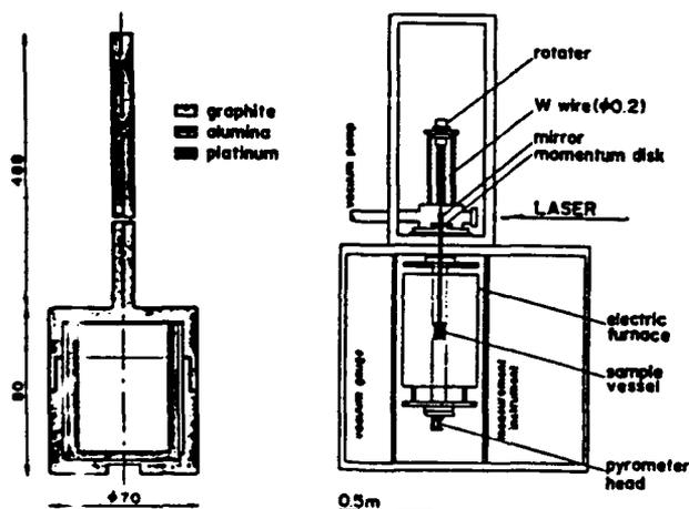
Figure 1. A cross-sectional view of the sample container.
