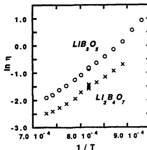
Figure 2. Viscosity of molten  $\text{Li}_2\text{B}_4\text{O}_7$  and  $\text{LiB}_3\text{O}_5$ .
