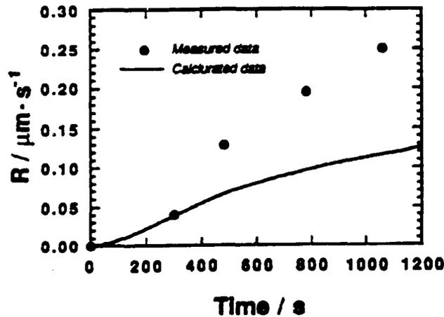
Figure 1. The calculated growth rate based on the diffusion controlling model. The measured values are plotted by close circles.  $R_c = 0.10$  K/min,  $C_0 = 6.5$  mol% acetone.
