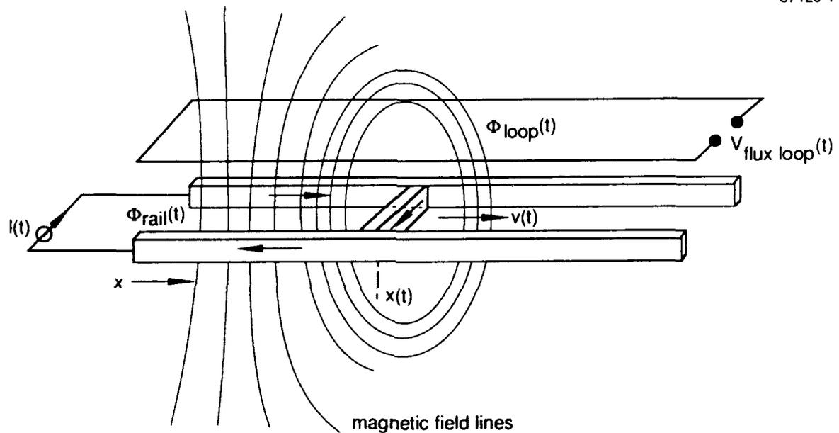
Figure 1 Operating principle of a flux loop diagnostic.
