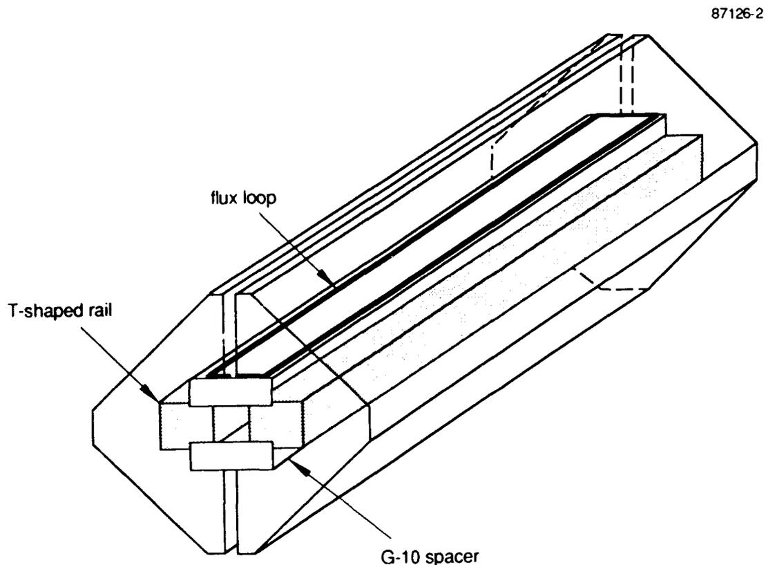
Figure 2 Flux loop diagnostic, incorporated in one of the G10 spacers that hold the T-shaped copper rails of the 1m dipole rail accelerator apart. Only the inner structure of the 1m rail accelerator is shown.
