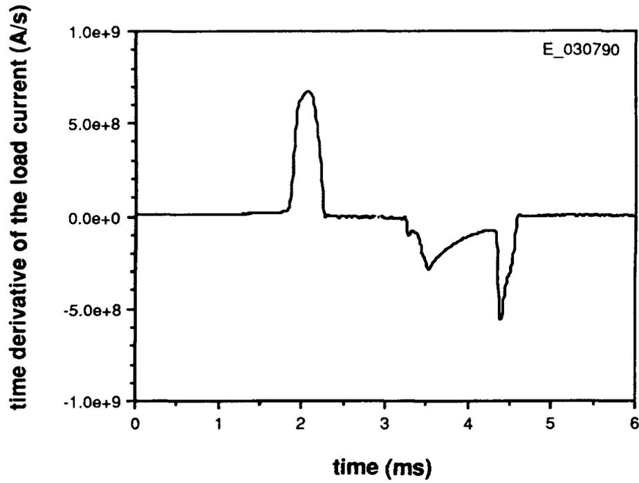
Figure 4 Derivative of the load current during a 1m dipole rail accelerator experiment.
