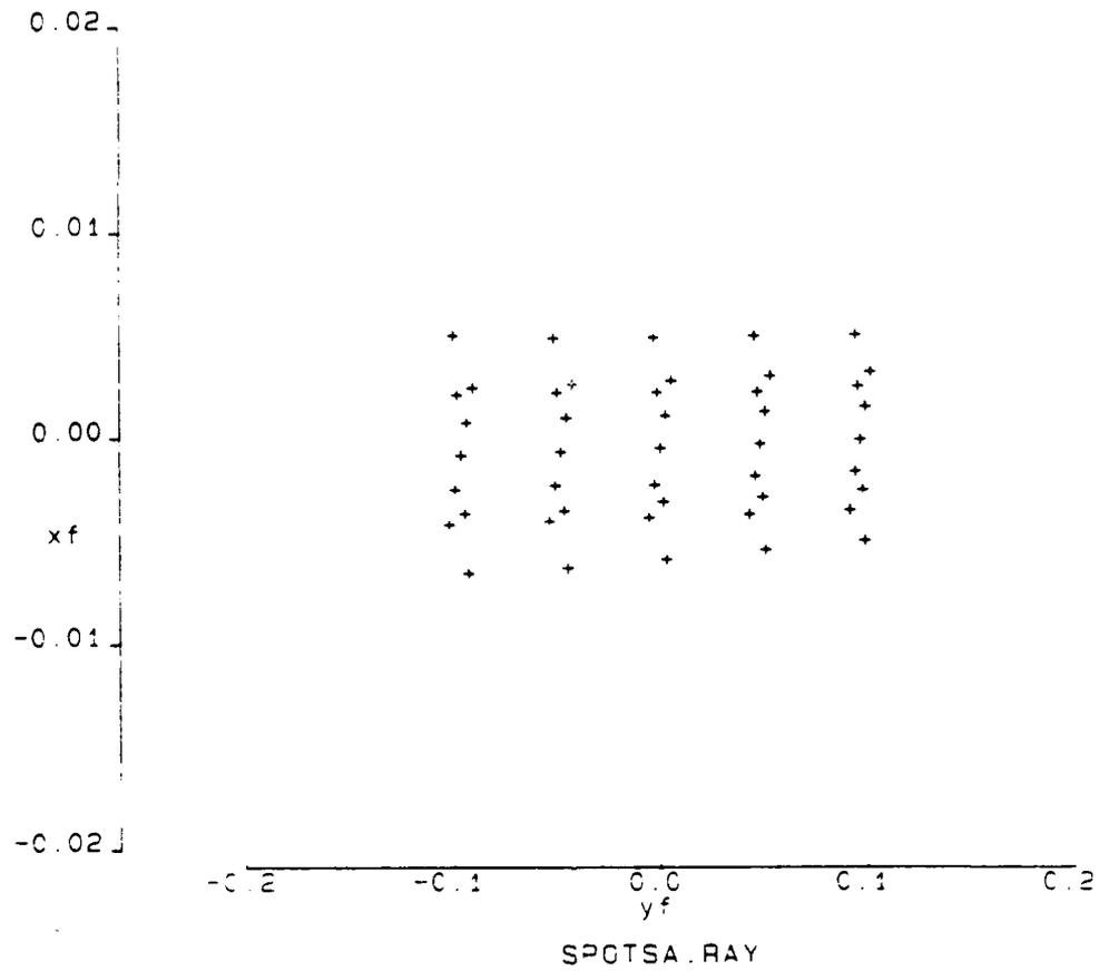
Figure G-6 Simulated Line Spread Function for P45 Mask 2 Horizontal Slit
