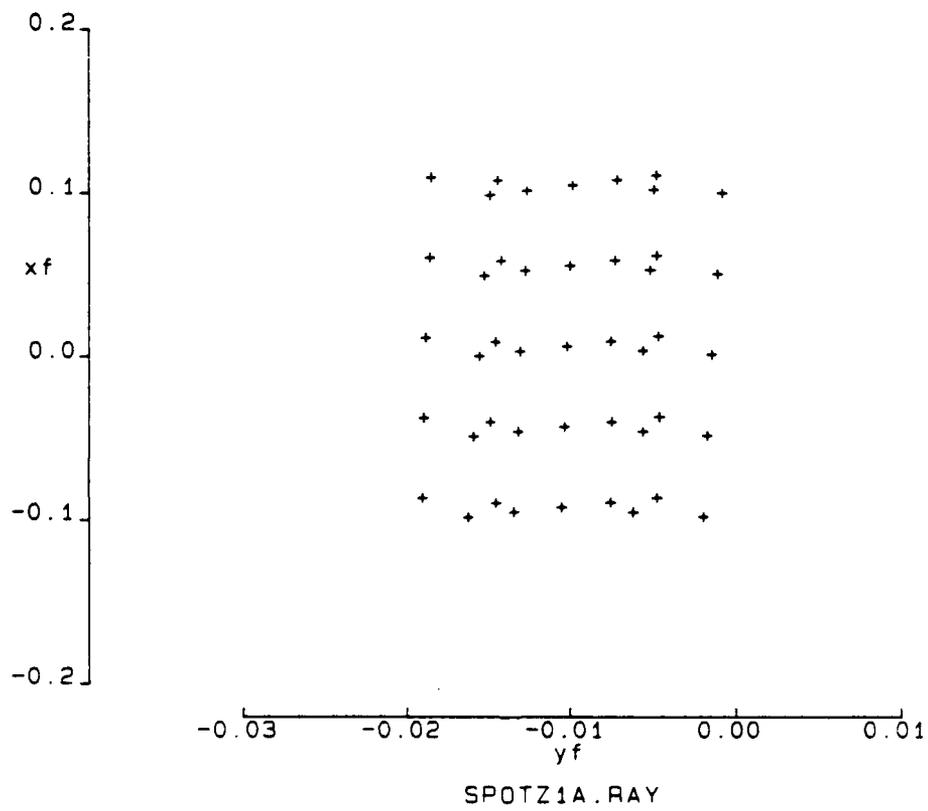
Figure G-3 Simulated Line Spread Function for P45 Mask 1 Vertical Slit
