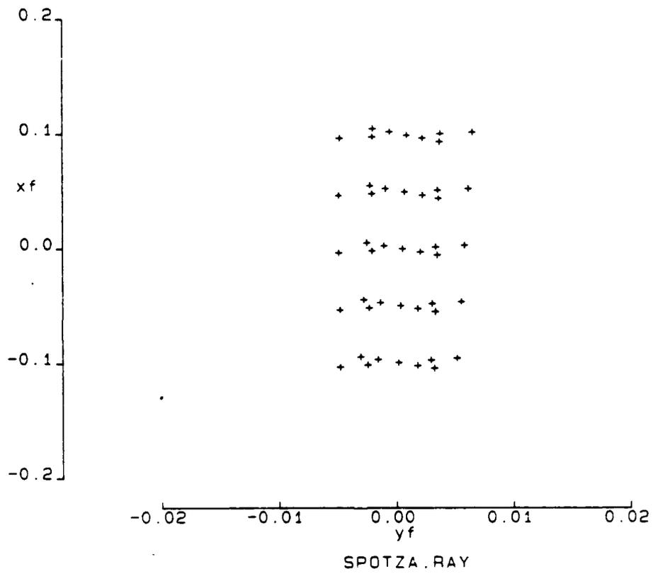
Figure G-5 Simulated Line Spread Function for P45 Mask 2 Vertical Slit
