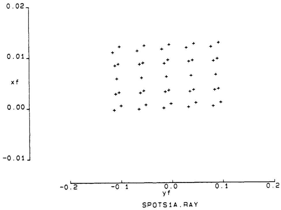
Figure G-4 Simulated Line Spread Function for P45 Mask 1 Horizontal Slit
