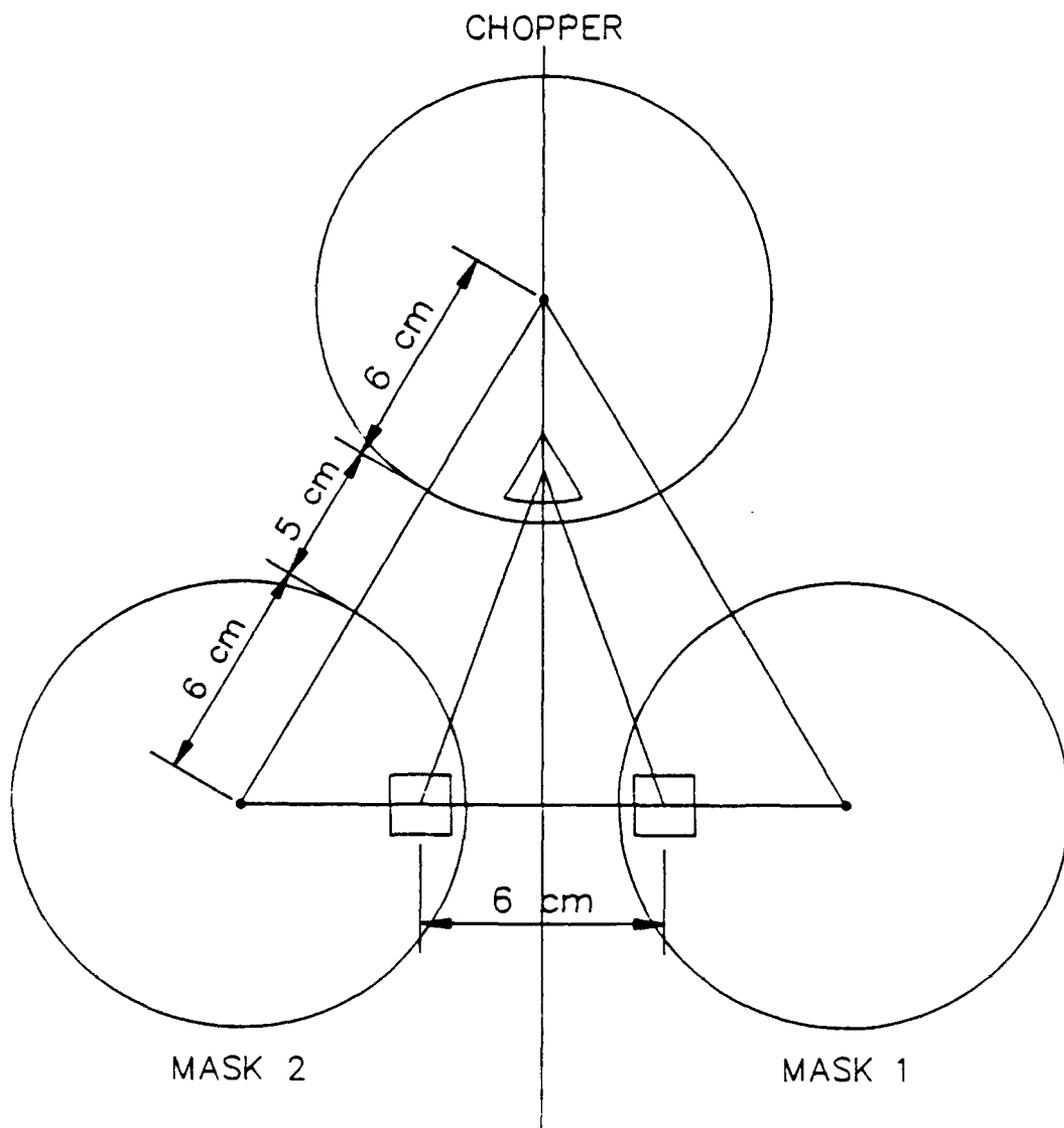
Figure 4 Plane Containing the Chopper and Two Encoding Masks
