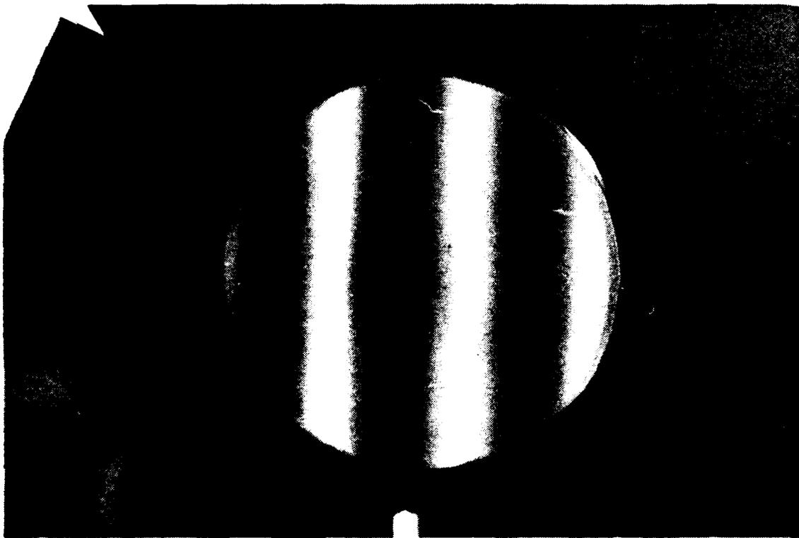
Figure B-4 Ronchigram of Mirror 1 at a Distance Equal to its Radius of Curvature ( $R_1$ ) + 15 mm from the Reticle and the Entrance Slit
