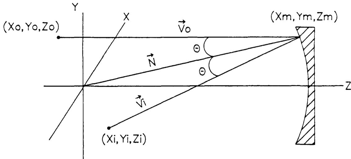
Figure 2 Reflection From a Spherical, Concave Mirror
