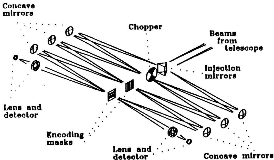
Figure 1 Schematic of New Instrument Configuration
