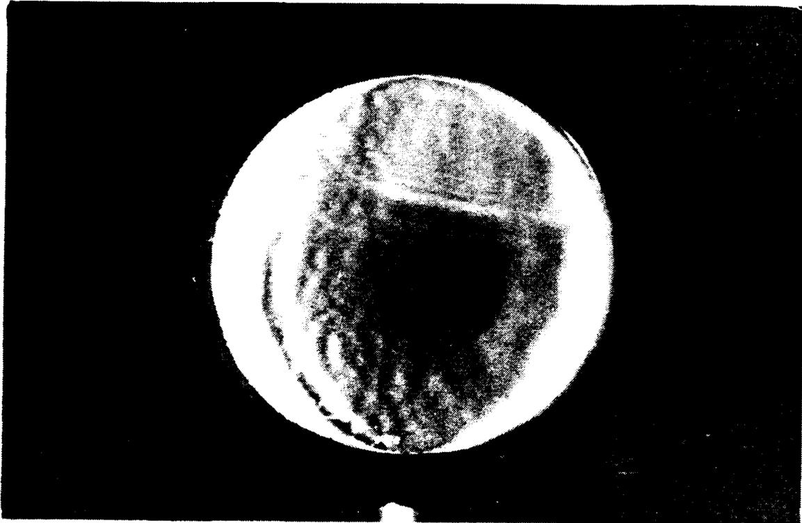
Figure C-1 Ronchigrams of Mirror 2 at a Distance Equal to its Radius of Curvature ( $R_2$ ) from the Reticule and the Entrance Slit
