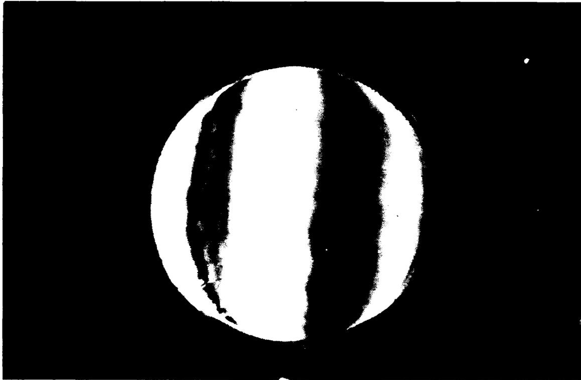
Figure C-3 Ronchigram of Mirror 2 at a Distance Equal to its Radius of Curvature ( $R_2$ ) + 10 mm from the Reticle and Entrance Slit
