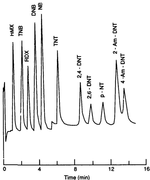
Figure 10. HPLC separation of high explosives using an LC-8 packed column (7.5 cm  $\times$  4.6 mm, with 3- $\mu$ m particles, 70.7/27.8/1.5 H<sub>2</sub>O/MeOH/THF [v/v/v] eluent at 2.0 mL/min). (From Miyares and Jenkins 1991.)
