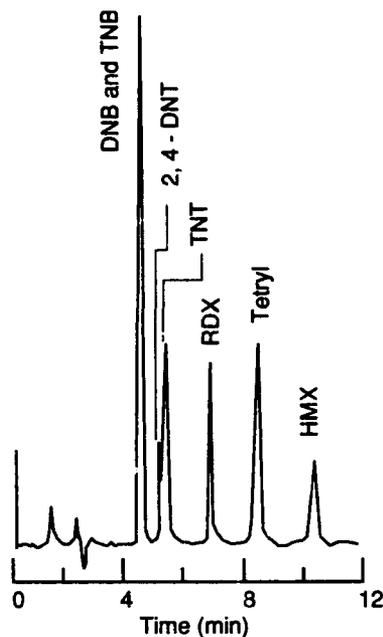
Figure 9. HPLC separation of high explosives using an LC-CN packed column (25 cm  $\times$  4.6 mm, with 5- $\mu$ m particles, 50/50 MeOH/H<sub>2</sub>O [v/v] eluent at 1.5 mL/min). (After Jenkins and Walsh 1987, Jenkins et al. 1988, 1989.)
