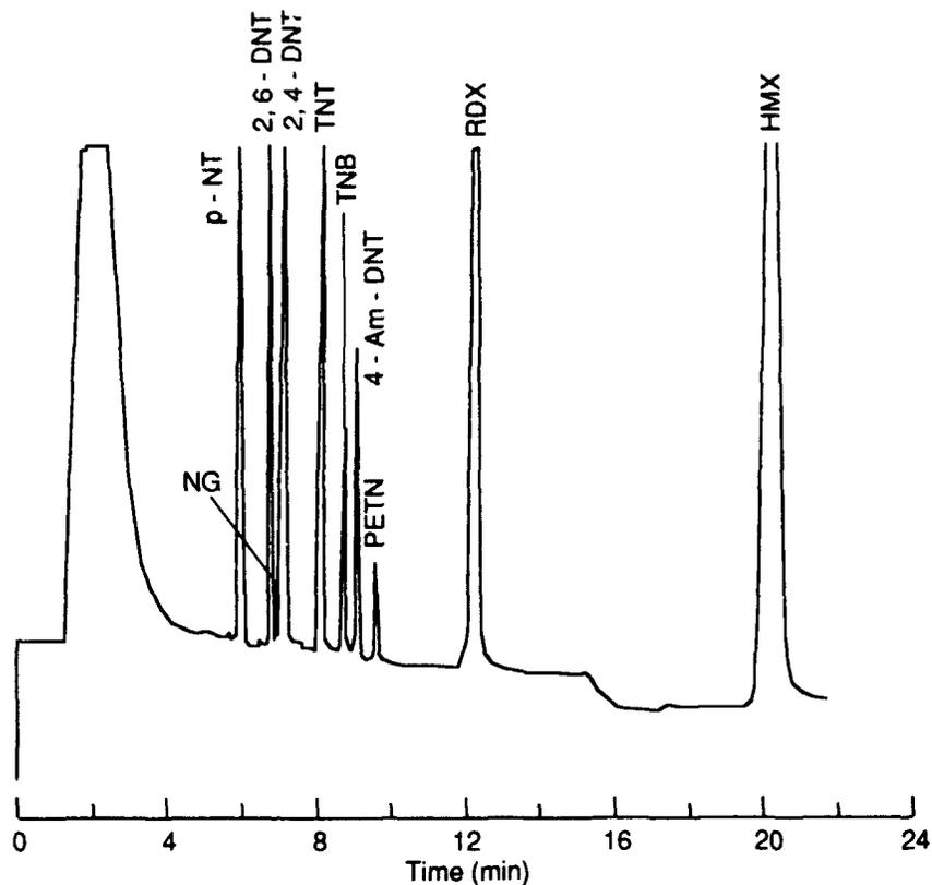
Figure 8. HPLC separation of high explosives using an LC-18 packed column (25 cm x 4.6 mm, with 5- $\mu$ m particles, 50/50 [v/v] MeOH/H<sub>2</sub>O at 1.5 mL/min). (After Jenkins and Walsh 1987, Jenkins et al. 1988, 1989.)
