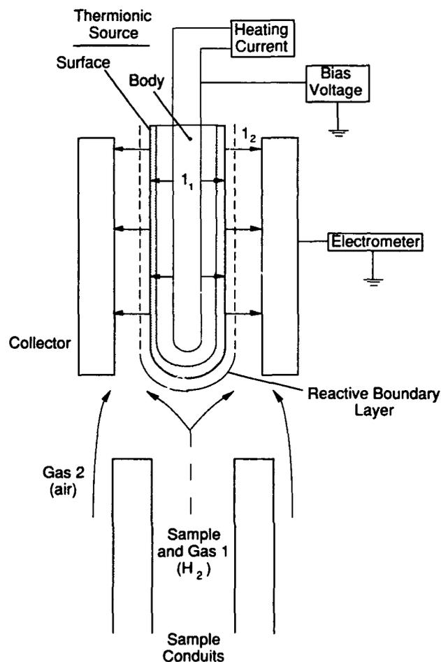
Figure 12. Schematic of the TID-2-H<sub>2</sub>/air detector. (After Patterson 1986.)
