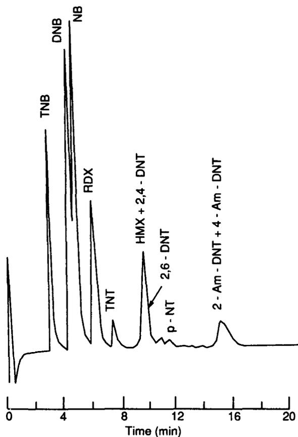
Figure 11. HPLC separation of high explosives using LC-8 and LC-CN columns in series (both 3.3 cm x 4.6 mm, with 3- $\mu$ m particles, 70.7/27.3/1.5 H<sub>2</sub>O/MeOH/THF [v/v/v] eluent at 1.5 mL/min). (From Miyares and Jenkins 1991.)
