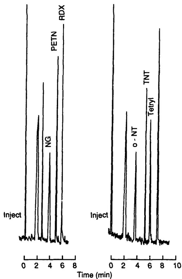
Figure 1. Separation of high explosives using an SB-Octyl 50 Superbond cross-linked flexible silicon capillary column (6.8 m  $\times$  0.05 mm ID). (After Douse 1988.)
