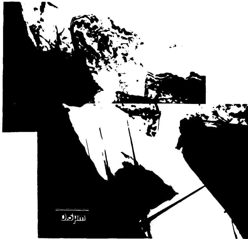
Figure 11. TEM Micrograph of Si Platelets. Twinned Si platelets next to a SiC particulate, with the region next to the SiC particulate and the Si platelets heavily dislocated with well defined subgrains.
