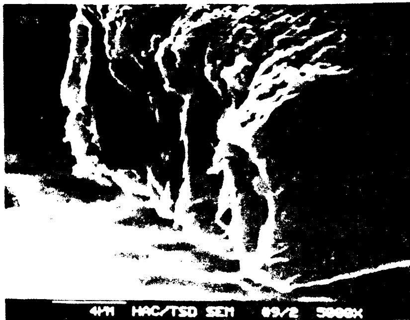
Figure H-35. SEM View of Wire End at Pin 2 Bond Showing Detail of Fracture Face
