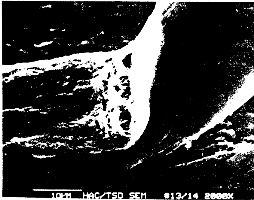
Figure H-57. SEM View of Sample #13 Pin 14 Bond Before Current Cycling at Temperature
