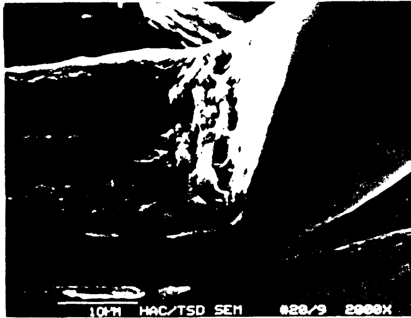
Figure H-69. View of Sample 20 Pin 9 Wire Bond Before Current Pulsing
