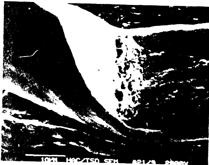
Figure H-84. Another View of Sample 21 Pin 9 Wire Bond Before Current Pulsing
