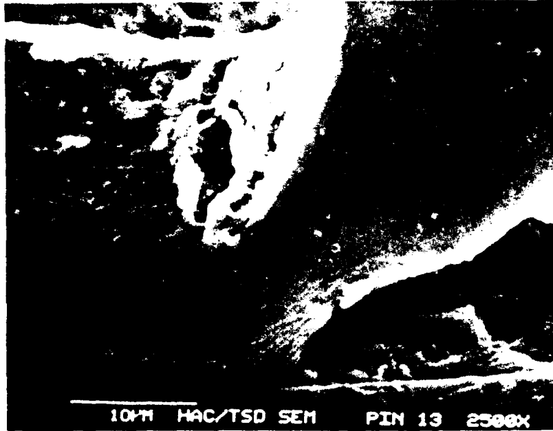
Figure H-3. Sample No. 6. SEM Photo of Heel of Wire Bond at Pin 13, Before Cycling
