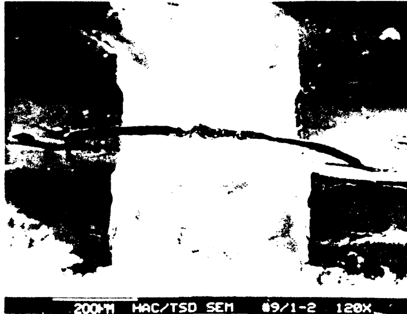
Figure H-30. SEM View of Pin 1-2 Wire After Current Cycling. The Wire Opened at the Pin 2 Bond Heel. Note the Thermal Damage to the Center of the Wire.
