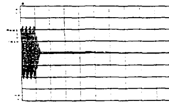
Figure 5 Transient Response of a Smart Beam Featuring Piezoelectric Actuator with Finite Voltage
