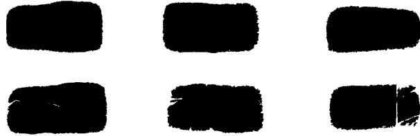
FIGURE 2. X-ray radiograph showing undamaged and damaged embedded piezoceramic wafers in the insulating glass/epoxy plies.
