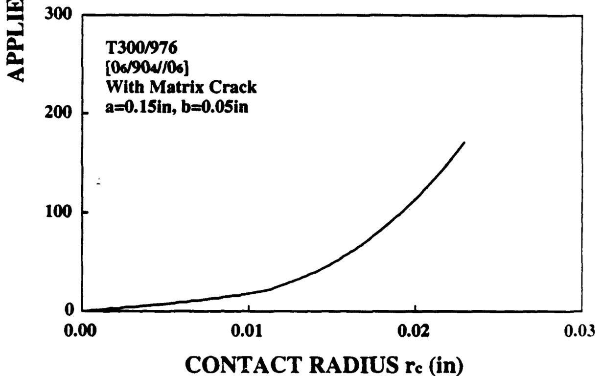
Figure 7. The responses of a [0<sub>6</sub>/90<sub>2</sub>]<sub>s</sub> composite containing a pre-introduced delamination and surface matrix crack and subjected to transverse loading resulting from a spherical indenter.
