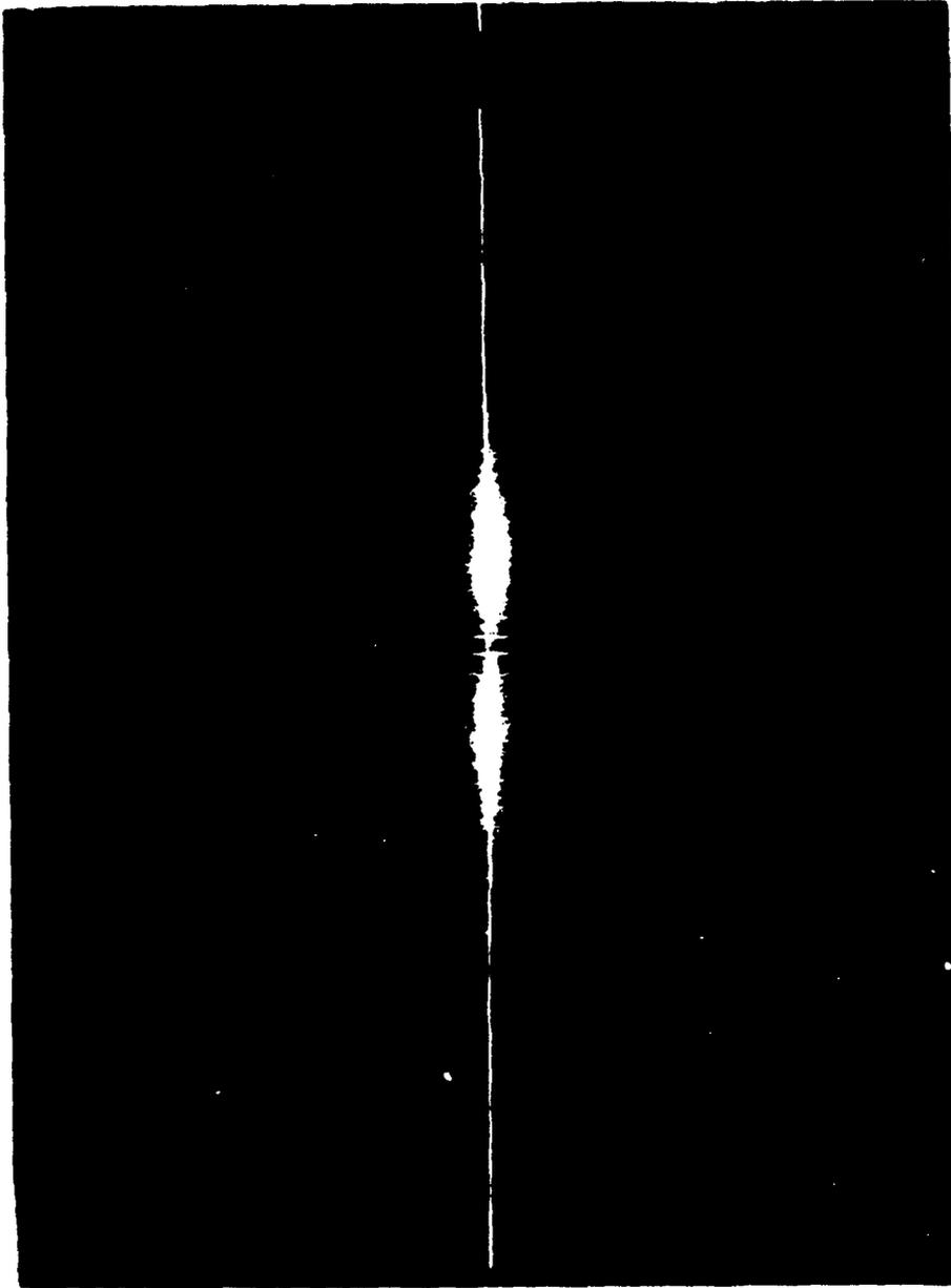
Figure 2. An X-Radiograph of a graphite/epoxy [0<sub>6</sub>/90<sub>2</sub>]<sub>s</sub> composite resulting from a quasi static transverse loading. Data taken from Ref. 5.
