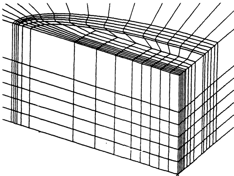
Figure 5. Description of a typical finite element mesh.
