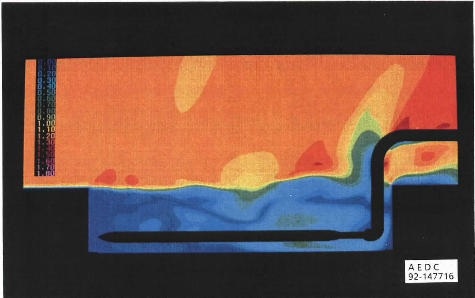
Figure 36. Mach number contours in the symmetry plane of the cavity with the store/sting, M_\infty = 1.20 , Z_s/H = 0.75 .
