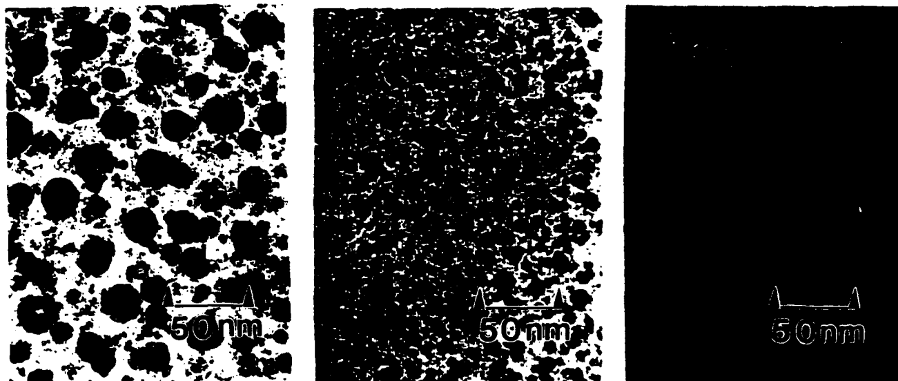
Figure 2. Bright field TEM images of Cu nanoclusters for samples implanted with 12 \times 10^{16} , 6 \times 10^{16} , and 3 \times 10^{16} ions/cm 2 (left to right).
