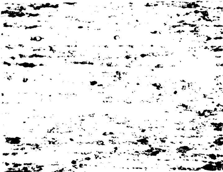
Figure 9a. Conventional powder alloy, L-ST section.
