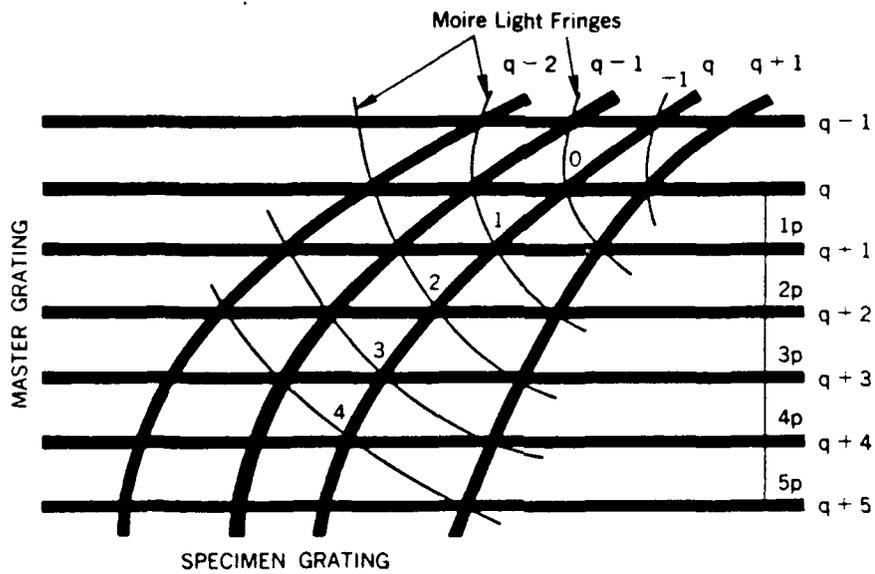
Figure 4. Moire fringes (schematic) produced by combination of pitch change and rotation, (Ref. 1).
