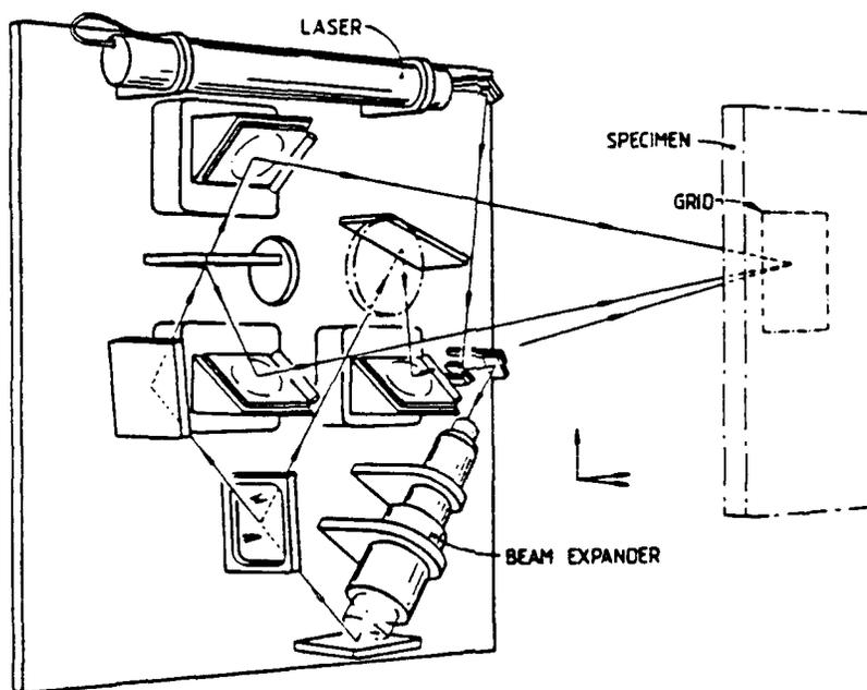
Figure 14. Folded three beam optical arrangement (Ref. 74).
