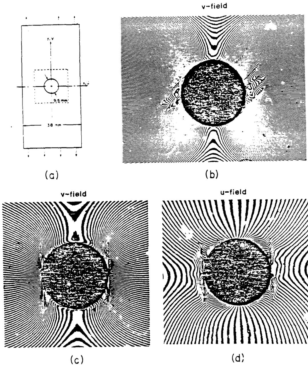
Figure 25. Displacement fields in fatigue - damaged graphite/epc  $\langle y \rangle$  composite specimen. (a) specimen geometry, (b) 45-deg. top ply, (c) and (d) 0-deg. top ply (Ref. 49).
