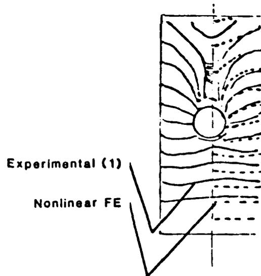
Figure 39. Experimental/numerical comparison of pin-loaded 0/90 glass/epoxy specimens, (Ref. 61).
