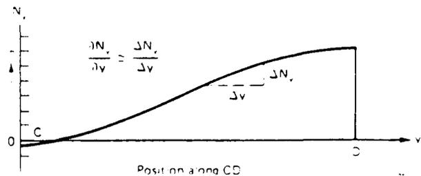
Figure 5. Illustration of procedure to obtain the four Cartesian fringe derivatives from the two Cartesian fringe patterns, (Ref. 4).
