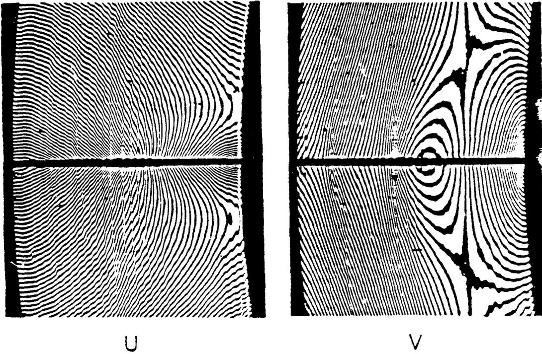
Figure 41. Residual strain, relieved by slicing and under-cutting a thick composite, (Ref. 69).
