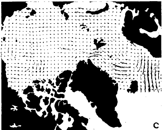
Fig. 13. The surface-forced barotropic circulation for the month of September 1986: (a) with ice-water drag forcing (maximum velocity 1.9 \text{cm s}^{-1} ), (b) with direct wind stress forcing (maximum velocity of 4.5 \text{cm s}^{-1} ), (c) wind stress field.
