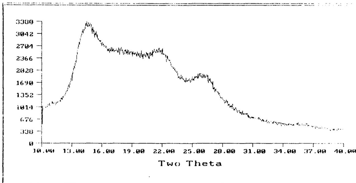
Figure 27. X-Ray Crystallography Plot of Uncoated Kapton.
