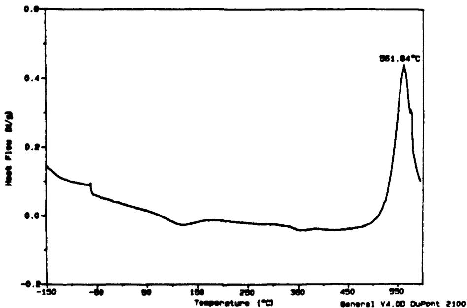
Figure 6. DSC Tracing of IP-200 PPQ.
