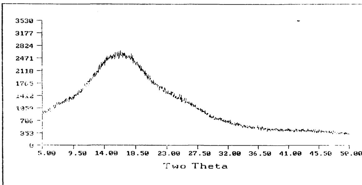
Figure 28. X-Ray Crystallography Plot of Uncoated EYMYD L-30N.
