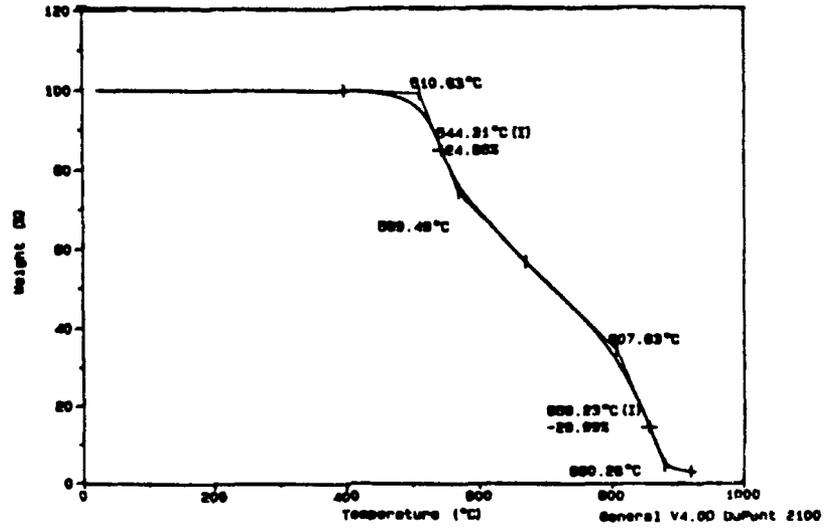
Figure 3. TGA Tracing of E-MYD L-30 in Vacuum.
