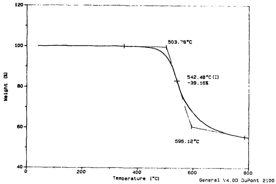
Figure 1. TGA Tracing of EMYD L-30N in Nitrogen.
