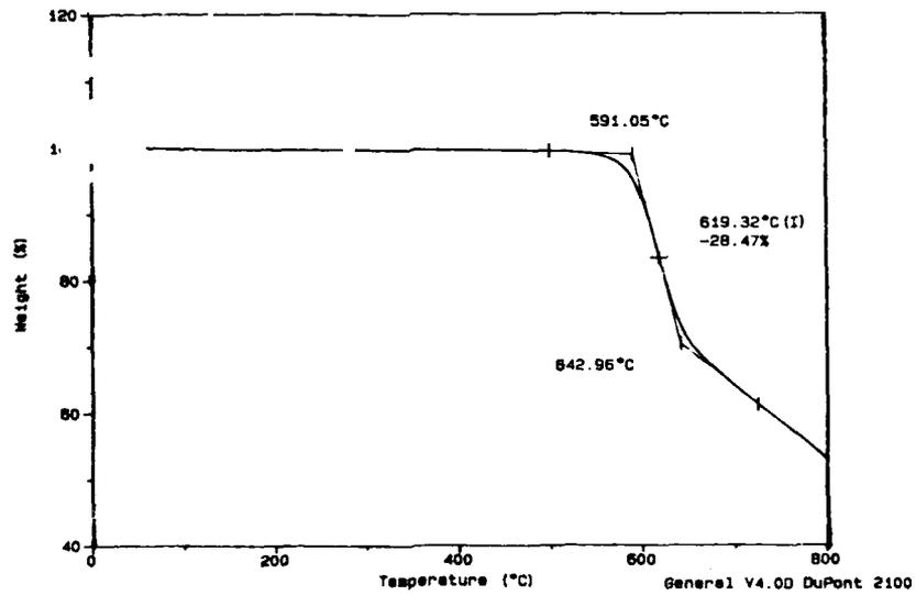
Figure 4. TGA Tracing of UPILEX S in Vacuum.
