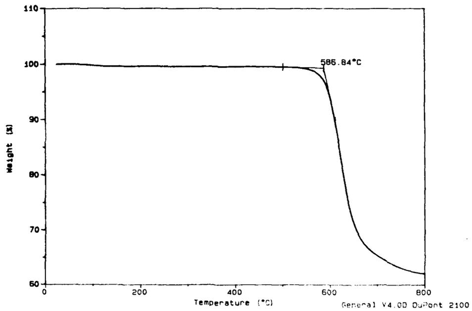
Figure 2. TGA Tracing of UPILEX S in Nitrogen.
