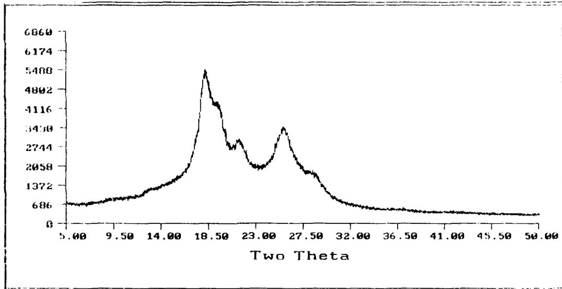
Figure 32. X-Ray Crystallography Plot of 2500 Angstroms SiO<sub>2</sub> Coated UPILEX S.
