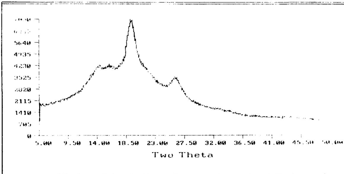
Figure 31. X-Ray Crystallography Plot of 2500 Angstroms SiO<sub>2</sub> Coated EYMYD L-30N.
