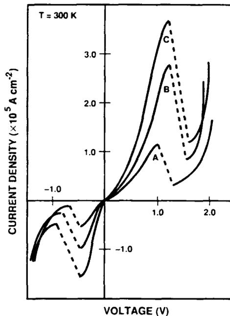
FIG. 2. Experimental current density vs voltage characteristics at room temperature for the three samples studied. At positive bias the peak current densities are  $1.1 \cdot 10^5$ ,  $2.7 \cdot 10^5$ , and  $3.7 \cdot 10^5 \text{ A cm}^{-2}$ , and the best peak-to-valley current ratios were 3.5, 3.3, and 3.2 for samples A, B, and C, respectively.
