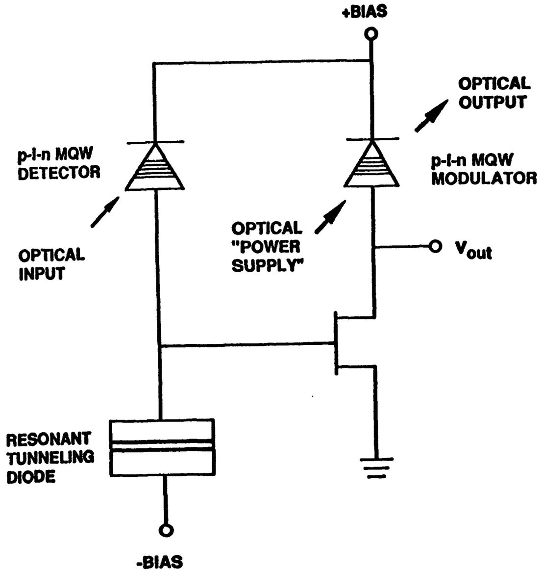
Figure 1 The circuit of the monolithic optoelectronic transistor
