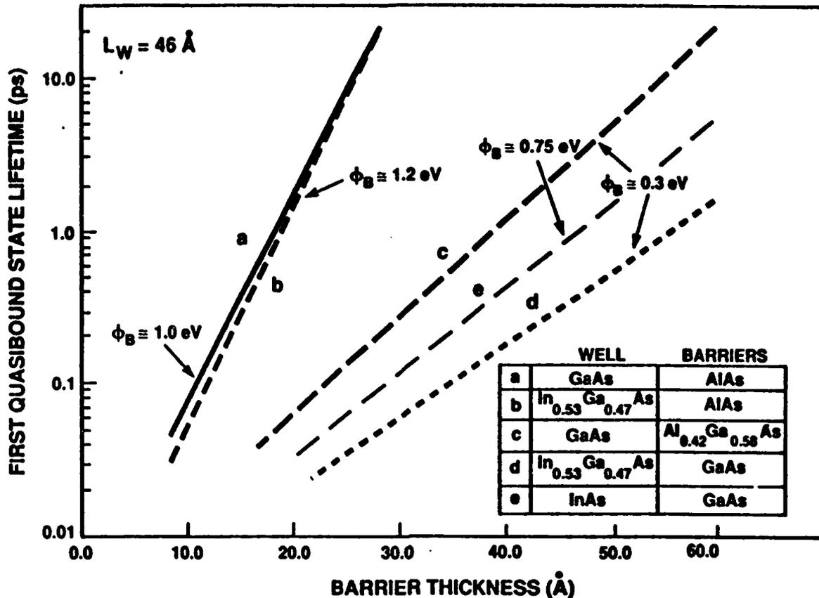
Fig. 5. Lifetime of the first quasibound state as a function of barrier thickness for double-barrier structures made from five different InGaAs/AlGaAs material systems. The quantum-well width is fixed at 4.6 nm.
