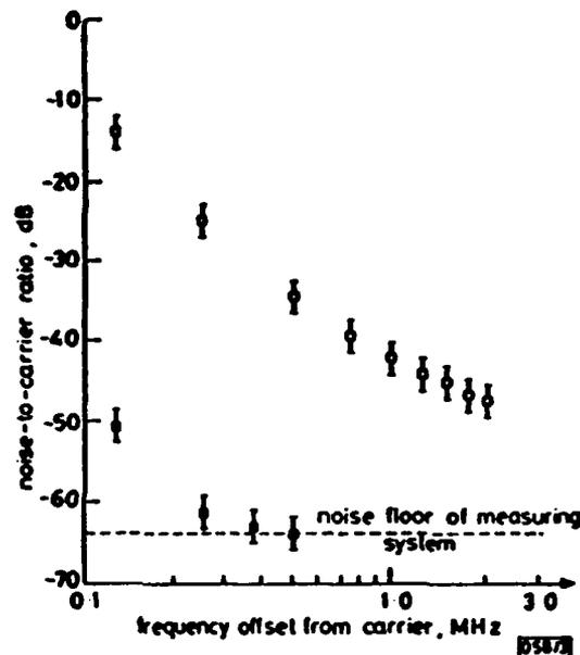
Fig. 3 Noise-to-carrier ratio  $S(f)$  for RTD oscillator
