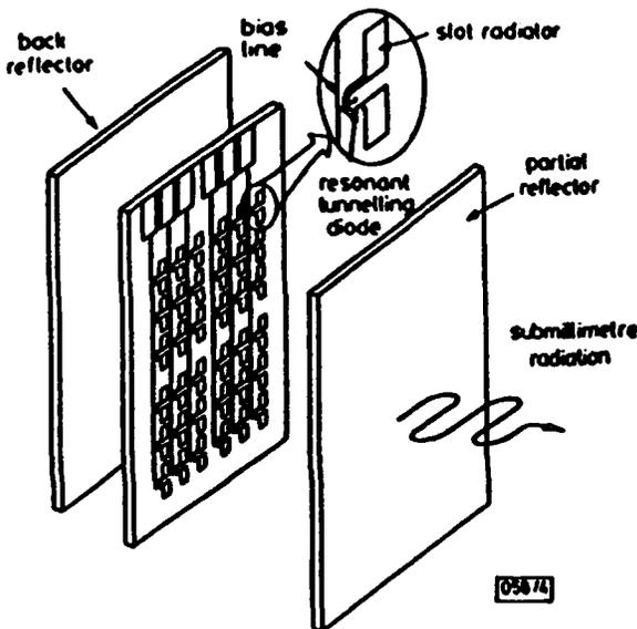
Fig. 4 Planar-monolithic array of RTD oscillators synchronized by quasi-optical cavity
