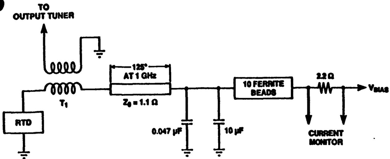
Fig. 1. Oscillator circuit using 25 parallel-connected RTDs
