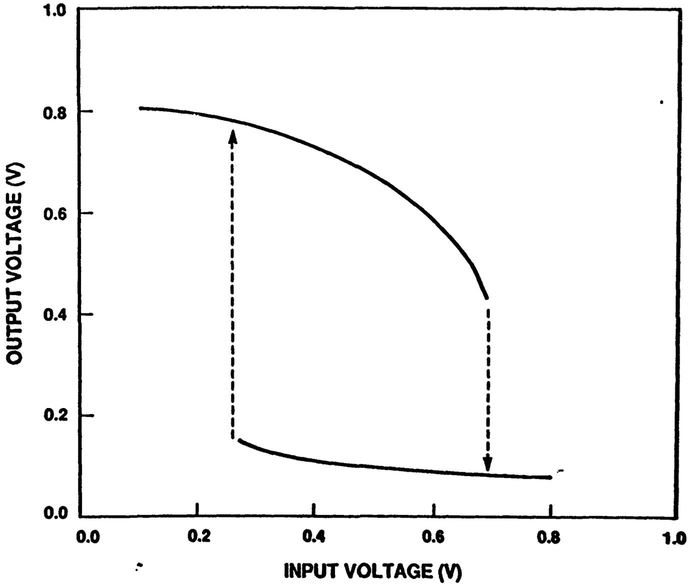
Fig. 3: Transfer characteristic of HFET-RTD inverter of Fig. 2.
