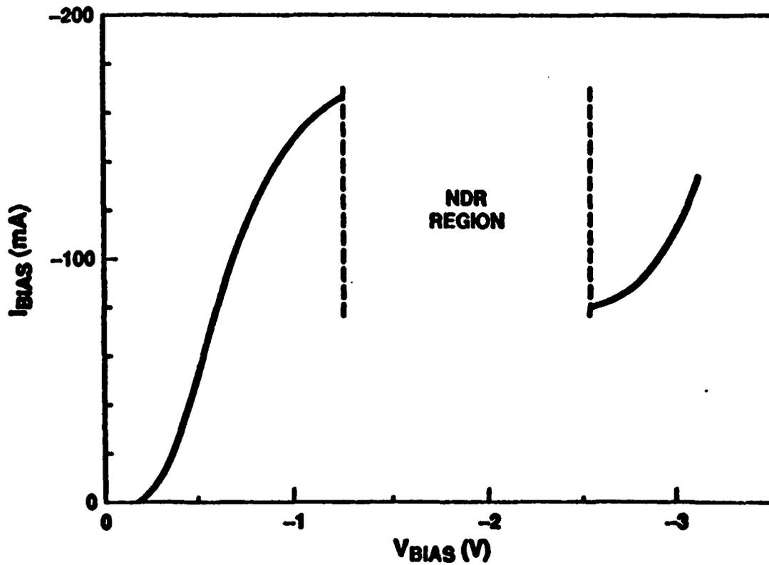
Fig. 2. I-V characteristic of 25 parallel-connected RTDs.
