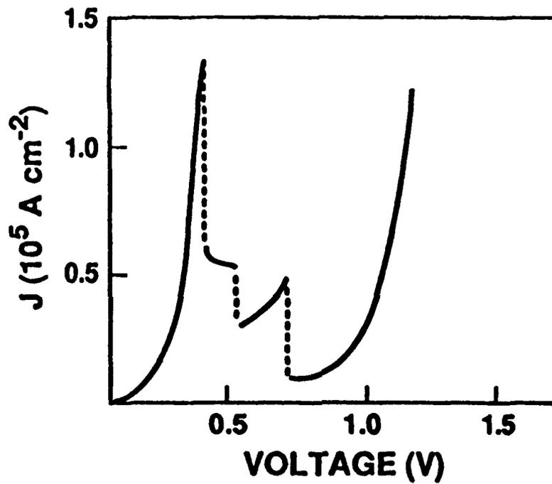
**Fig. 1:** Current density vs voltage for a low-power high-speed RTD made from the InGaAs/AlAs materials system.
