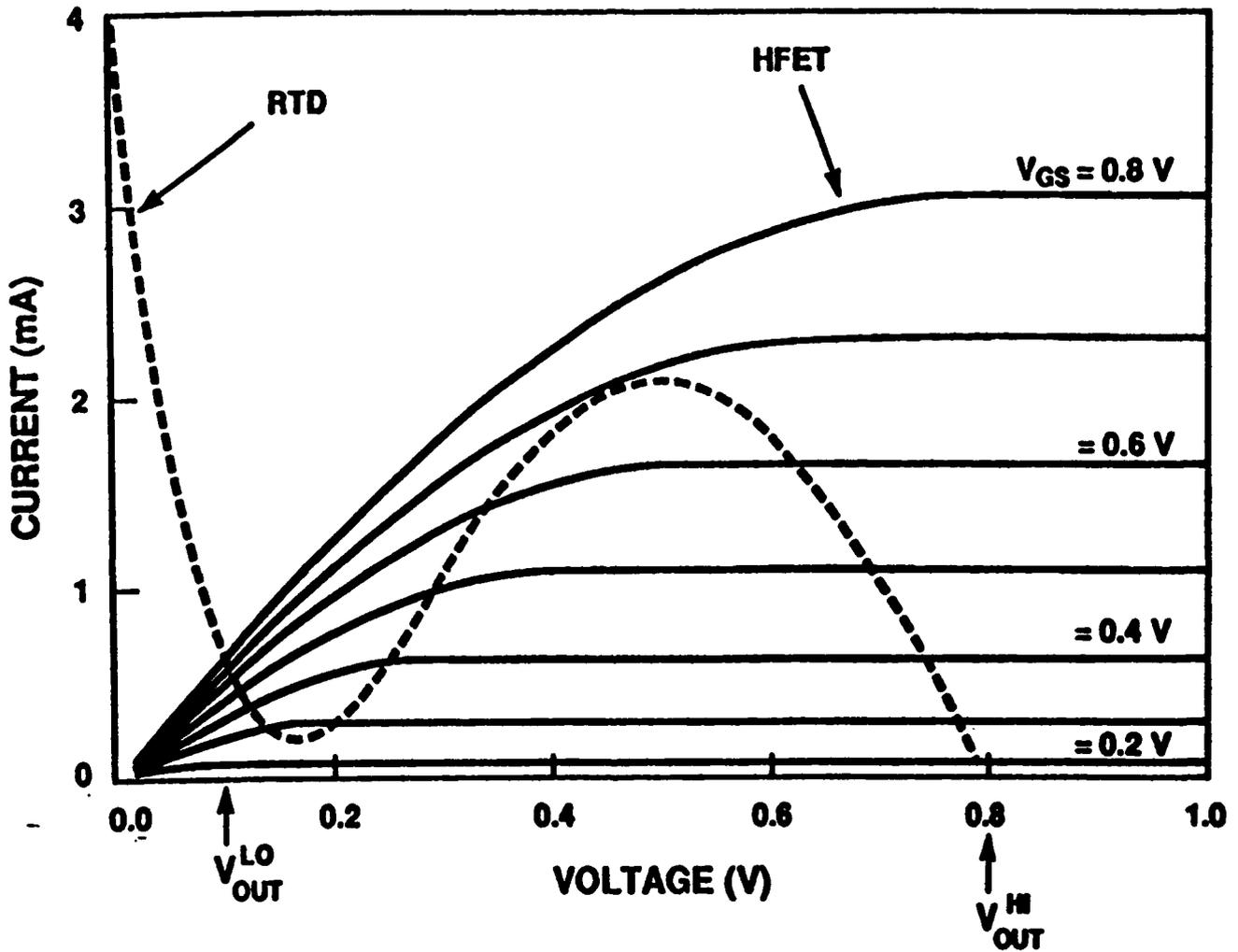
Fig. 2: Current-voltage curves for  $1.5\text{-}\mu\text{m}^2$ -area InGaAs/AlAs RTD and  $1.0\text{-}\mu\text{m}$ -gate-length InGaAs HFET at room temperature. Both curves are derived from SPICE 2G models.
