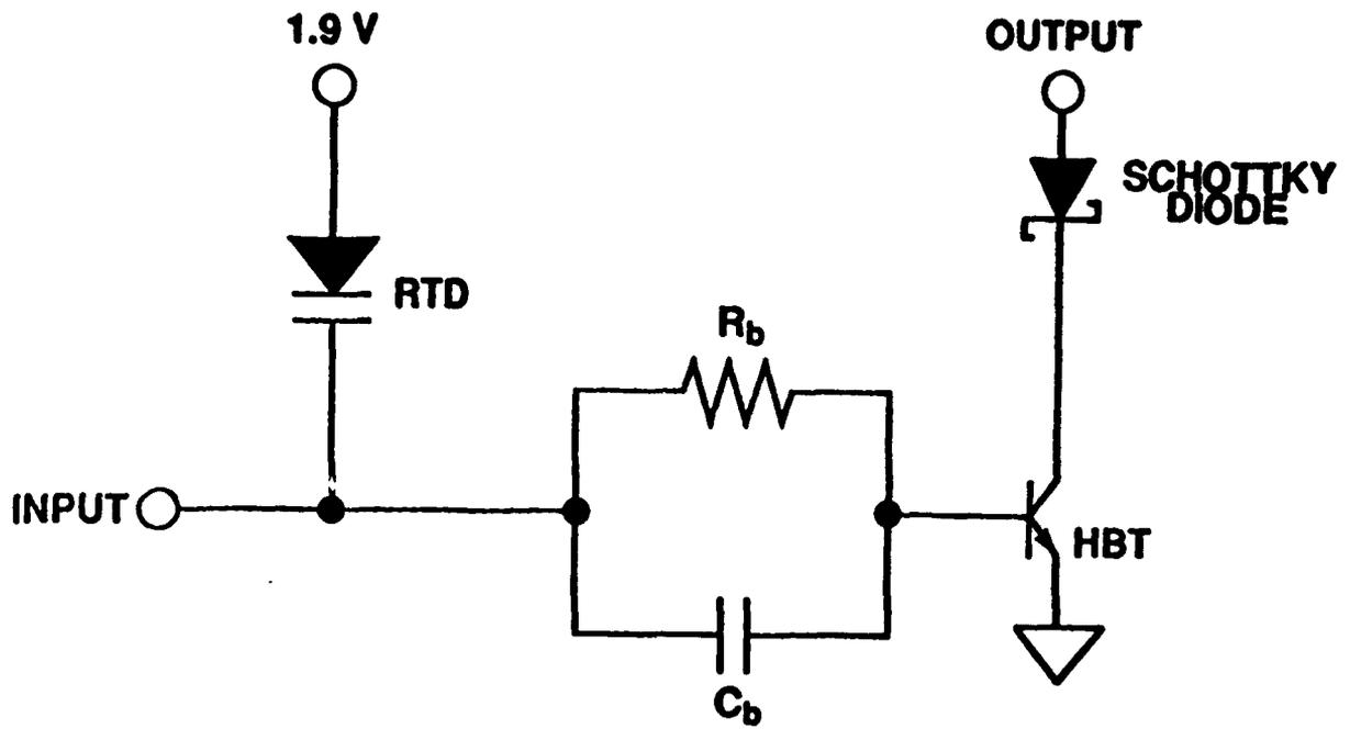
**Fig. 4:** Circuit diagram for inverter element containing an RTD and an npn HBT.
