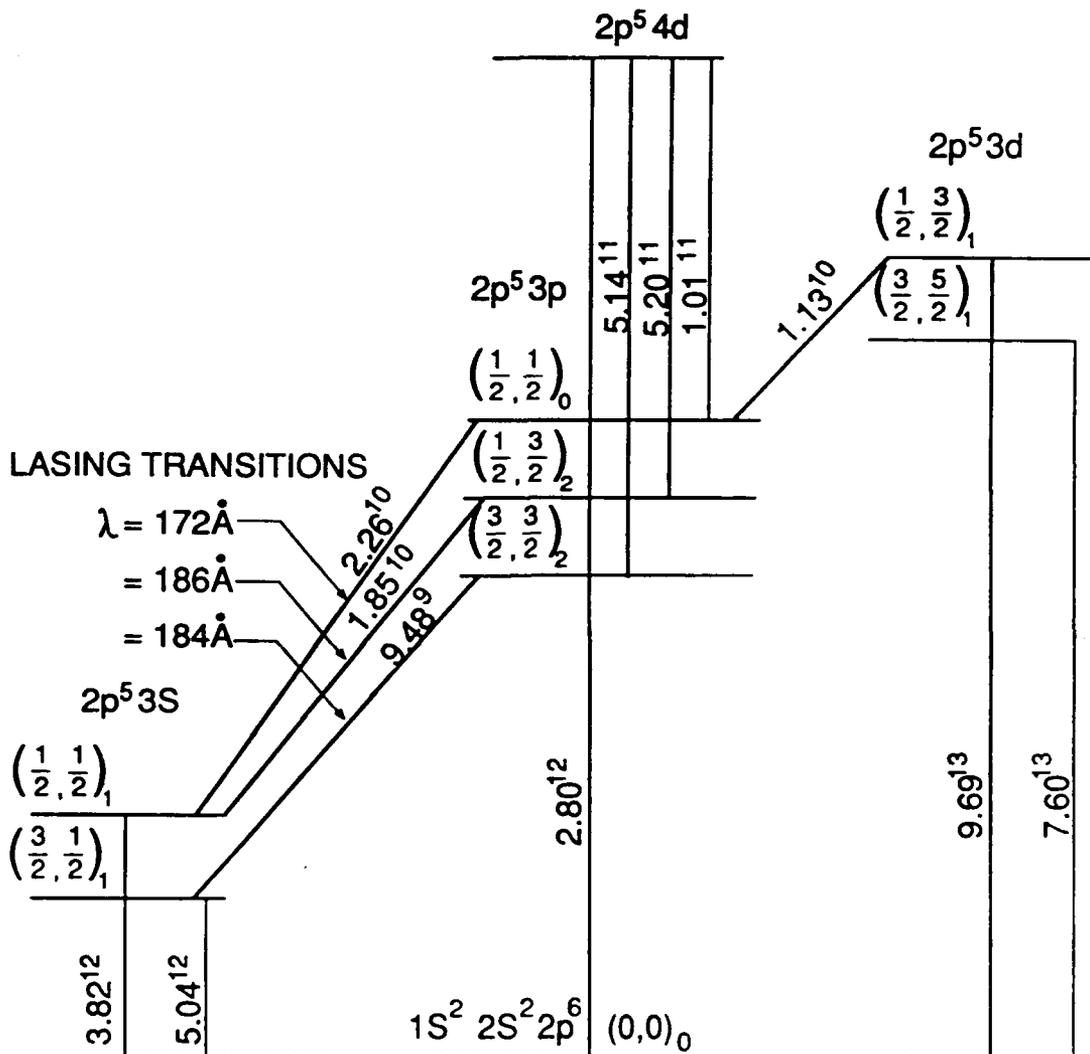
Fig. 1 Energy level diagram [ $(j_1, j_2)_J$  notation] and oscillator strengths for important lasing and resonance transitions for neonlike krypton. The 4d level is representative of a number of fine split levels that are lumped according to statistical equilibrium.
