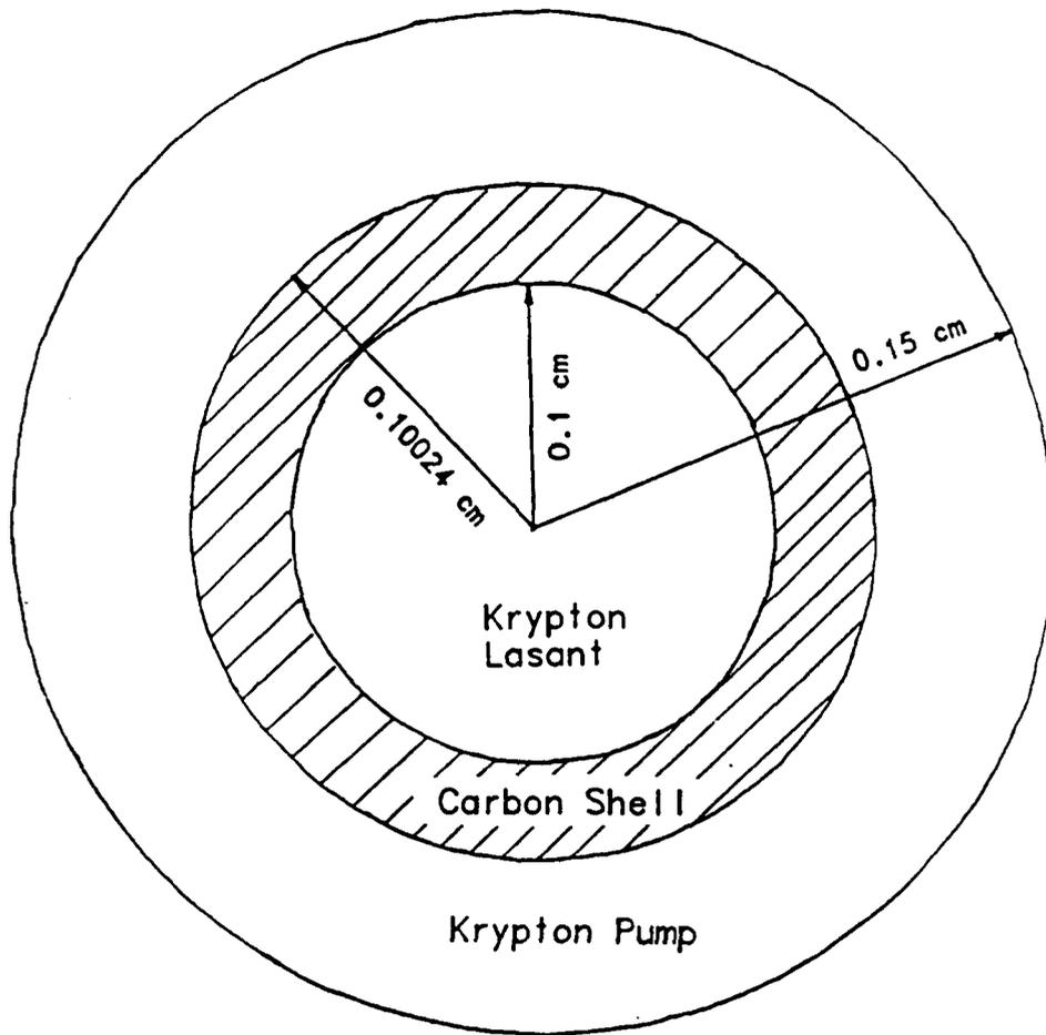
Fig. 2 Schematic diagram of z-pinch coaxial laser.
