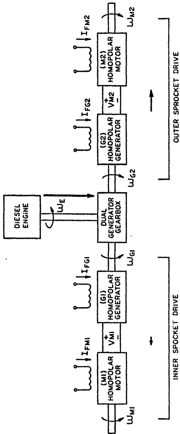
Figure 5-38. DI Homopolar Power Flow, Non-Regenerative Turns
