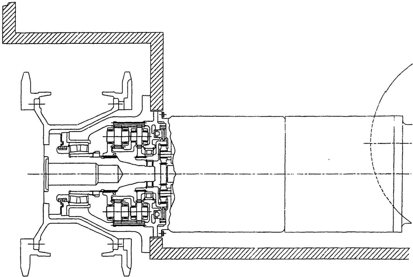
Figure 5-31. Triple Planetary Final Drive (19.5 Ton) (Homopolar)
