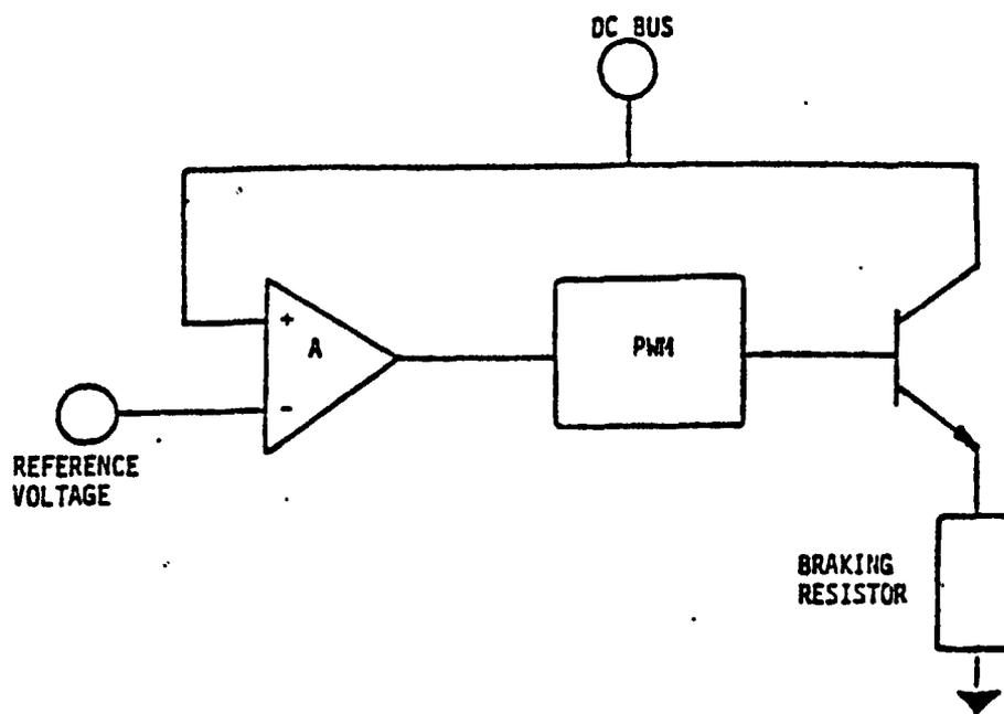
Figure 5-52. Braking Circuit Diagram
