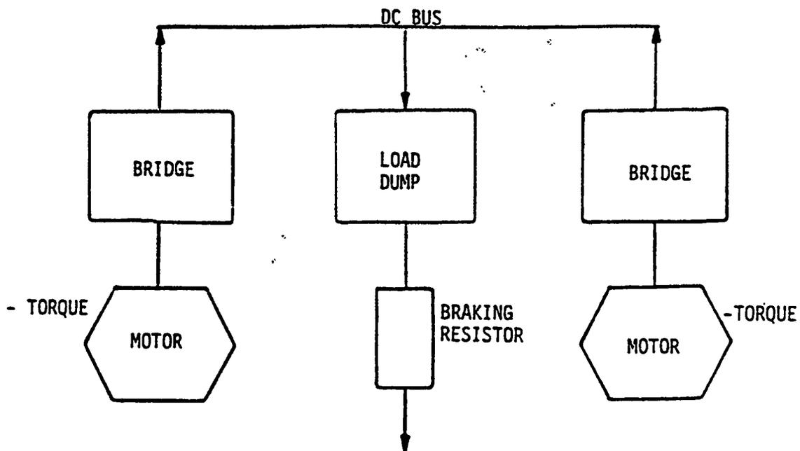
Figure 5-49. Power Flow Diagrams; Negative Torque at Motors
