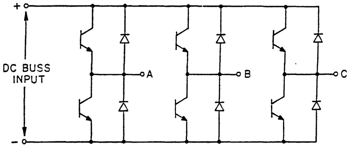
Figure 5-16. Three Phase Bidirectional Inverter.
