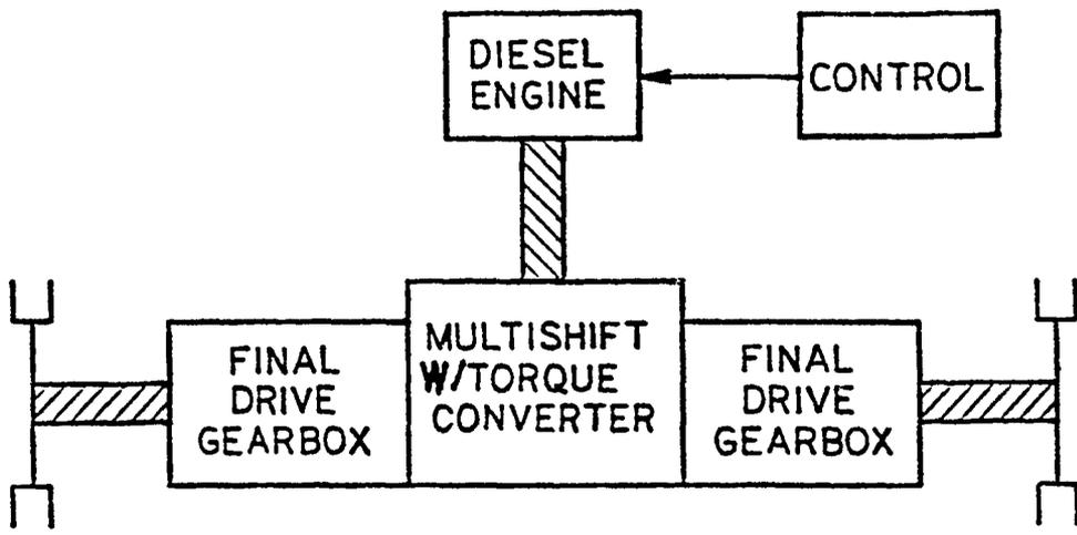
Figure 5-1. Conventional Combat Vehicle Drive.
