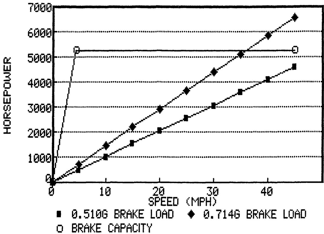
Figure 5-83. Panic Brake Load Versus Capacity (40 Ton Vehicle)
