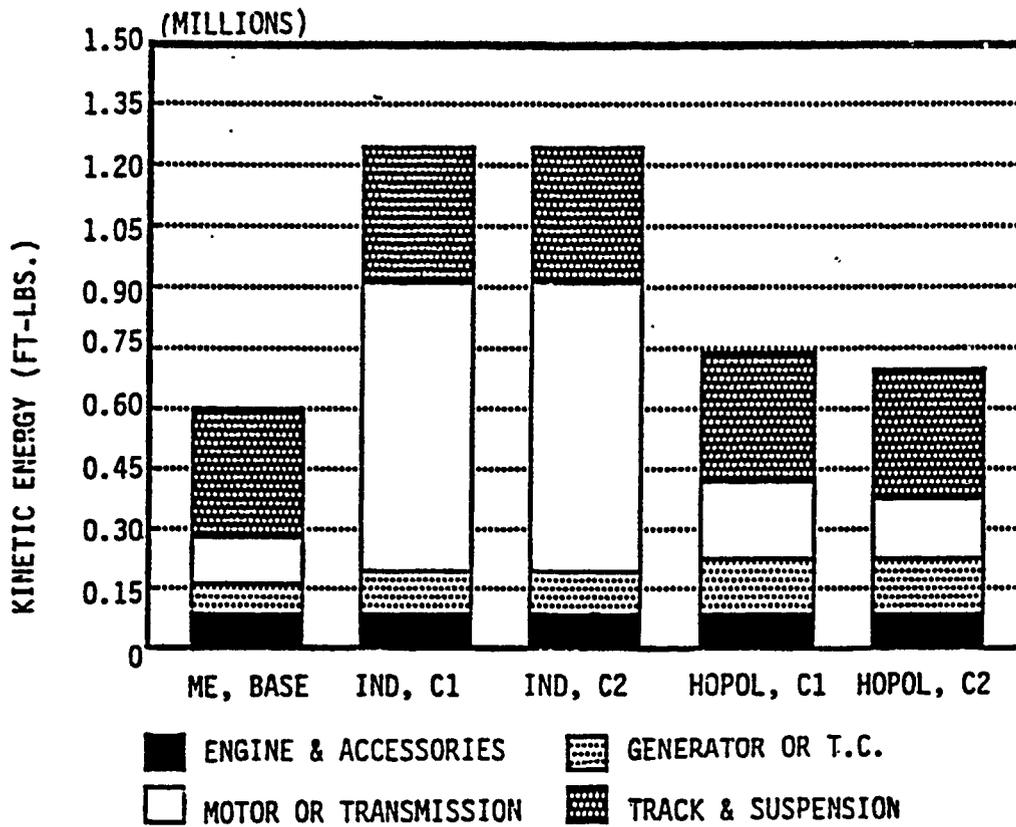
Figure 5-74. Kinetic Energy in Rotation (45 mph)
