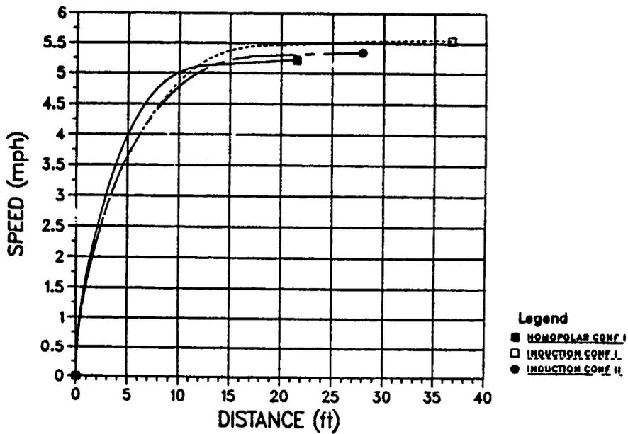
Figure 5-78. Acceleration and Speed on 60 Percent Grade
