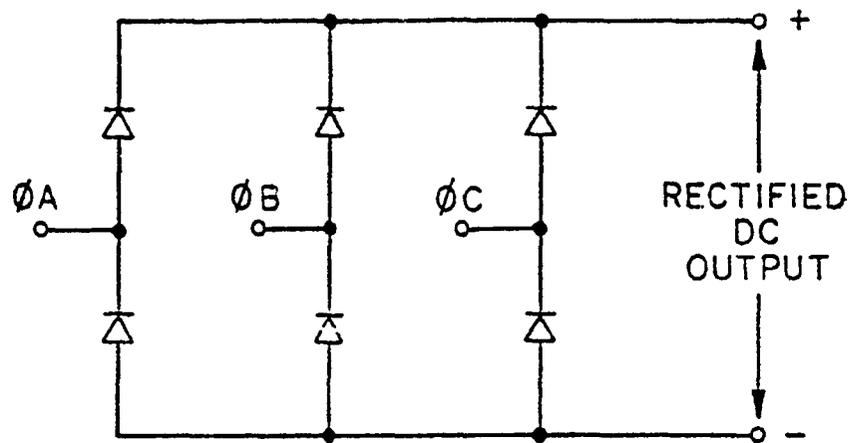
Figure 5-13. Three Phase Full-Wave Rectifier Bridge.
