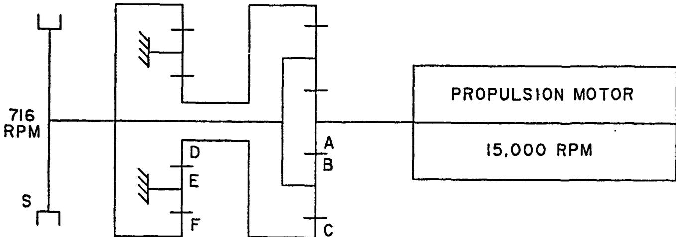
Figure 5-29. Final Drive Epicyclic System (Configuration I)
