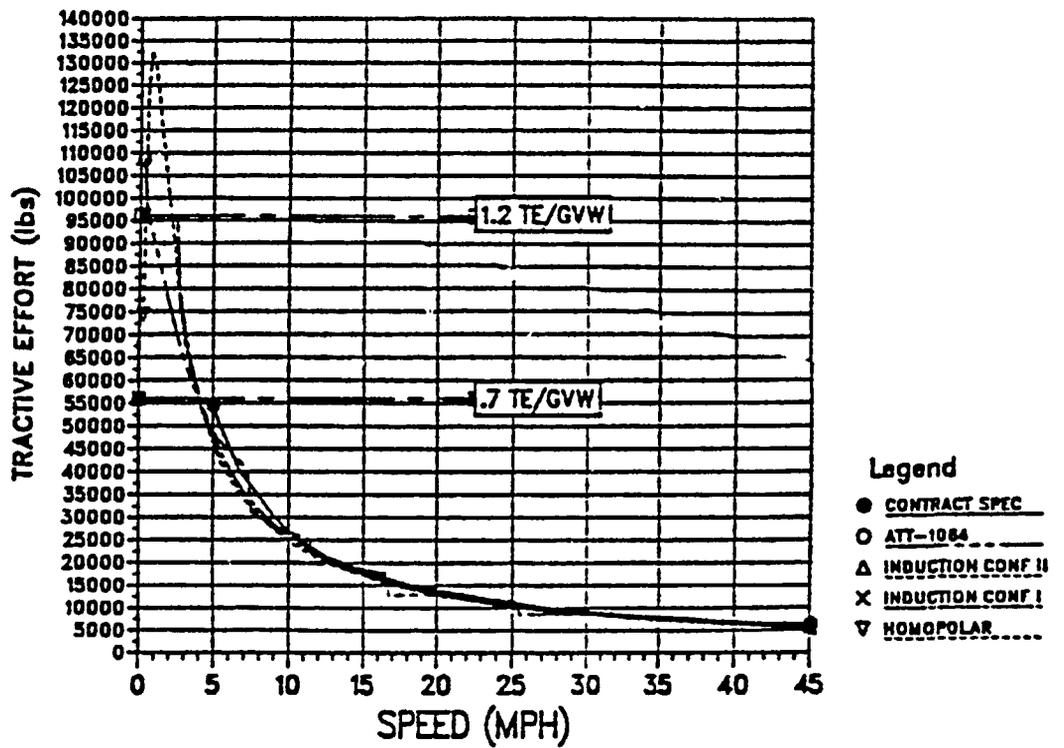
Figure 5-69. Tractive Effort Versus Speed (40 Ton Vehicle)
