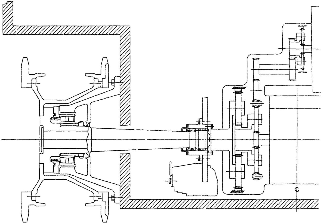
Figure 5-34. Drive and Sprocket Carrier Integration (19.5 Ton)
