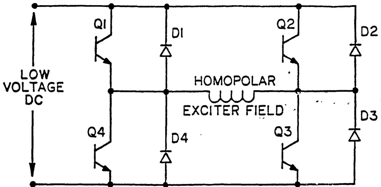
Figure 5-7. Typical Exciter Field Control
