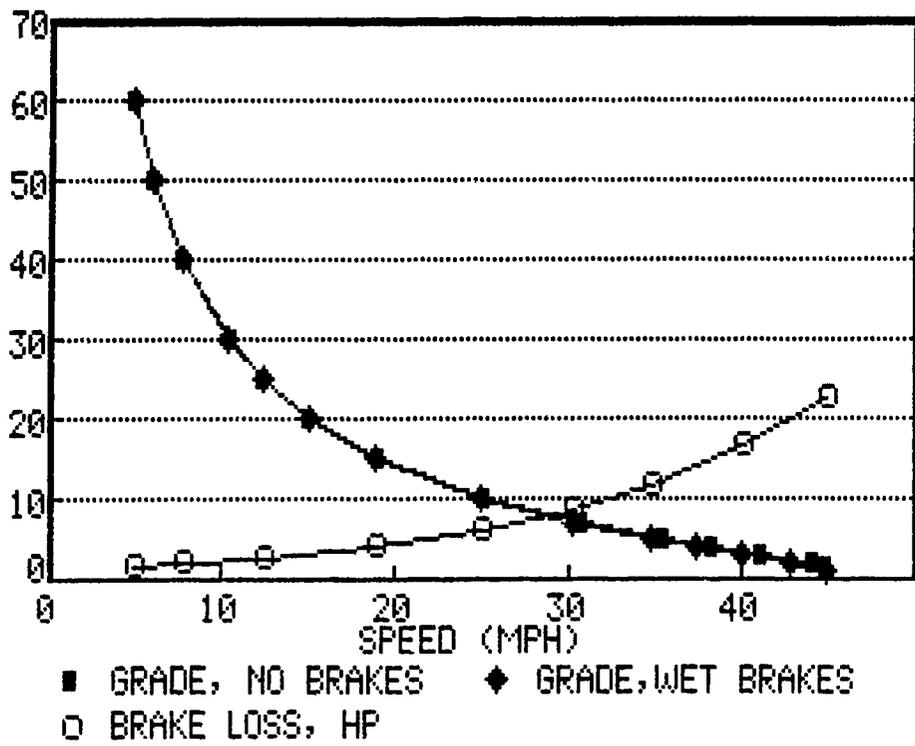
Figure 5-81. Wet Disk Brake Losses
