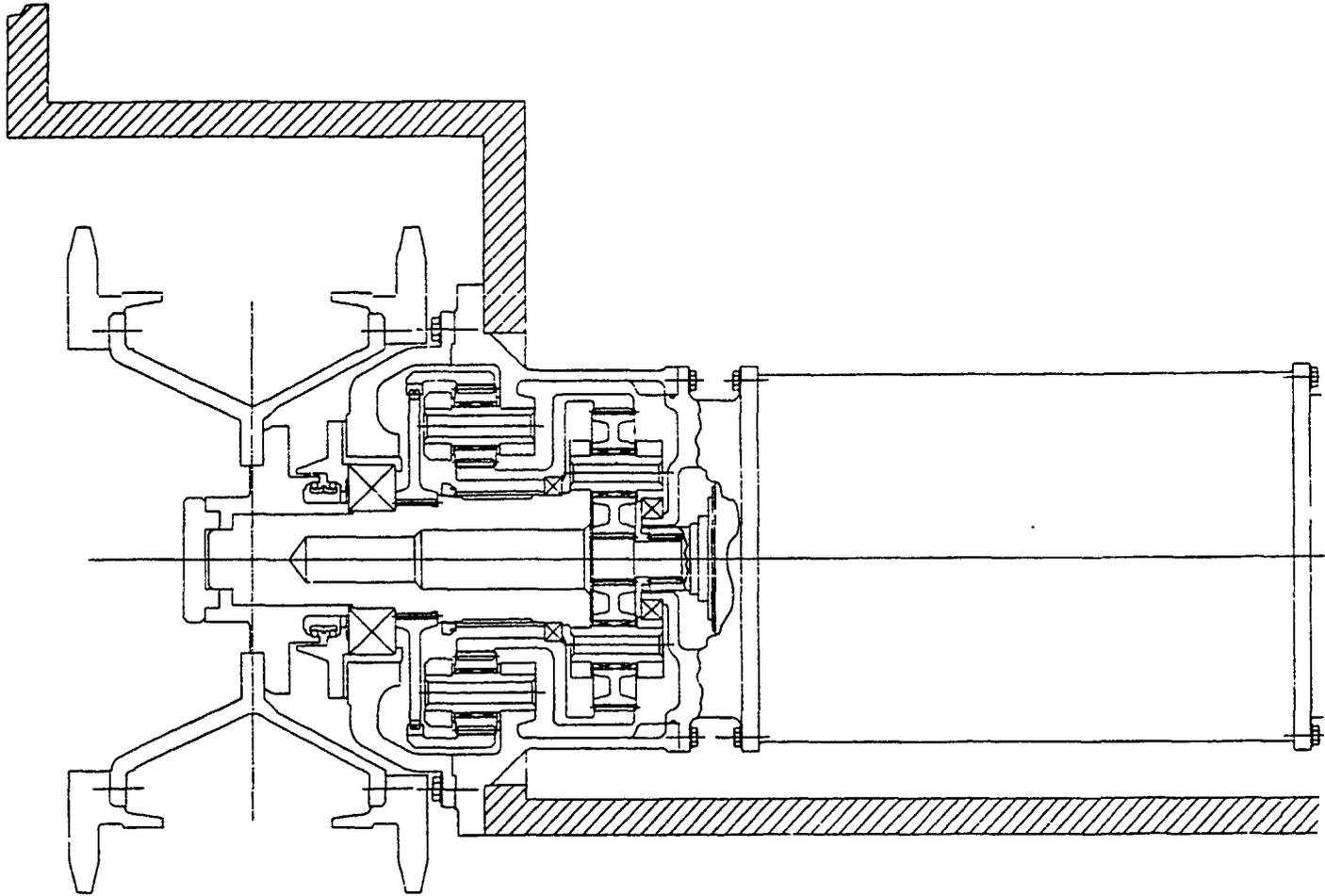
Figure 5-30. Sprocket Mounted Motor (19.4 Ton) (Configuration I)
