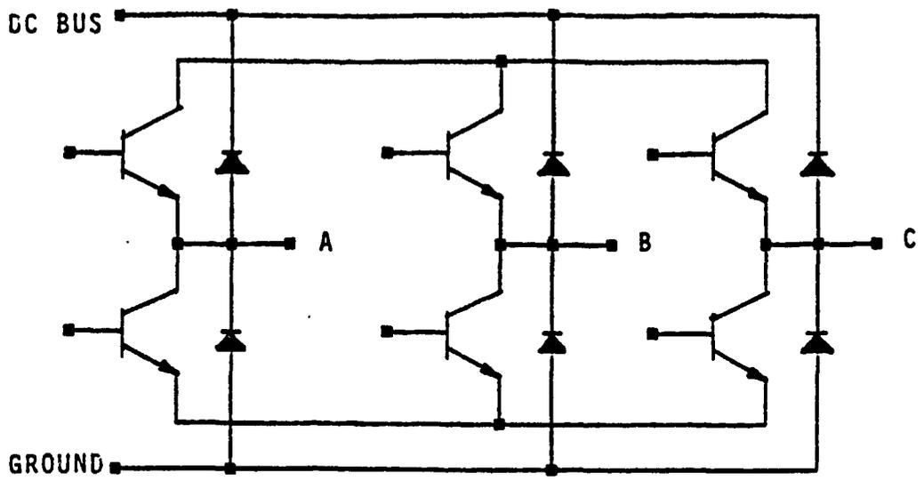
Figure 5-53. Bridge Circuit
