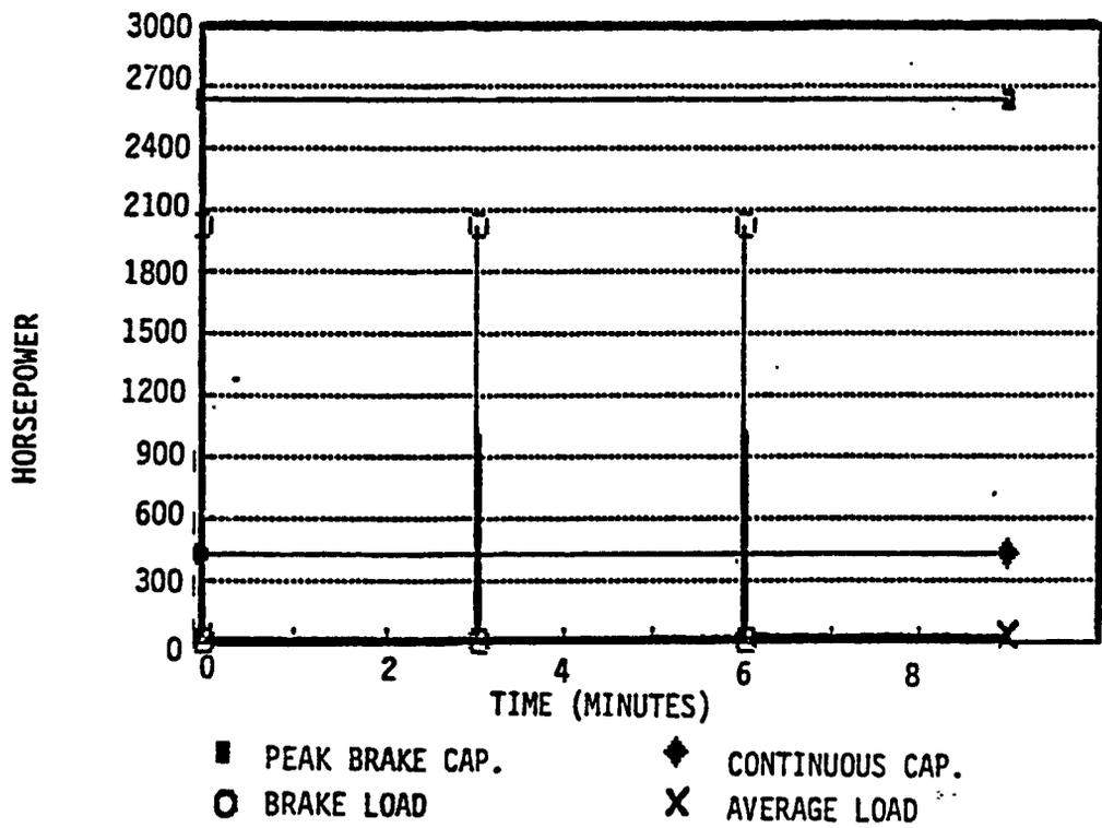
Figure 5-84. Horsepower Versus Time (25 Cycle Braking)
