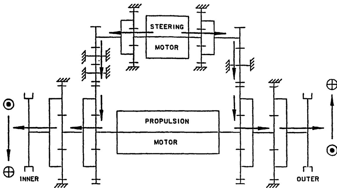
Figure 5-59. Power Flow - Steering Only (Configuration II)
