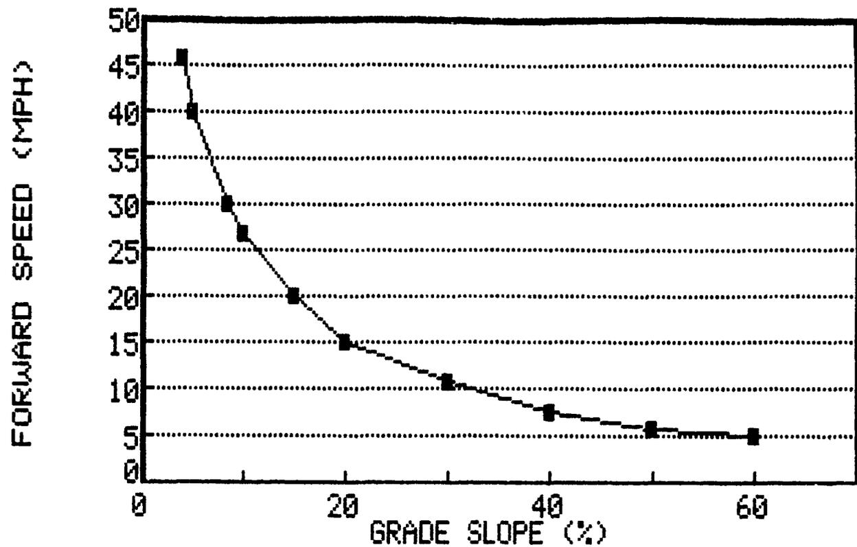
Figure 5-67. Sustained Speed Versus Grade
