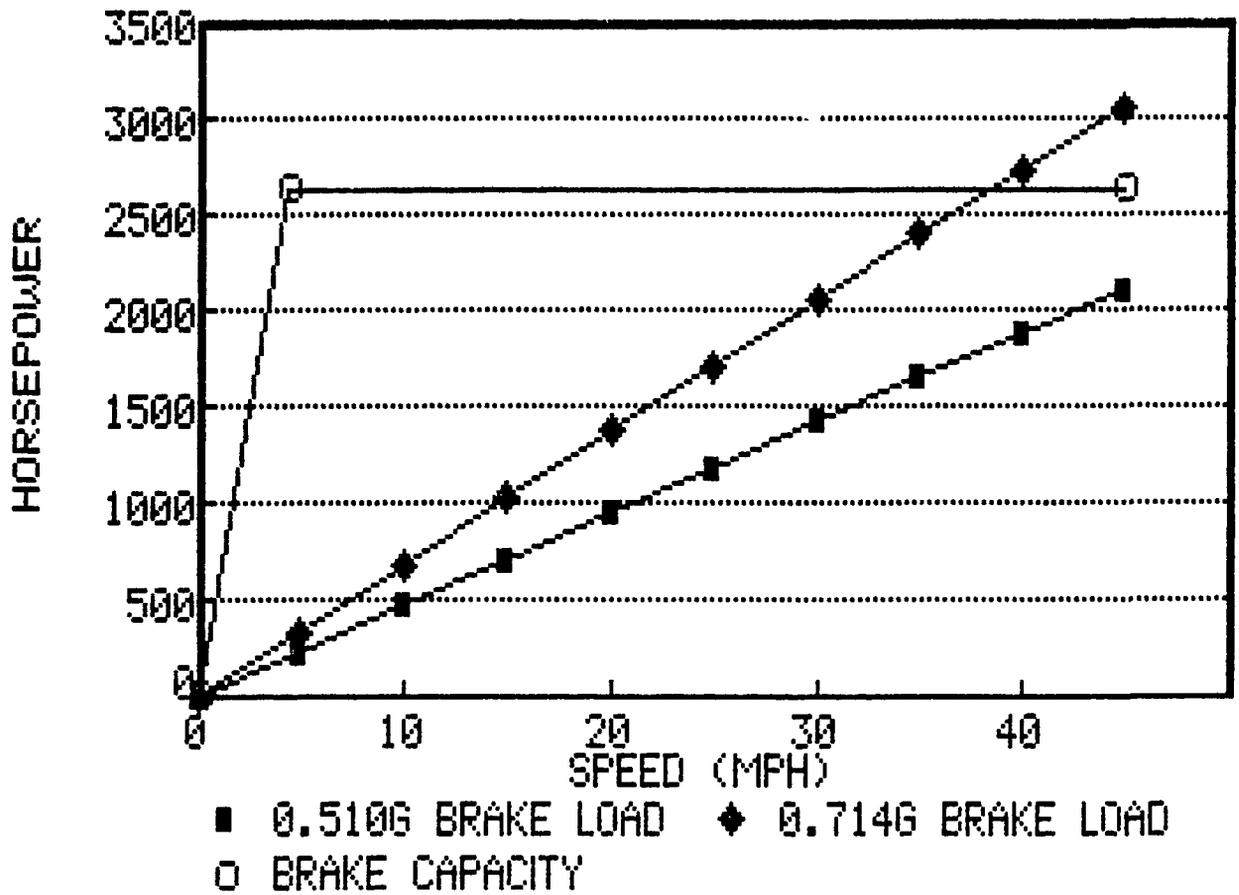
Figure 5-82. Panic Brake Load Versus Capacity (19.5 Ton Vehicle)
