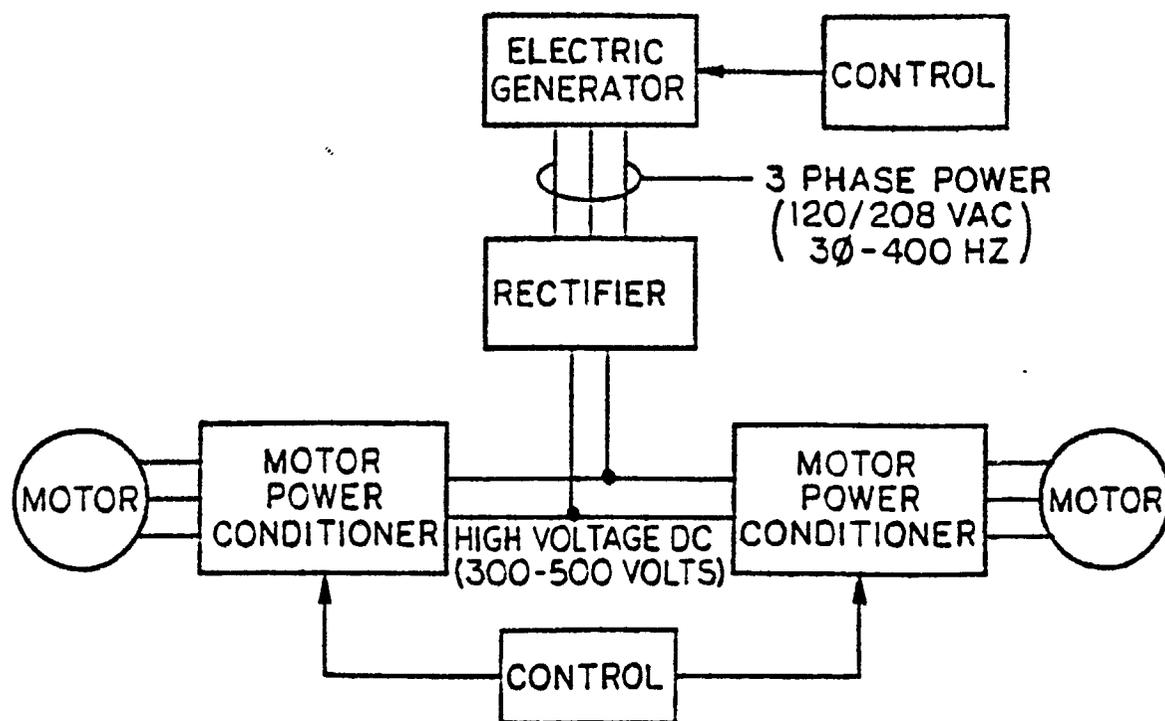
Figure 5-4. Typical AC Drive System
