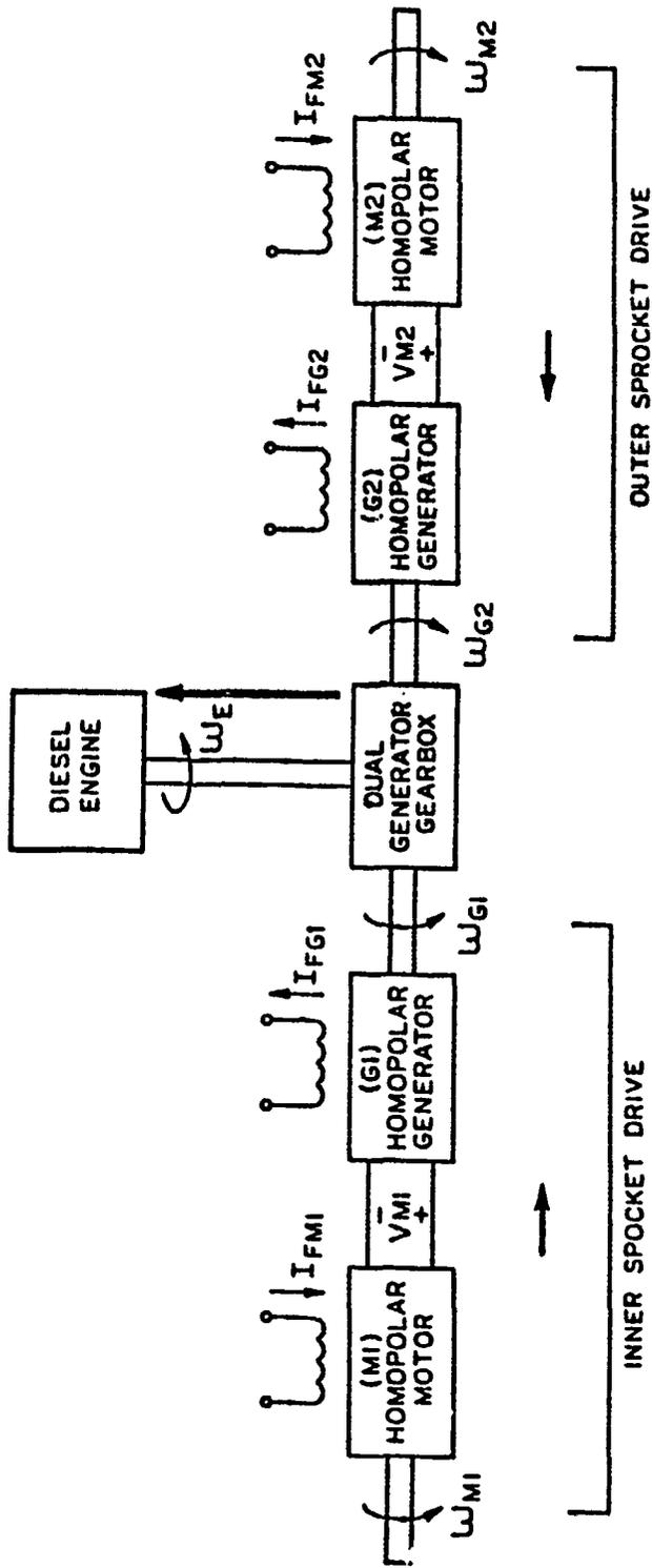
Figure 5-42. DI Homopolar Power Flow, Dynamic Braking
