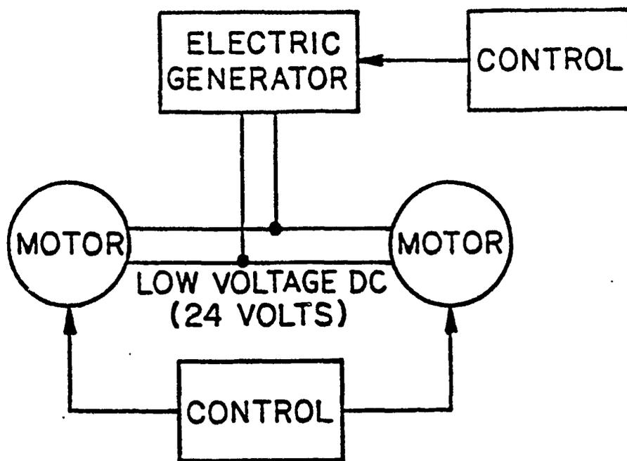
Figure 5-5. Typical DC Drive System
