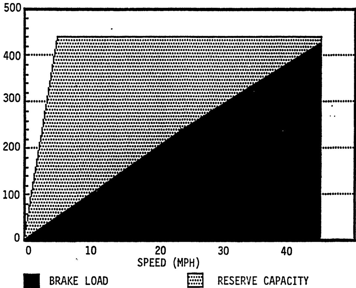
Figure 5-85. Brake Load & Capacity (15 percent Downgrade)
