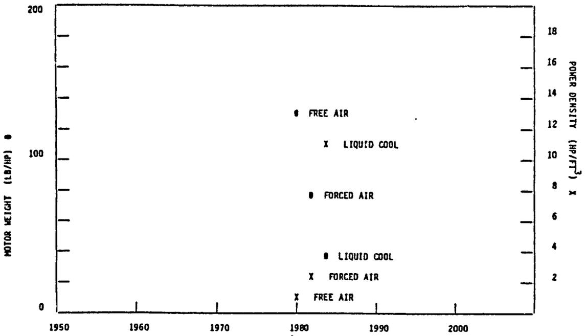
Figure 5-86. Motor Size Comparison Data
