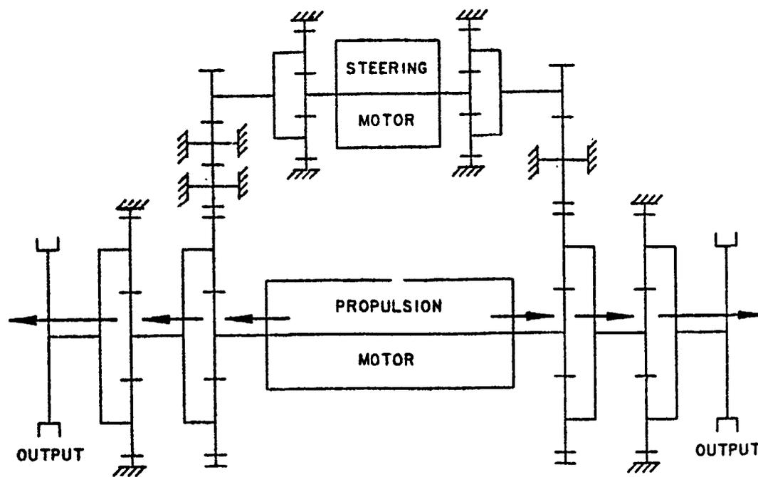
Figure 5-57. Power Flow for no Steering (Configuration II)
