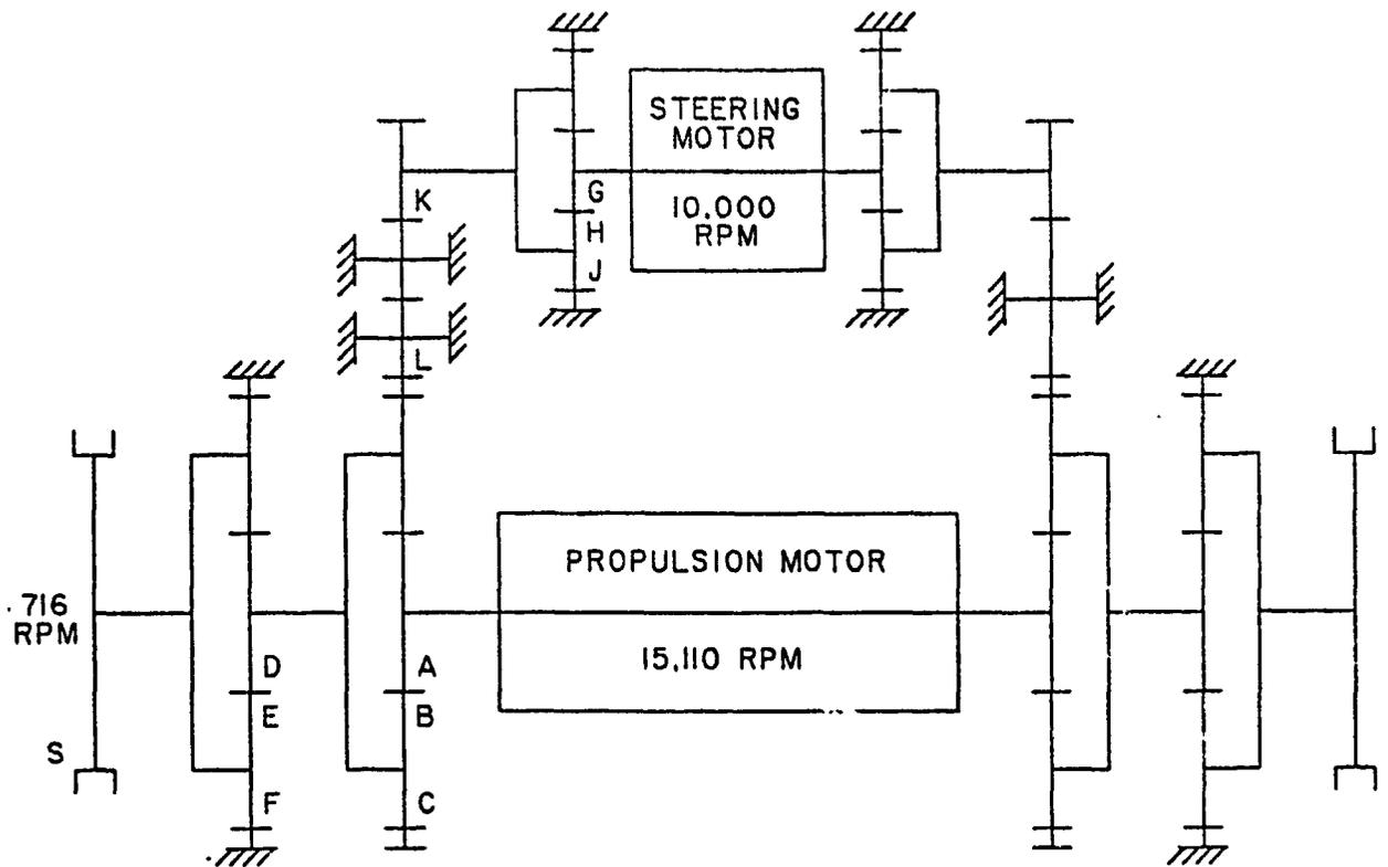
Figure 5-35. Propulsion and Steering Gear System (Configuration II)
