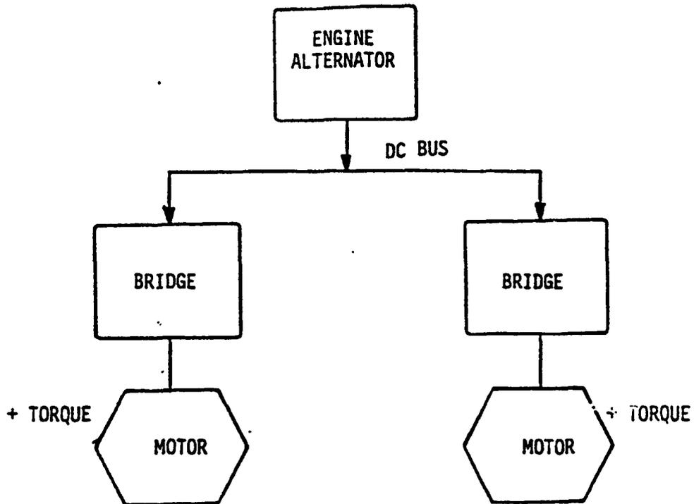
Figure 5-48. Power Flow Diagrams; Positive Torque at Motors
