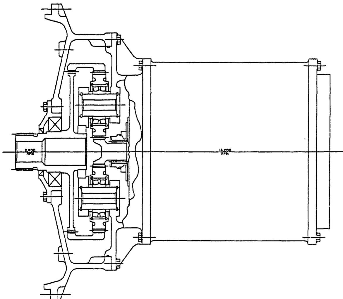
Figure 5-26. HF Induction AC Alternator Drive
