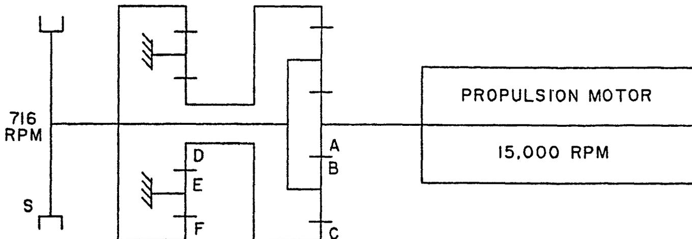
Figure 5-28. Final Drive with Split Power Flow (Configuration I)
