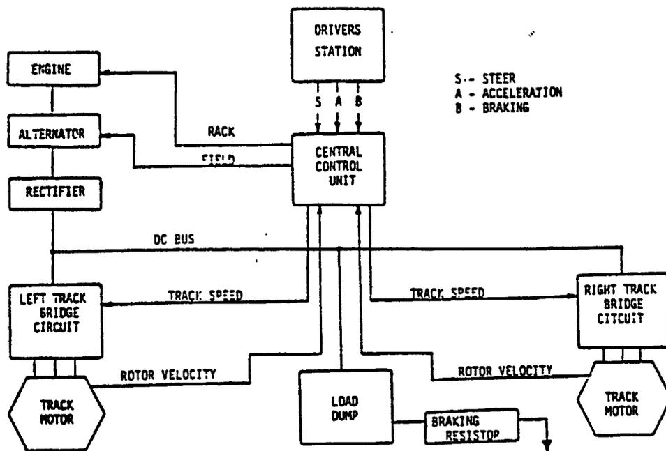
Figure 5-46. Control System Block Diagram
