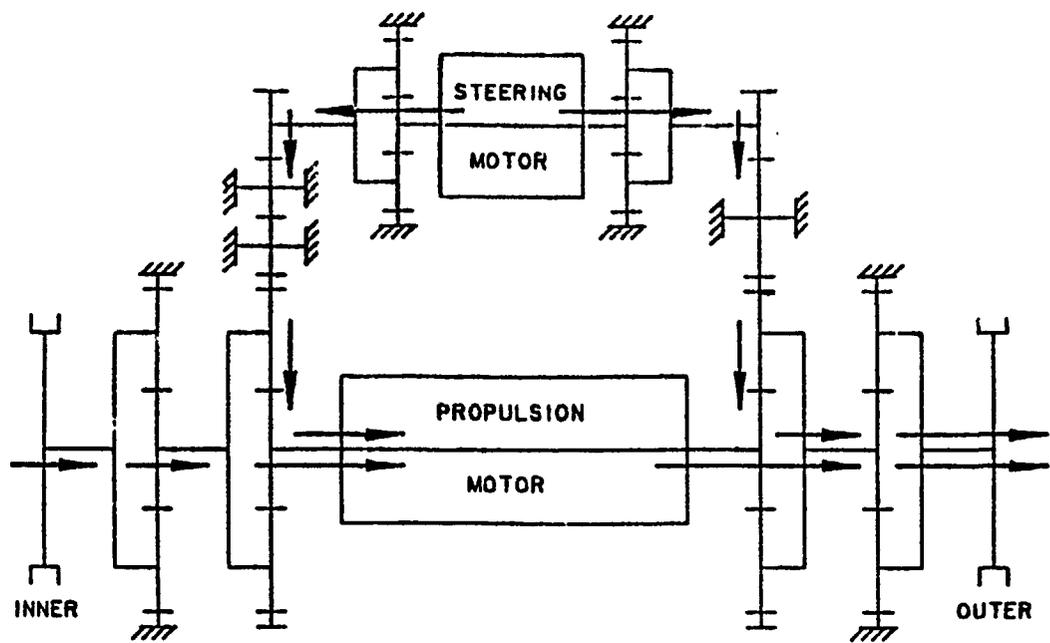
Figure 5-58. Power Flow for Propel and Steer (Configuration II)
