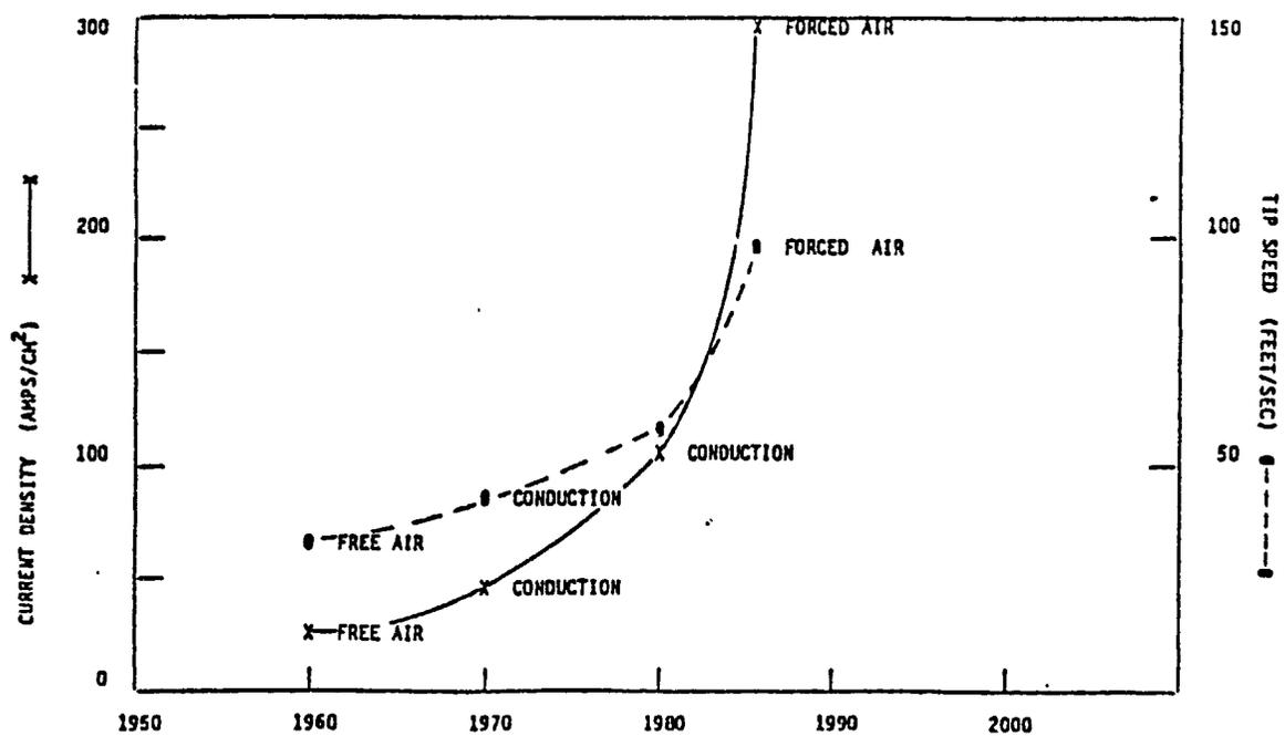
Figure 5-88. Brush Capacity Comparison Data (Graphite)
