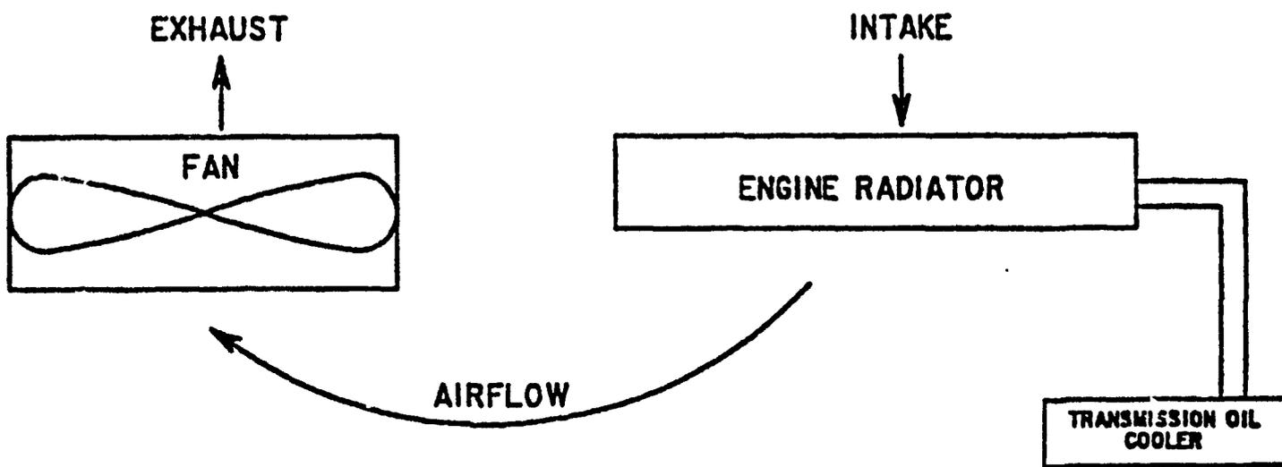
Figure 5-19. Mechanical Cooling System Arrangement.
