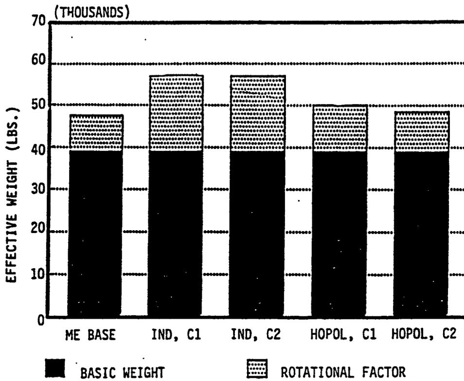
Figure 5-75. Impact of Rotational Inertia
