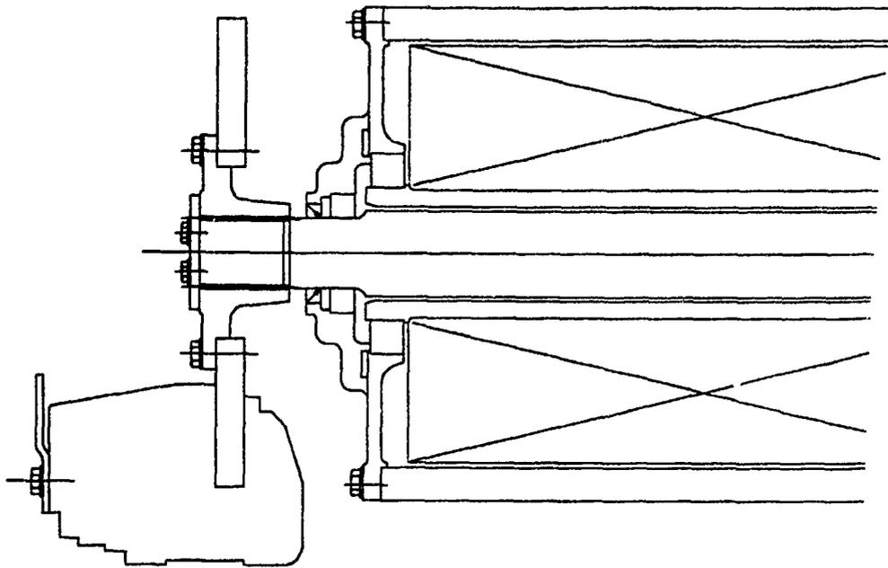
Figure 5-32. Integrated Motor/Final Drive
