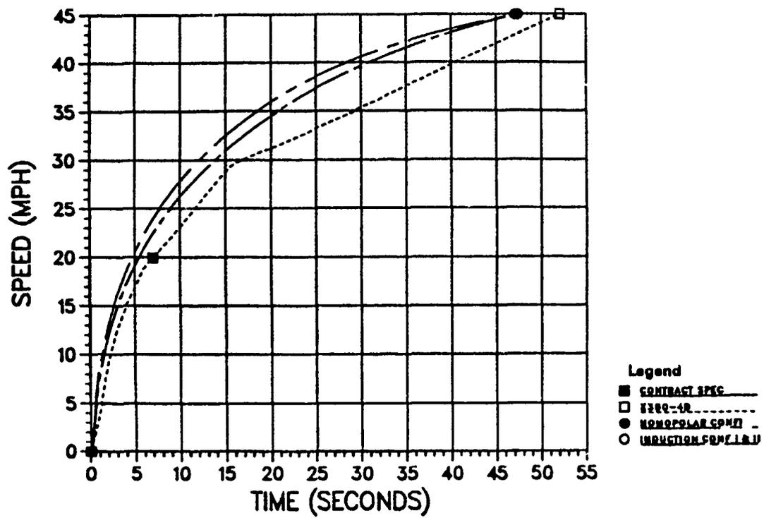
Figure 5-70. Acceleration Performance (19.5 Ton Vehicle)
