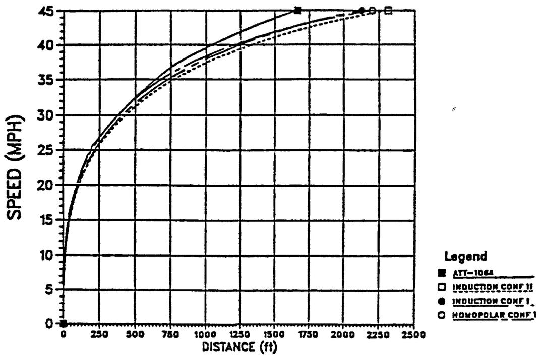
Figure 5-73. Speed Versus Distance (40 Ton Vehicle)
