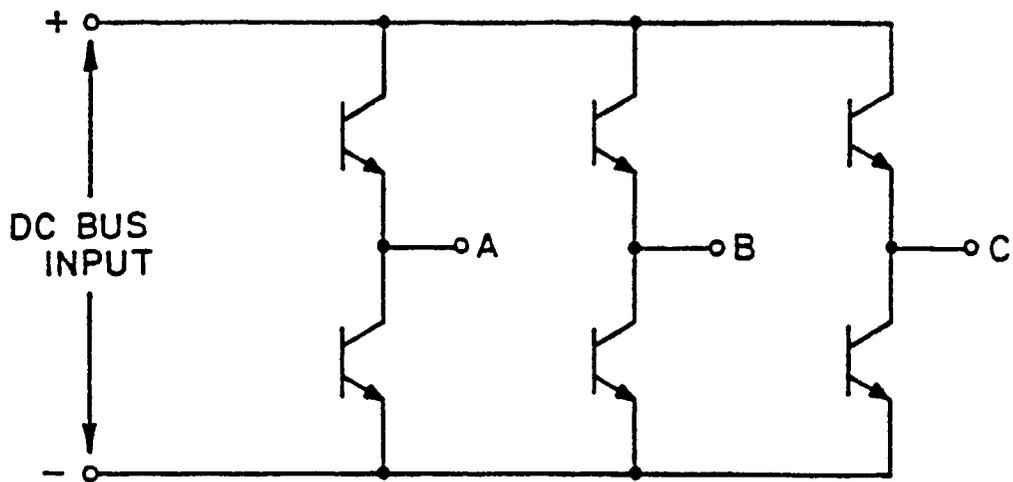
Figure 5-15. Three Phase Transistor Inverter.
