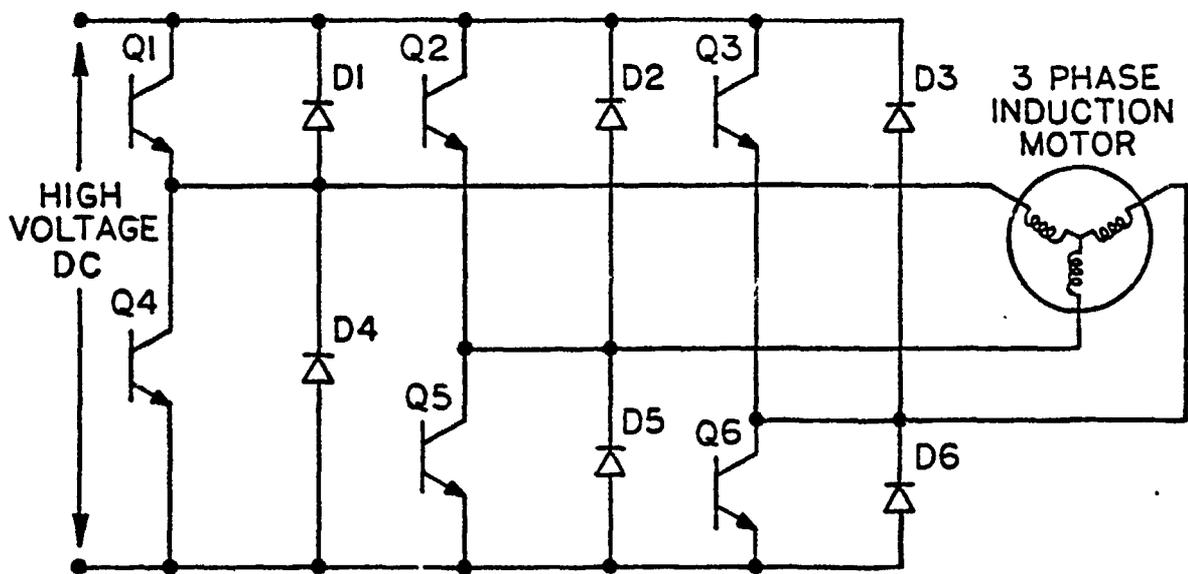
Figure 5-6. Typical Three-Phase DC/AC Inverter
