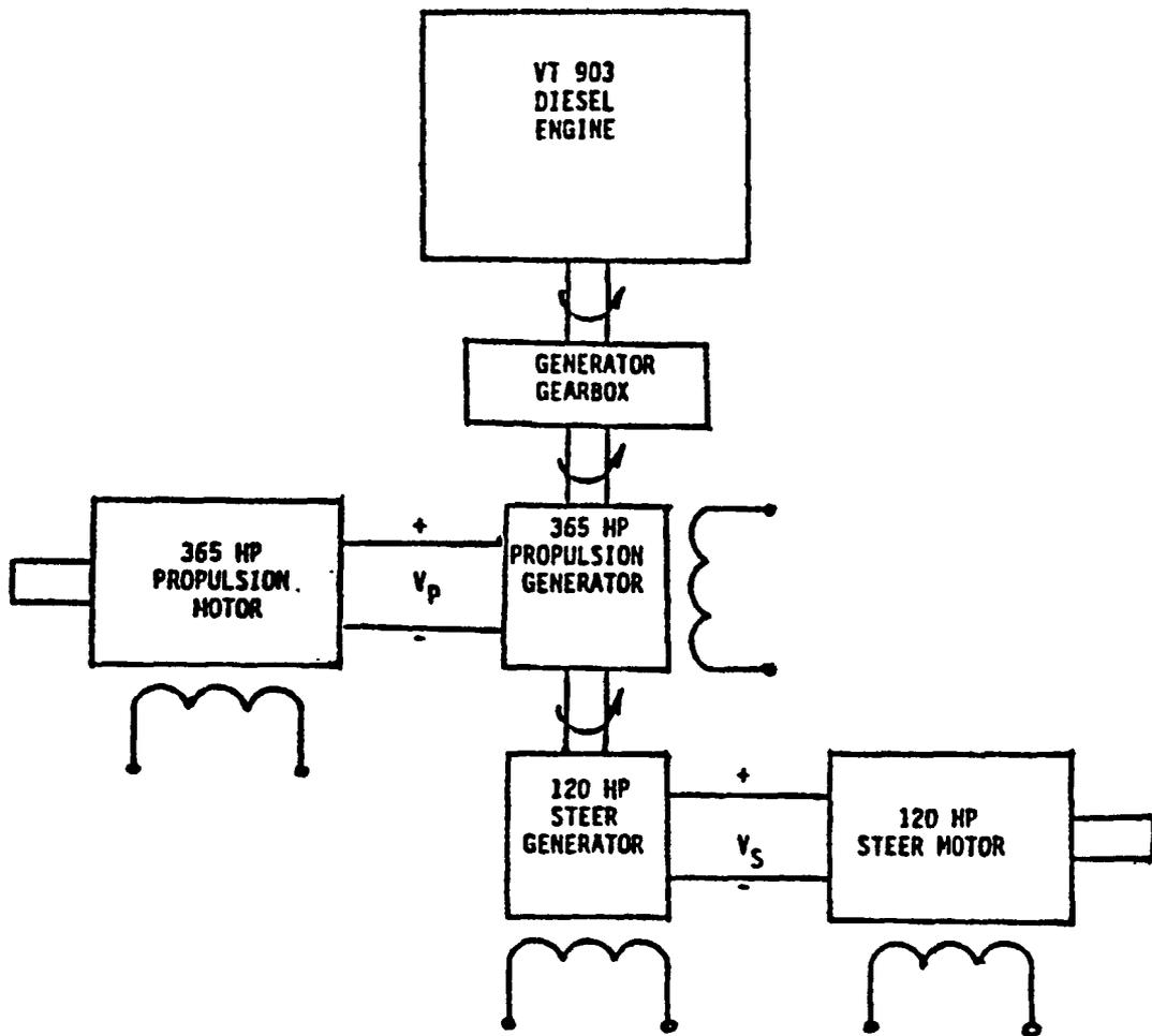
Figure 5-56. Configuration II; Homopolar Motor System
