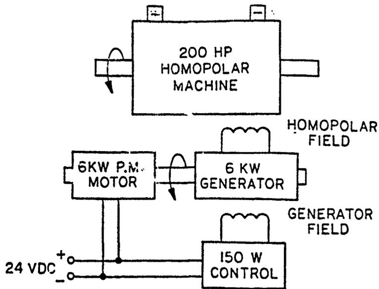
Figure 5-44. Potential Rotary Field Exciter Configuration
