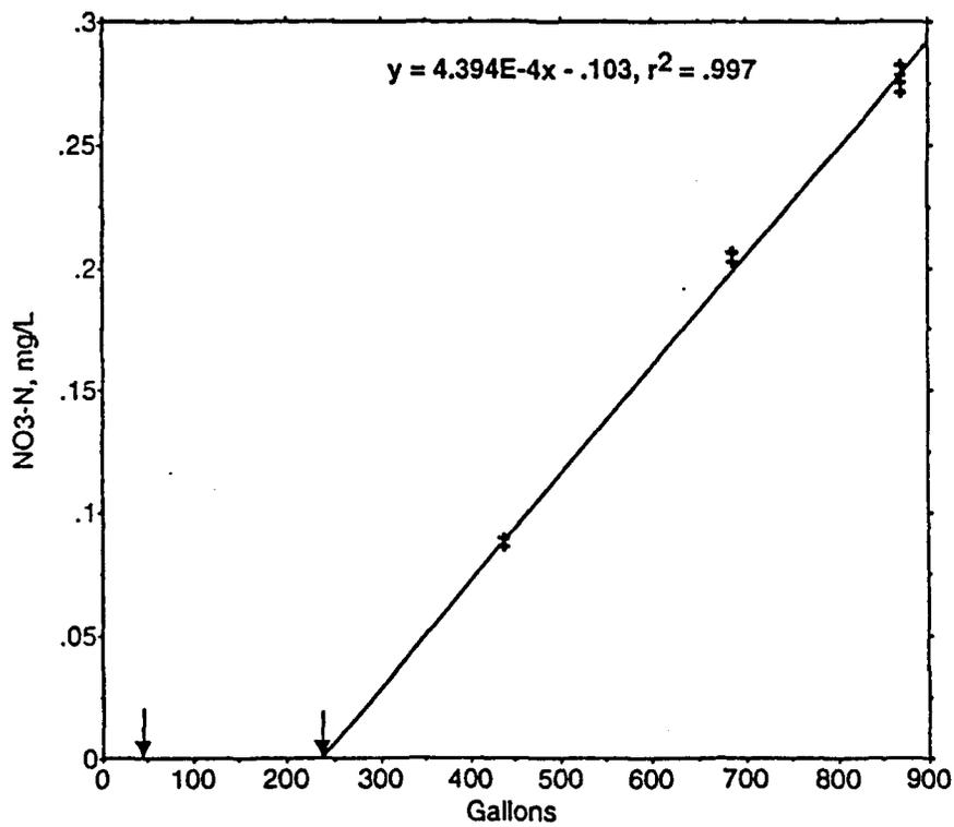
Figure 5: Best fit line to those samples containing detectable NO<sub>3</sub>-N. Lines for both NO<sub>3</sub>-N versus time (a) and versus gallons of water produced (b) have very high correlation coefficients, and predict that leakage from the alluvium was produced from the bedrock well beginning at about 38 or 39 minutes. The first two samples, at time 8 minutes and 38 minutes, showed undetectable NO<sub>3</sub>-N. These two samples are shown as arrows on 5b.
