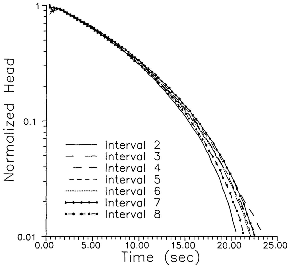
Figure III.B.1 - Normalized head ( $H/H_0$ ) versus time plots for slug tests in seven intervals of GEMS well 2-5 ( $H_0 = 3.05$  m). See Table III.B.1 for depths corresponding to each interval.
