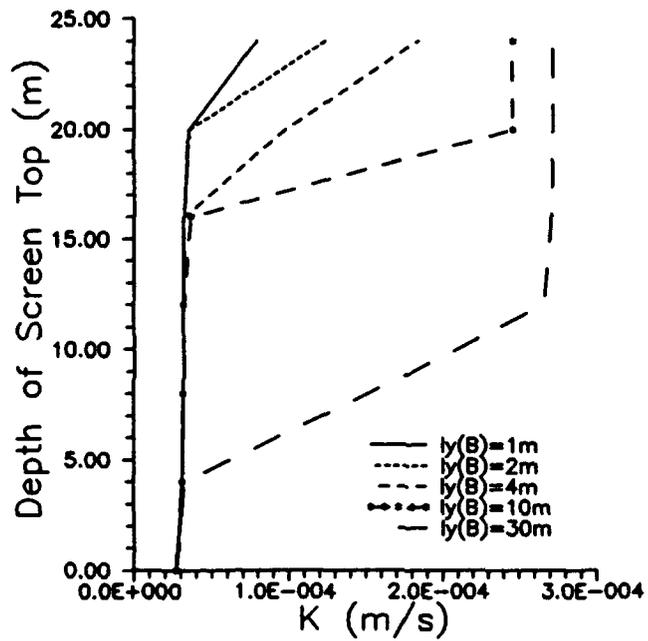
Figure II.B.10. Conductivity versus depth plot for Scenario 1A of Table II.B.1 ( $l_y(B)$  = thickness of layer B)
