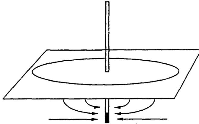
Figure A-1: Schematic diagram of the bedrock well, boundary between the alluvium and bedrock, radius of the cone of depression created during pumping, and possible ground-water flow paths.
