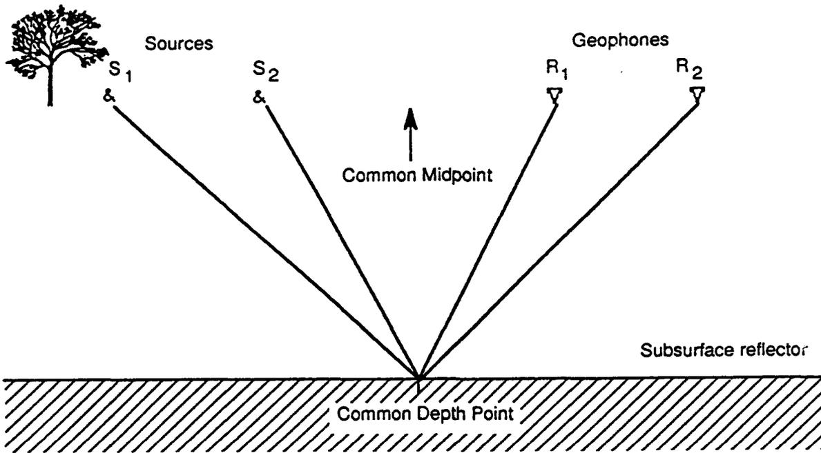
Figure A-4. The concept of Common Depth Point (CDP). Note that ray paths from two different shots ( $S_1$  and  $S_2$ ) reflect from a common point in the subsurface.
