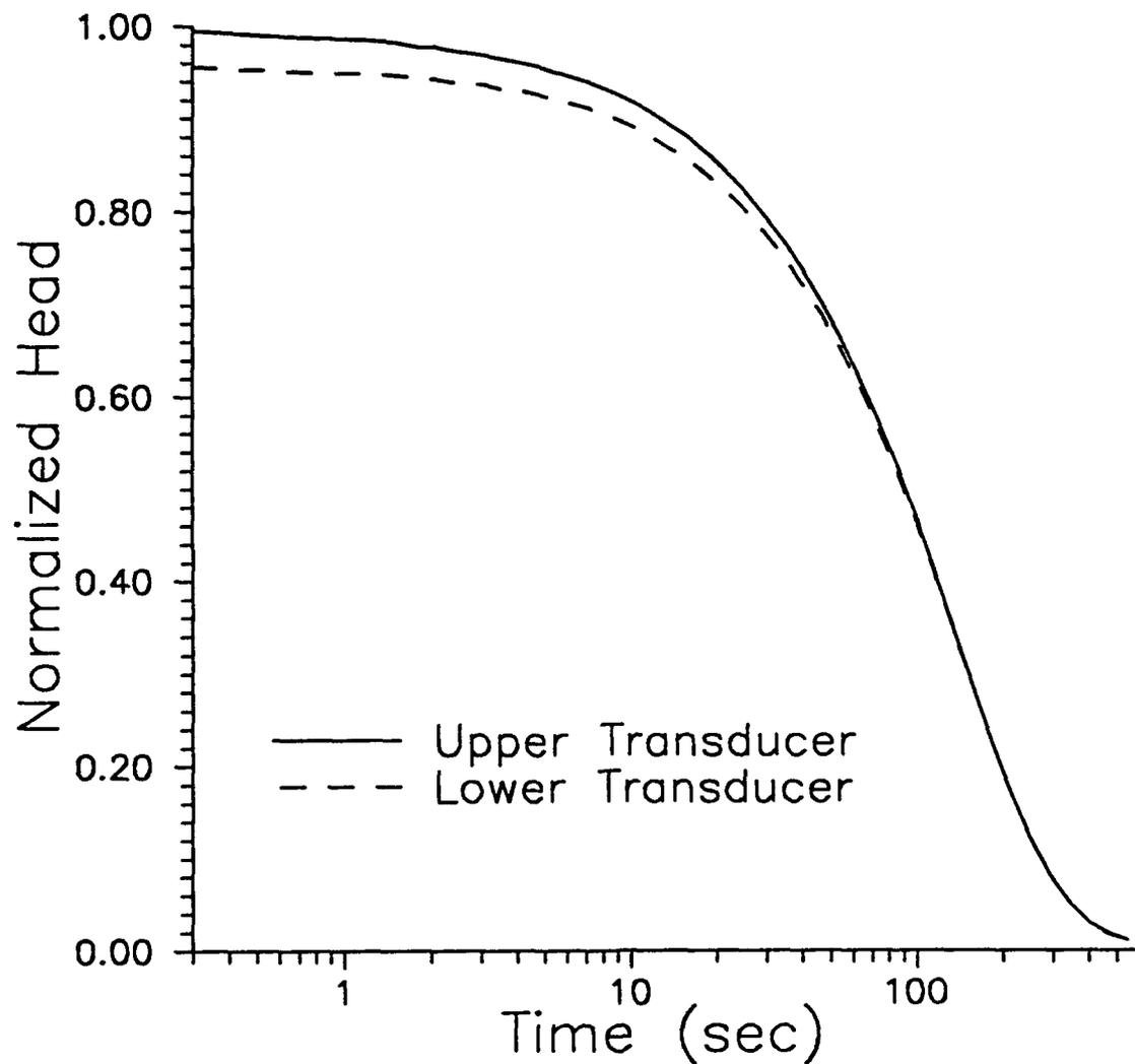
Figure III.B.7 - Normalized head ( $H/H_0$ ) versus time plots for slug test at GEMS well 0-6 ( $H_0 = 7.39$  m). Note that the transducer-packer arrangement described in the text was used in this test.
