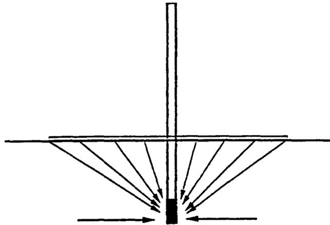
Figure A-2: Vertical cross section through Figure A-1, generalizing ground-water flow paths as straight lines. Note that the flow paths are mostly vertical near the well and increasingly more horizontal with distance from the well.
