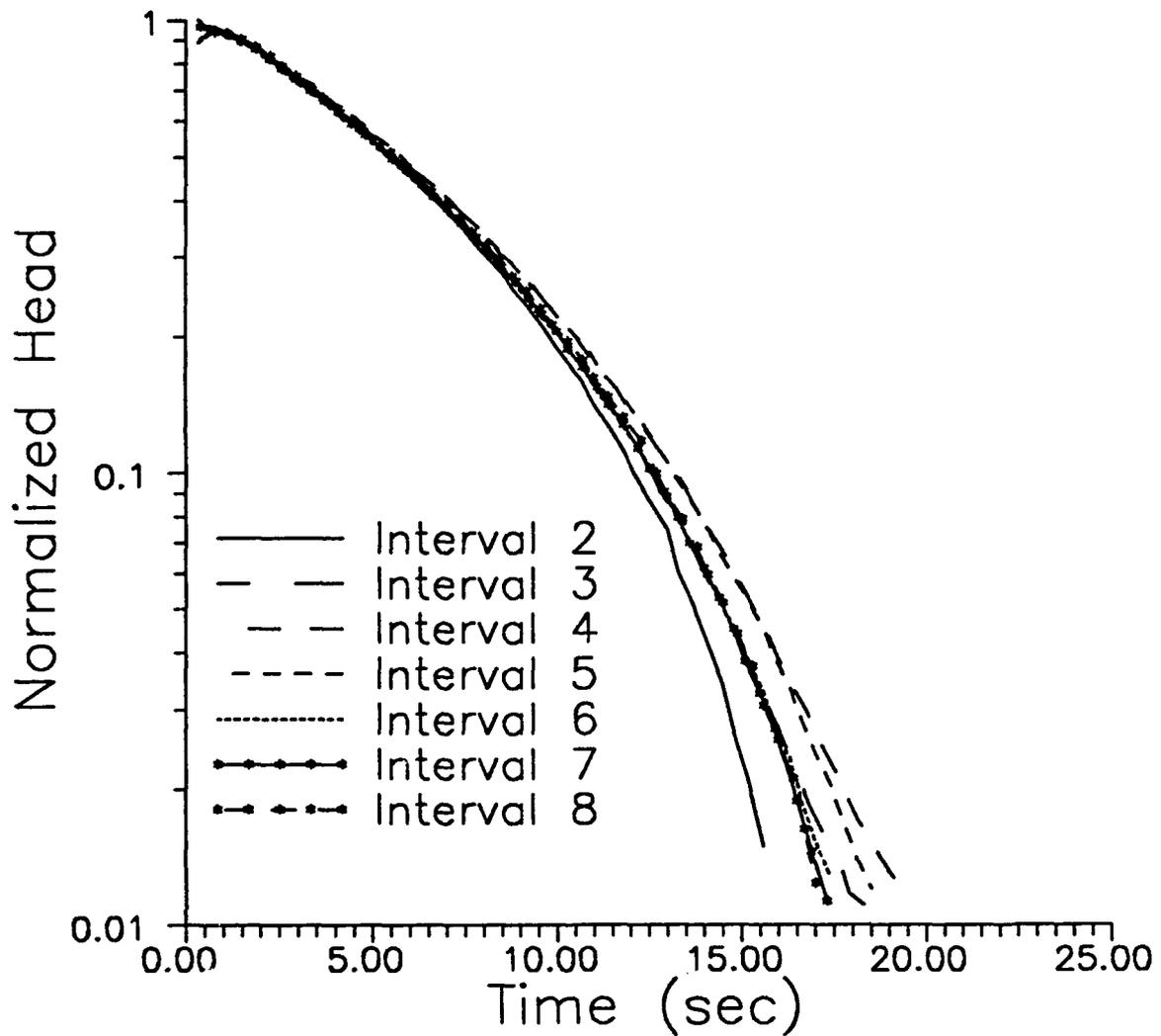
Figure III.B.2 - Normalized head ( $H/H_0$ ) versus time plots for slug tests in seven intervals of GEMS well 2-5 ( $H_0 = 1.52$  m). See Table III.B.1 for depths corresponding to each interval.
