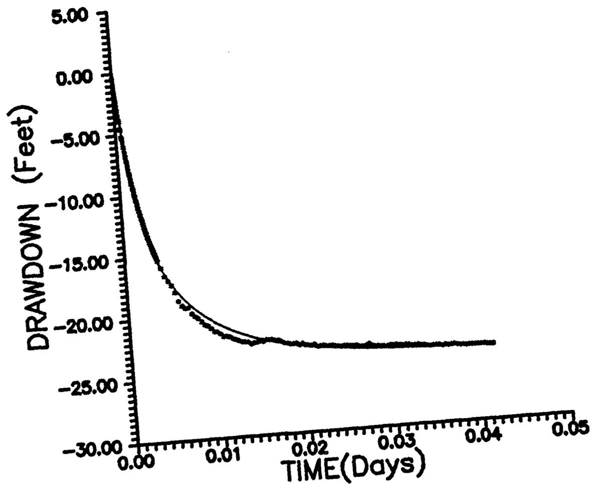
Figure 3. Fit of first period drawdown data to the leaky well function ( solid curve).
