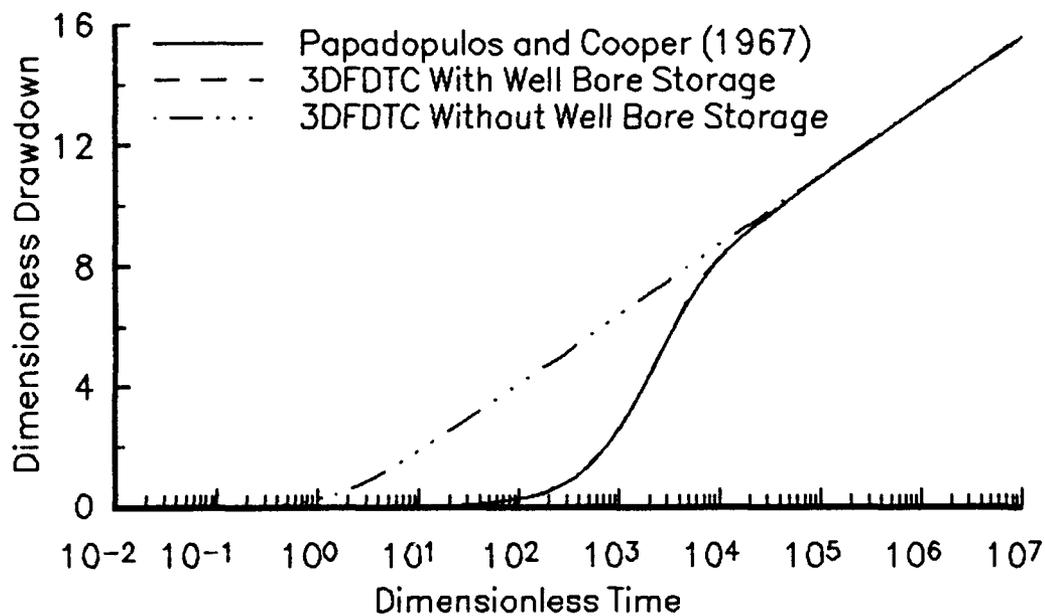
Figure II.A.1 Dimensionless drawdown ( $4\pi Ts/Q$ ) versus time ( $4Tt/Sr^2$ ) plot comparing the Papadopoulos and Cooper (1967) solution with 3DFDTC results. (Observation well is located at  $r=4.6$ ;  $r_w=0.167$ ,  $T=1$  and  $S=10^{-5}$ ; 3DFDTC discretization: 3 radial nodes inside well bore, 39 nodes in the radial from  $r_w$  to 37364.15 meters and 5 nodes in vertical).
