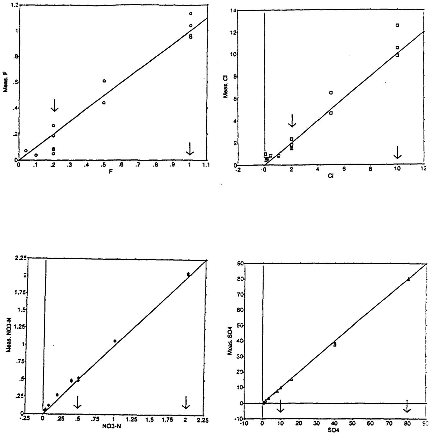
Figure 2: Determination of detection limits on anion concentrations determined by ion chromatography. One to two trials of two measurements each on four anions are used to assess how far below the lower of two calibration standards (concentrations shown by arrows on each graph) one can trust chromatography results. The one-to-one correlation line is shown on each graph. a) Fluoride. b) Chloride. c) Nitrate as mg/L nitrogen. d) Sulfate.
