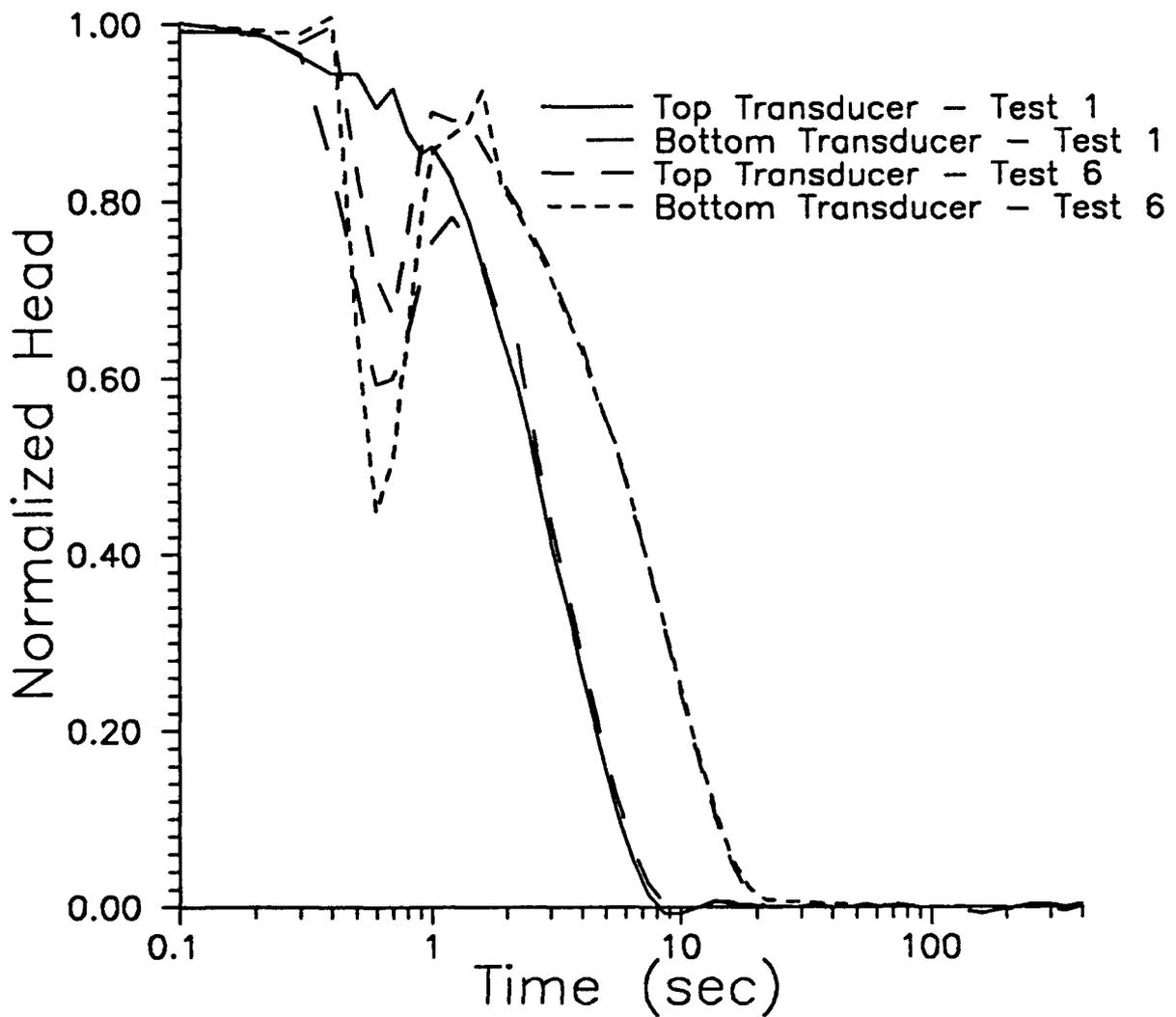
Figure III.B.6 - Normalized head ( $H/H_0$ ) versus time plots for two slug tests at GEMS well 10-1 ( $H_{01} = 1.07$  m;  $H_{06} = 6.83$  m). Note that two transducers were used in each test.
