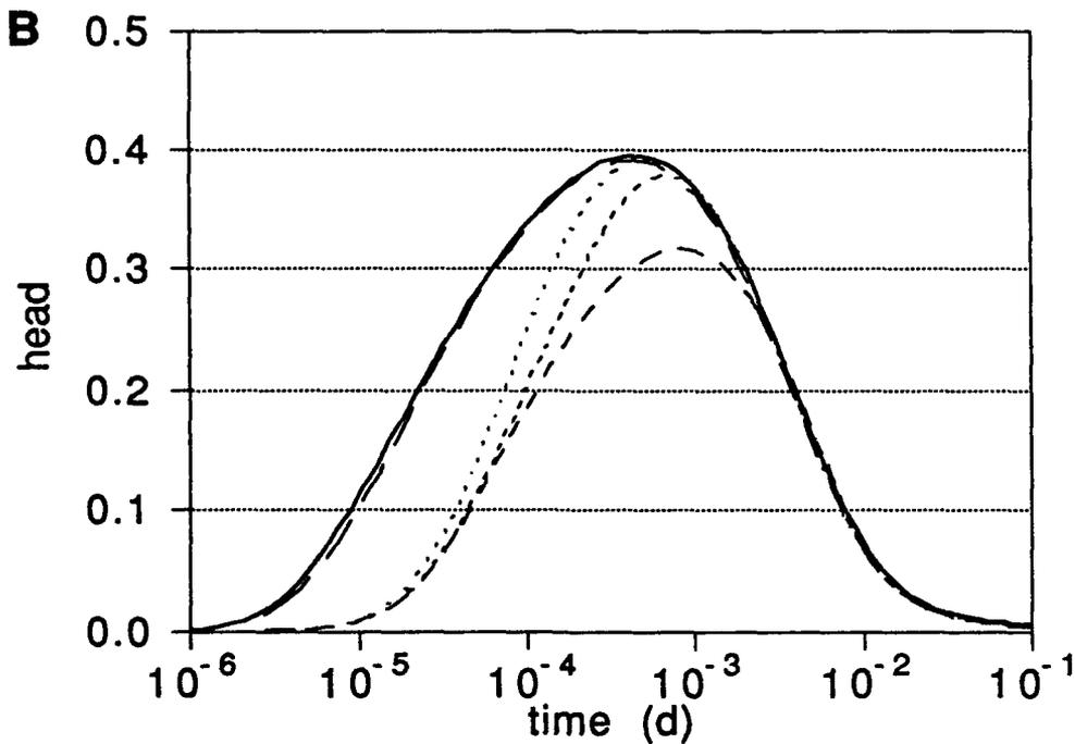
**Figure II.B.1:** Effects of variable layering on fully-penetrating slug test results at (A) the slugged well and (B) an observation well located at vertical node 13 and 3.7 meters radial distance from the slugged well. Layering schemes are shown in Figure II.B.2.
