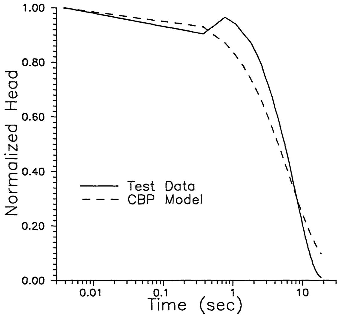
Figure III.B.4 - Normalized head ( $H/H_0$ ) versus time plots of slug-test data from interval 3 (19.77-20.05 m) of GEMS well 2-5 and the best-fit CBP model.
