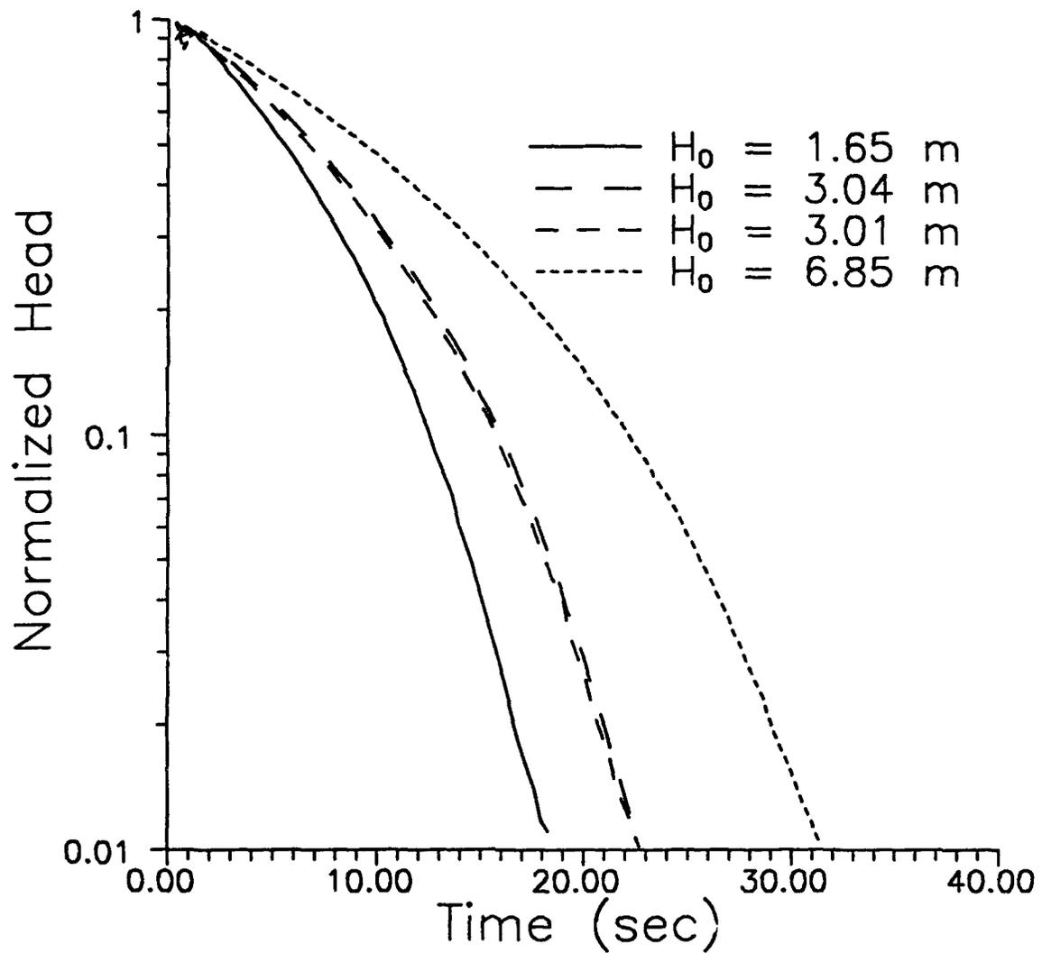
Figure III.B.3 - Normalized head ( $H/H_0$ ) versus time plots for slug tests in the third interval (19.77-20.05 m) of GEMS well 2-5 using  $H_0$ 's of different magnitudes.
