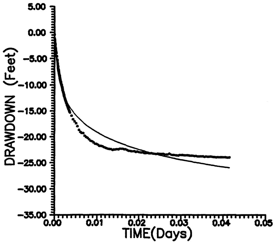
Figure 2. Fit of first period drawdown data to the Theis well function (solid curve).
