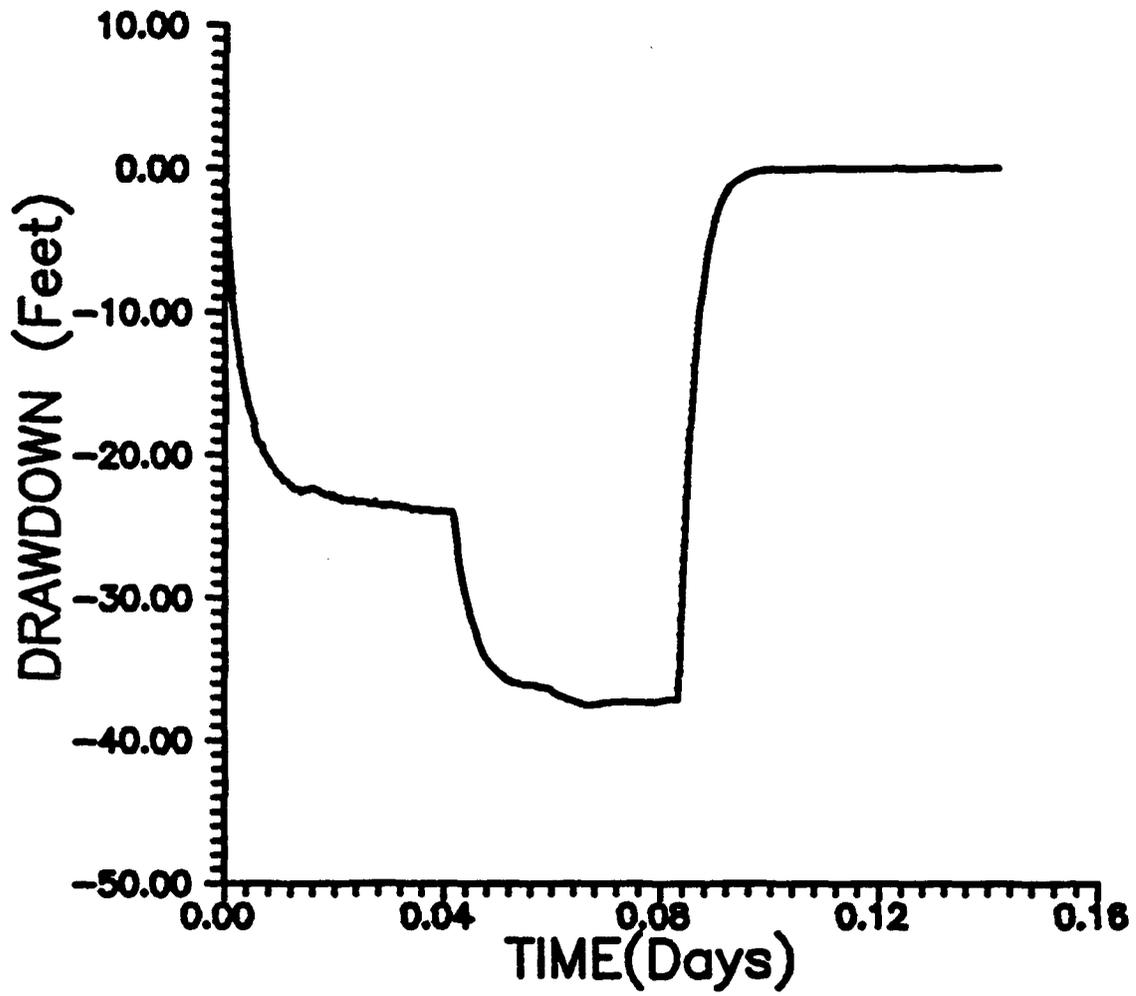
Figure 1. Drawdown data from all three periods (two pumping and one recovery).
