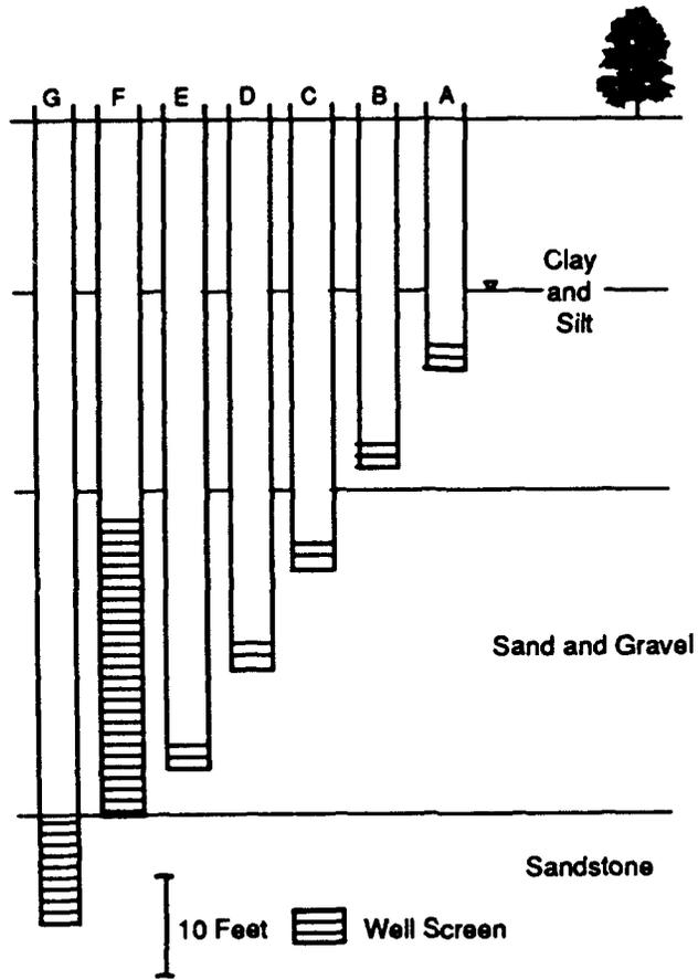
Figure 2. A typical well nest cross-section
