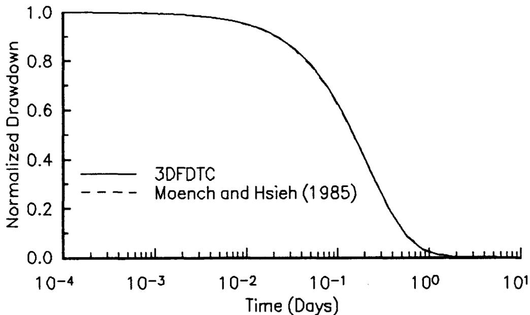
Figure II.A.2 Normalized drawdown ( $H/H_0$ ) versus time plot comparing Moench and Hsieh (1985) solution with 3DFDTC results. ( $r_w=0.167$ ,  $r_{skin}=0.333$ ,  $T_{skin}=10^{-3}$ ,  $S_{skin}=10^{-3}$ ,  $T_{aquifer}=1$ ,  $S_{aquifer}=10^{-5}$ ; discretization as in Figure II.A.1 except that 3 of the 39 radial nodes are placed between  $r_w$  and  $r_{skin}$ ).
