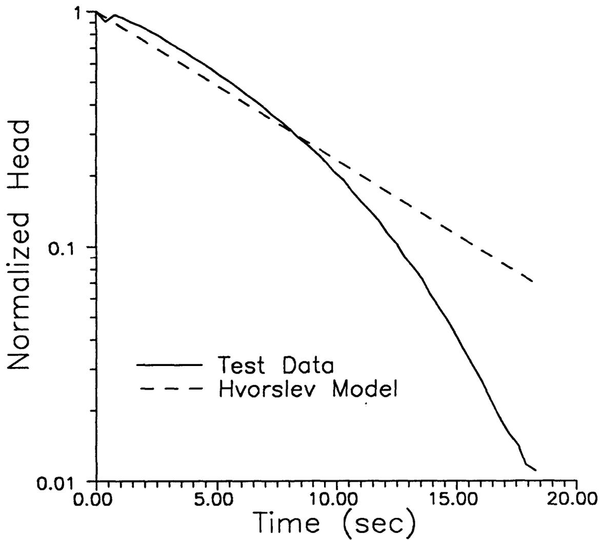
Figure III.B.5 - Normalized head ( $H/H_0$ ) versus time plots of slug-test data from interval 3 (19.77-20.05 m) of GEMS well 2-5 and the best-fit Hvorslev model.
