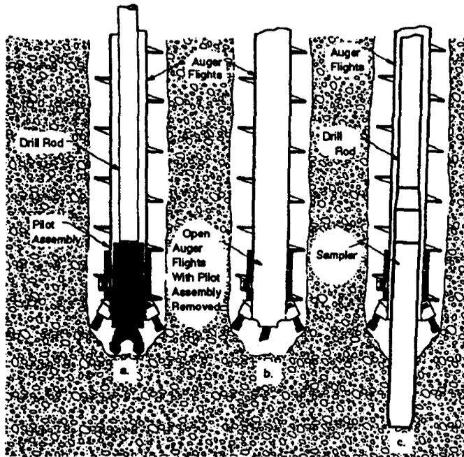
Figure 1. Sequential steps showing borehole advancement with pilot assembly and collection of a formation sample (after Riggs 1983).
