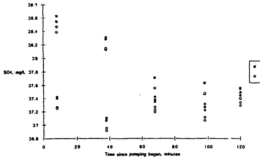
Figure 4: Variation in anion concentrations during bedrock pumping test, and predictions of concentrations of F, Cl and SO<sub>4</sub> based on NO<sub>3</sub>-N content. For each anion, an aliquot from two bottles was analyzed twice, resulting in four values for each anion for each time step (filled squares). Predicted results (unfilled diamond) are discussed in the text. a) NO<sub>3</sub>-N. b) F. c) Cl. d) SO<sub>4</sub>.
