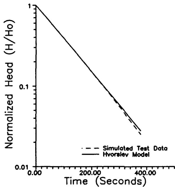
Figure II.B.16 - Plot showing the results of the Hvorslev analysis applied to simulated test data from Scenario 7A
