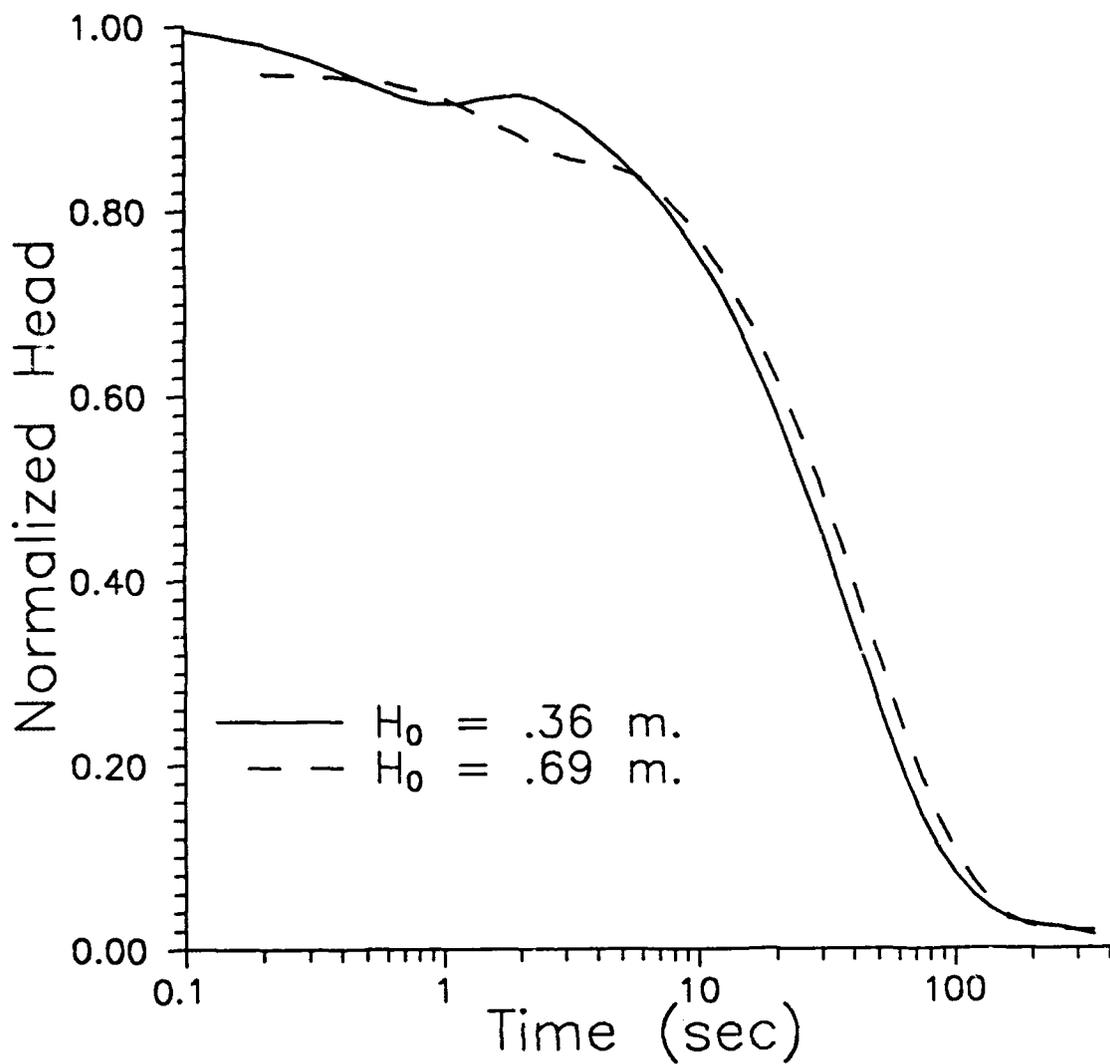
Figure III.B.8 - Normalized head ( $H/H_0$ ) versus time plots for two slug tests at GEMS well 0-6 ( $H_{01} = 0.36$  m;  $H_{02} = 0.69$  m). Note that these slug tests were initiated using the PVC pipes described in the text.
