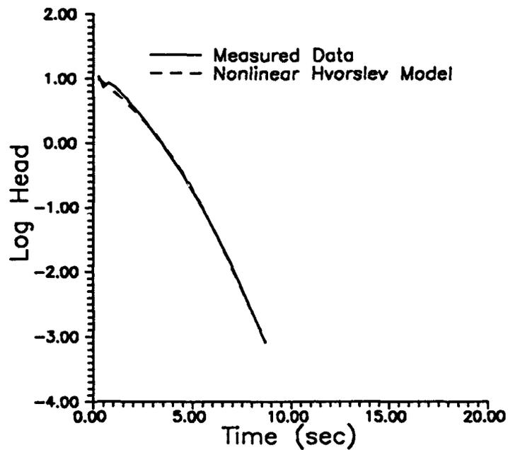
Figure III.C.1 - Natural logarithm of head versus time plots of slug-test data from GEMS well 0-2 ( $H_0 = 0.88$  m) and the best-fit nonlinear Hvorslev model
