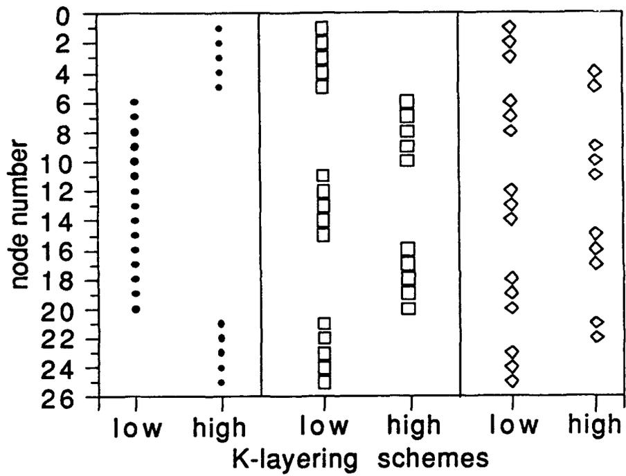
Figure II.B.2: Layering schemes employed for results shown in Figure II.B.1. Low and high hydraulic conductivities are those for the layered, anisotropic aquifer.
