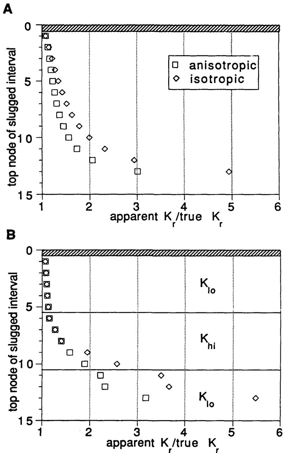
**Figure II.B.3:** Effects of slugged interval length in the uniform (A) and the layered (B) aquifers. Slugged interval is centered at vertical node 13 and its length increases symmetrically up to the full thickness of the aquifer (25 nodes). Note that the  $K$ -configurations are also symmetric about node 13.
