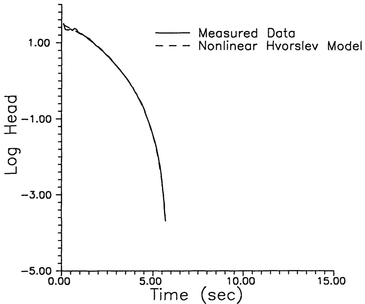
Figure III.C.3 - Natural logarithm of head versus time plots of slug-test data from a fully penetrating slug test at GEMS well 2-5 ( $H_0 = .79$  m) and the best fit nonlinear Hvorslev model.
