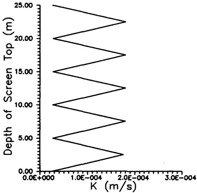
Figure II.B.12 - Conductivity versus depth plot for Scenario 3 of Table II.B.1
