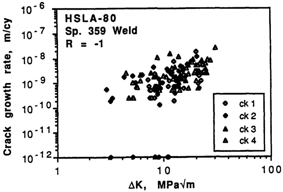
Figure 24. Fatigue crack growth rate, rotating beam test, for sp. 359, weld metal.
