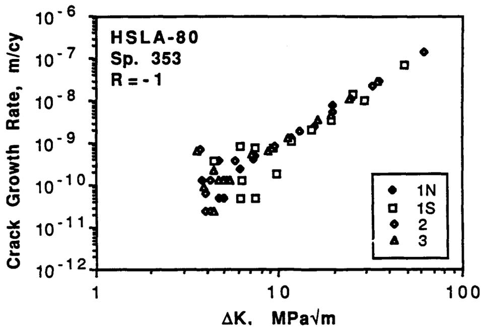
Figure 20. Fatigue crack growth rate for as-received material (Lehigh plate) from rotating beam test, sp. 353, stress amplitude = 550 MPa.
