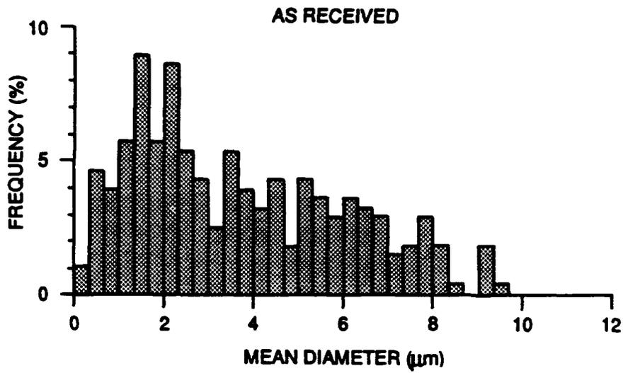
Figure 9. Grain size distribution in the as-received HSLA 80 plate.
