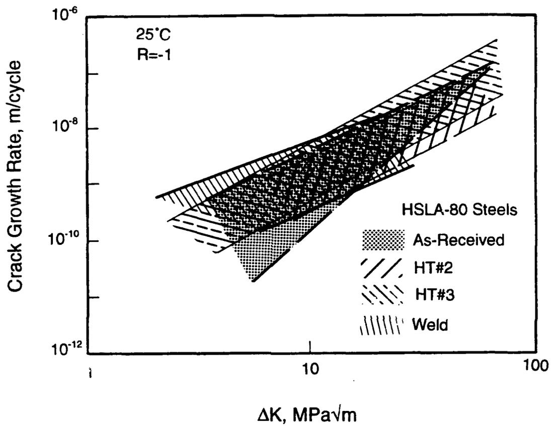
Figure 30. Comparison of fatigue crack growth responses of microcracks in HSLA-80 steels and weld.
