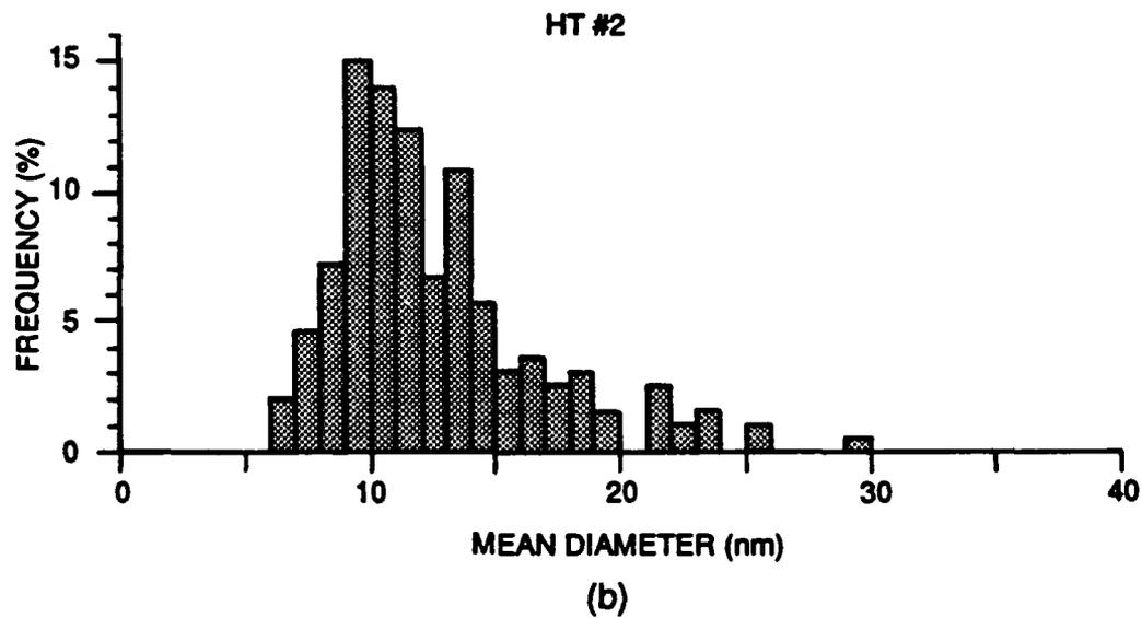
Figure 7. Distribution of  $\epsilon$ -copper precipitates in HSLA steels: (a) as-received, (b) HT#2, (c) HT#3, and (d) weld.
