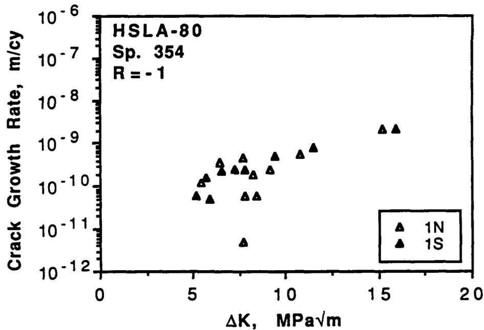
Figure 21. Fatigue crack growth rate for as-received material (Lehigh plate) from rotating beam test, sp. 354, stress amplitude = 520 MPa.
