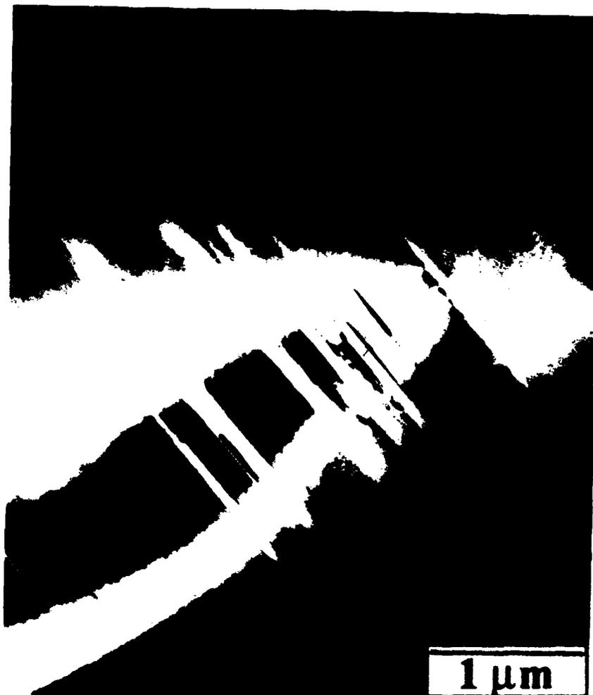
**Figure 12.** Transmission electron micrograph of as-arc-cast Al<sub>67.5</sub>Ti<sub>25</sub>Fe<sub>7.5</sub> alloy, showing a large faulted precipitate.
