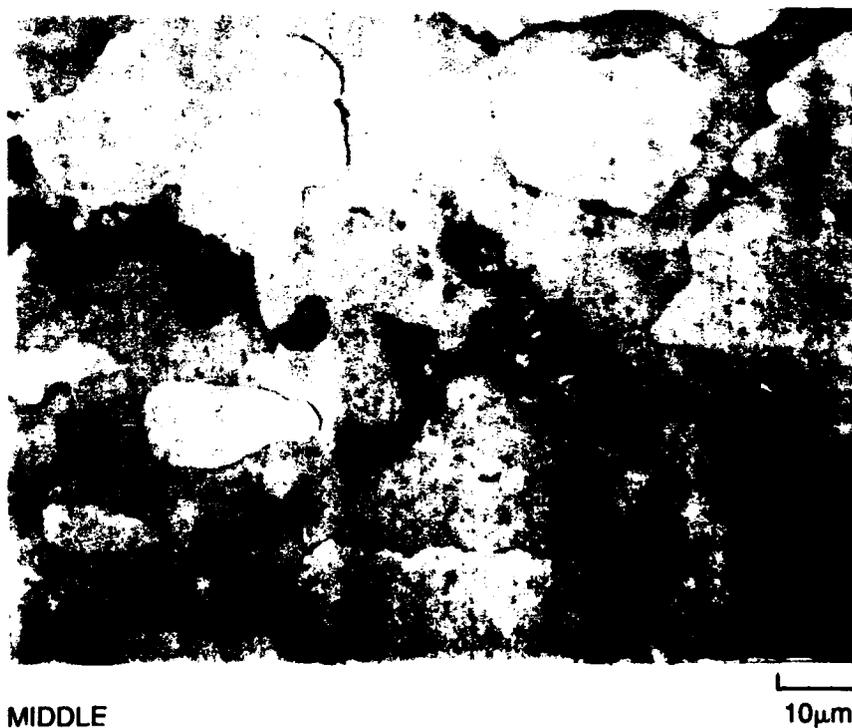
**Figure 34 Representative microstructures of Al-16.75 at% Ti-8.25 at% Nb-7.5 at% Fe following casting and HHT for 240 h.**
