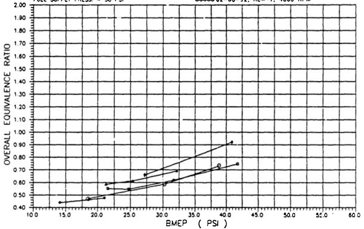
Figure 16. Calculated Overall Equivalence Ratio vs. Brake Mean-Effective Pressure
