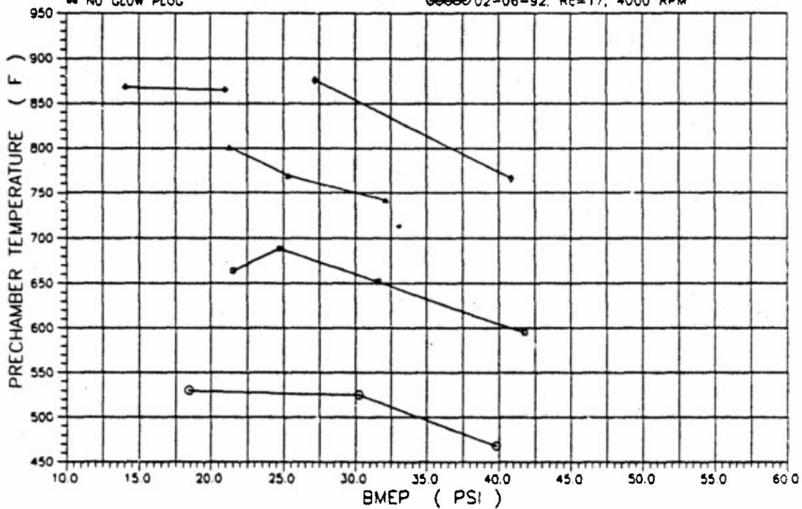
Figure 13. Pre-Chamber Temperature vs. Brake Mean-Effective Pressure
