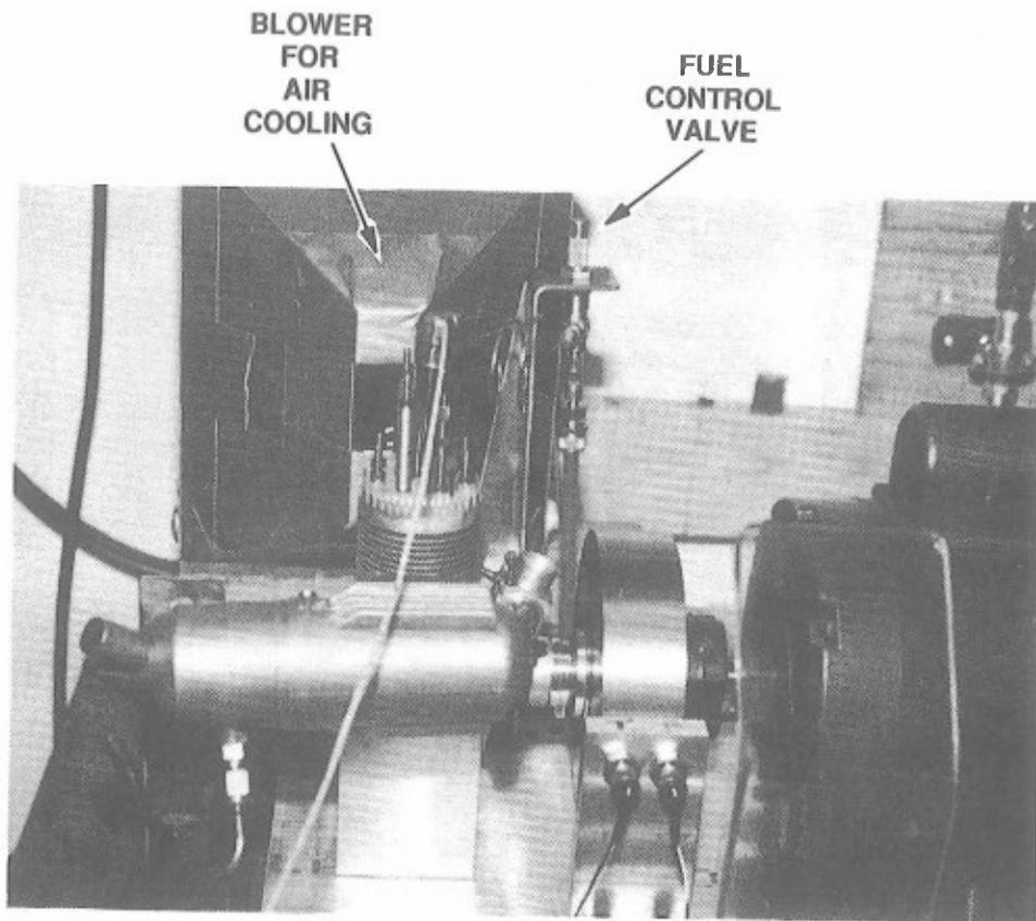
Figure 7. Test Engine with Flywheel and Coupling
