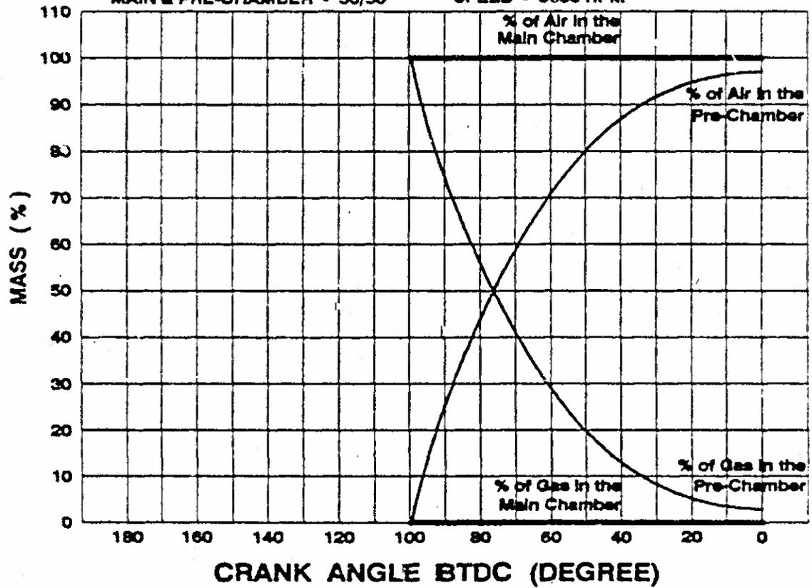
Figure 2. Percent Mass Distribution vs. Crank Angle
