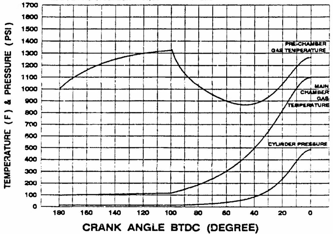
Figure 1. Chamber Temperature and Pressure vs. Crank Angle
