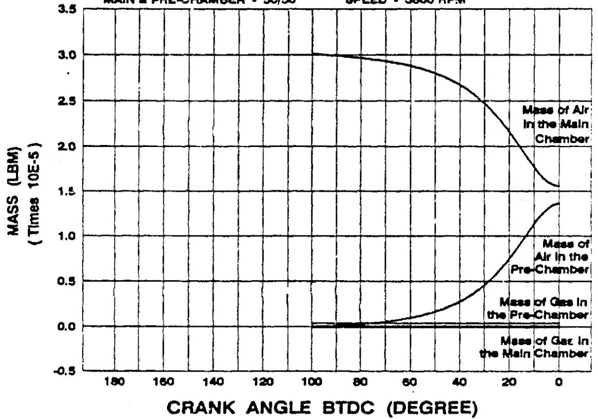
Figure 3. Mass Distribution vs. Crank Angle
