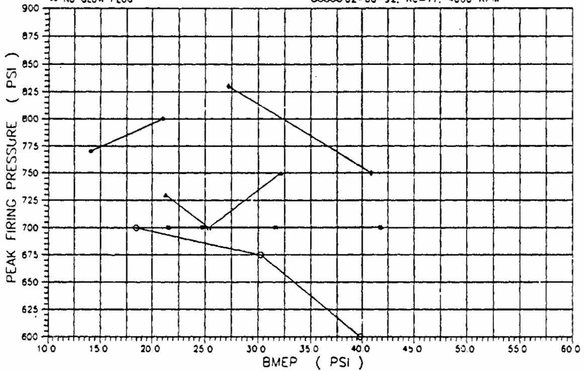
Figure 12. Peak Firing Pressure vs. Brake Mean-Effective Pressure
