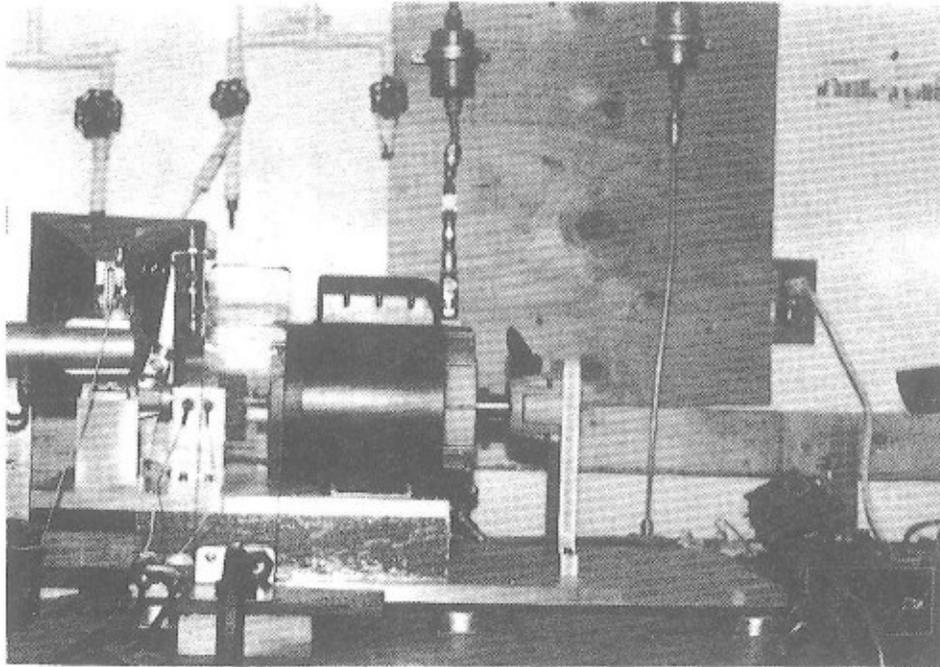
Figure 21. Test Facility Showing Hand-Cranking Device
