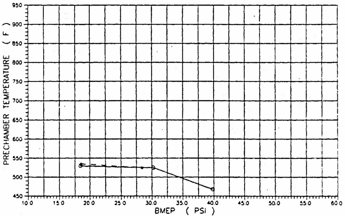
Figure 20. Pre-Chamber Temperature vs. Brake Mean-Effective Pressure (Comparison of Different Fuels)
