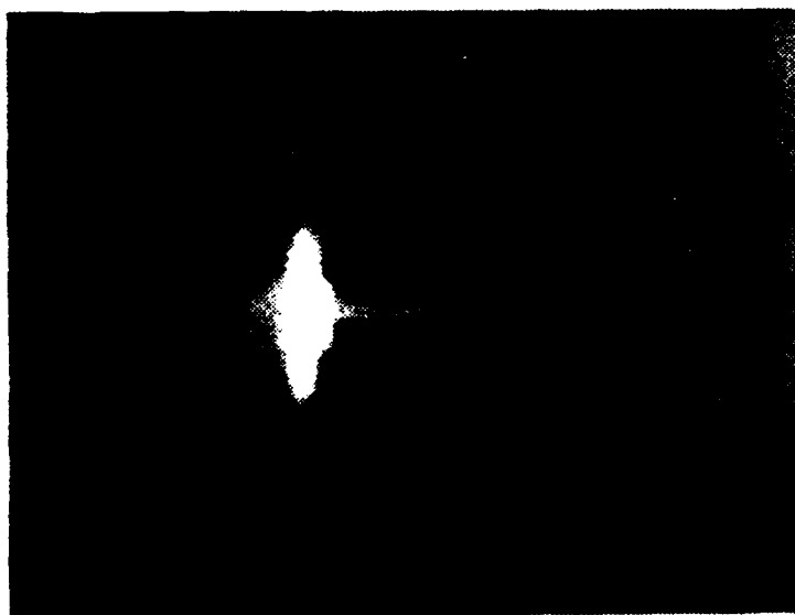
Figure 2. Photograph of the window breakdown without magnets installed on the waveguide.
