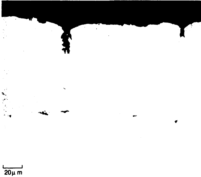
Figure 13. TMF Cracks in LPPS NiCoCrAlY After 1000 Cycles
