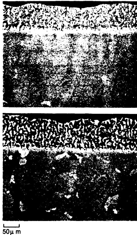
Figure 53. Longitudinal Section of the Lathe-Polished and As-Tumbled TMF Samples shown in Figure 52
