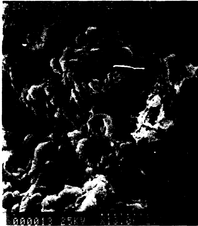
Figure C17. Grab sample 890-085 (WIPP-2 SM-6). Aggregate surface that was exposed to brine
