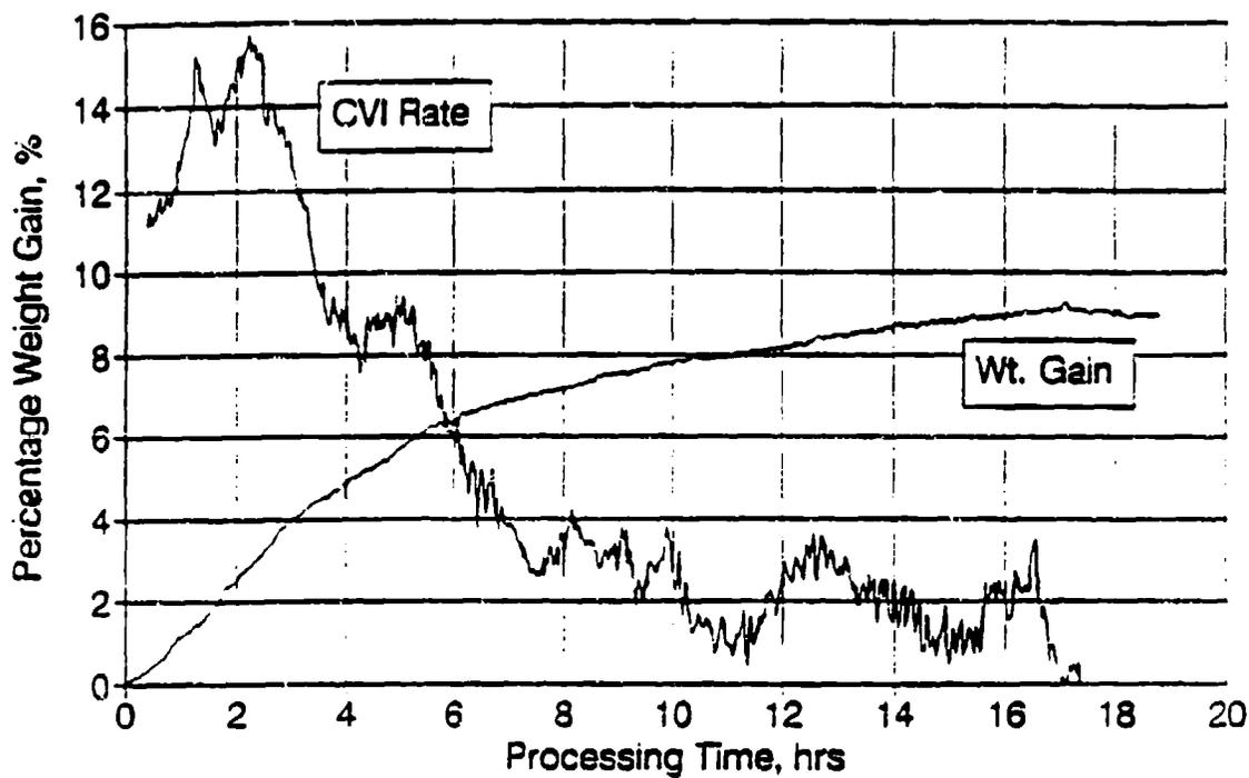
Figure 4-3. CVI Weight Gain and Rate Curves
