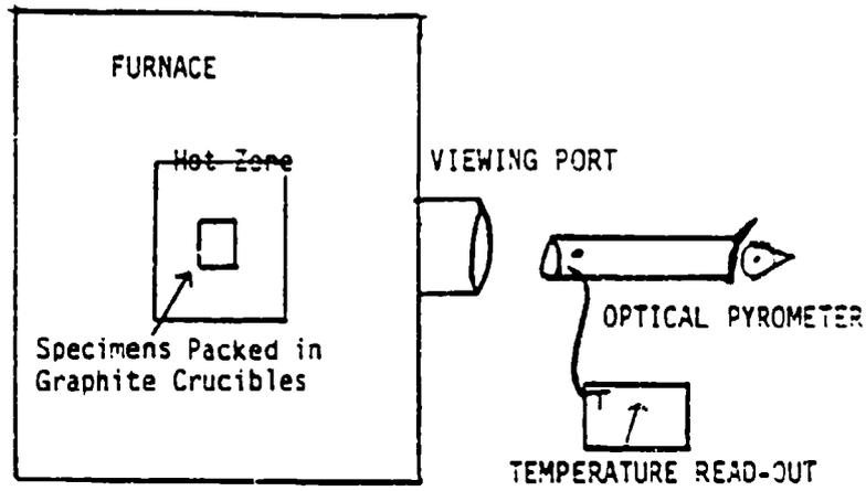
Figure 7. TEMPERATURE MEASUREMENT.
