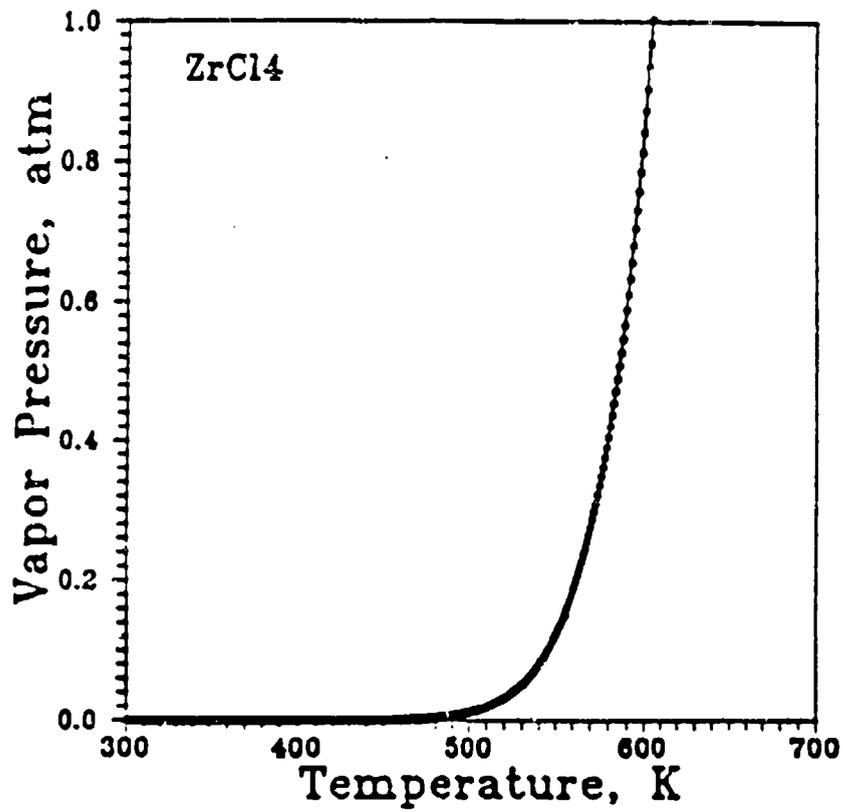
Figure 3-3. Calculated equilibrium vapor pressure of ZrCl<sub>4</sub> as a function of temperature. Note the vapor pressure increases drastically near the sublimation point of ZrCl<sub>4</sub>, 604°K (331°C).
