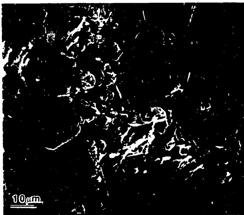
Figure 36b. SEM micrograph of an inhibited matrix composite packed cemented in the  $\text{ZrC/SiC/Si/Al}_2\text{O}_3$  mixture and oxidized at  $1000^\circ\text{C}$ .
