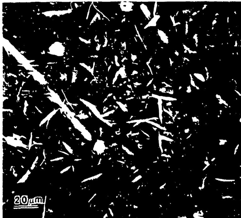
Figure 41b. SEM micrograph of an inhibited matrix composite packed cemented in the SiC/Si/Al<sub>2</sub>O<sub>3</sub> mixture and oxidized at 1200°C.
