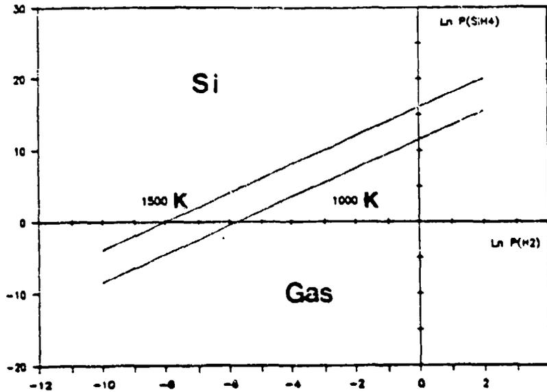
Figure 4-1. Calculated equilibrium lines in  $\text{SiH}_4\text{-H}_2$  system at  $1000^\circ\text{C}$  and  $1500^\circ\text{C}$ .
