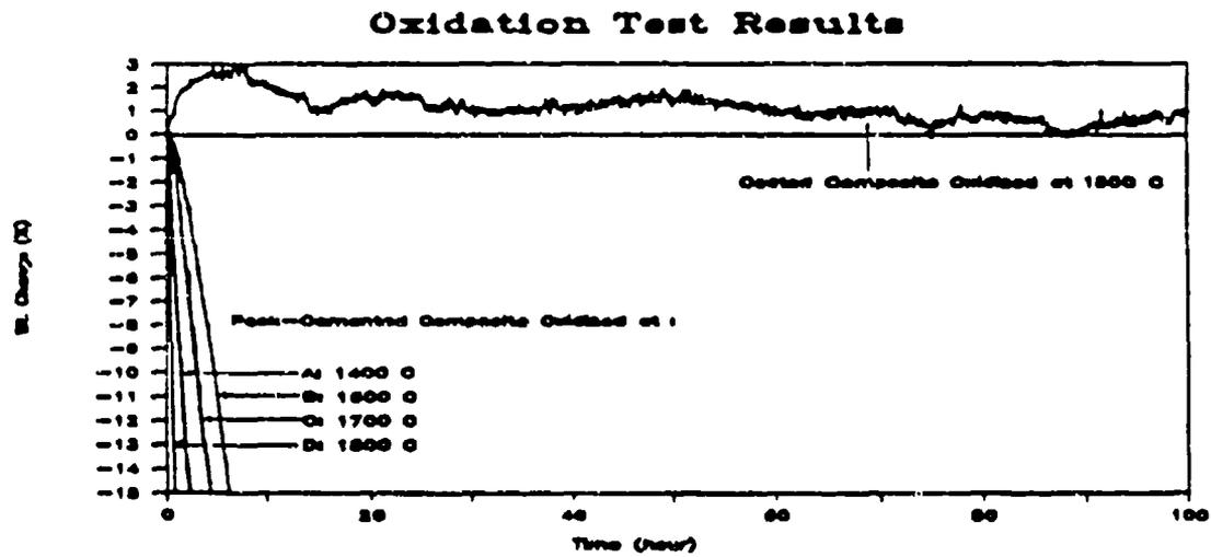
Figure 4-35. TGA result of a composite protected by a graded SiC + ZrC coating at 1500°C in air, as compared with test results of pack-cemented composite.
