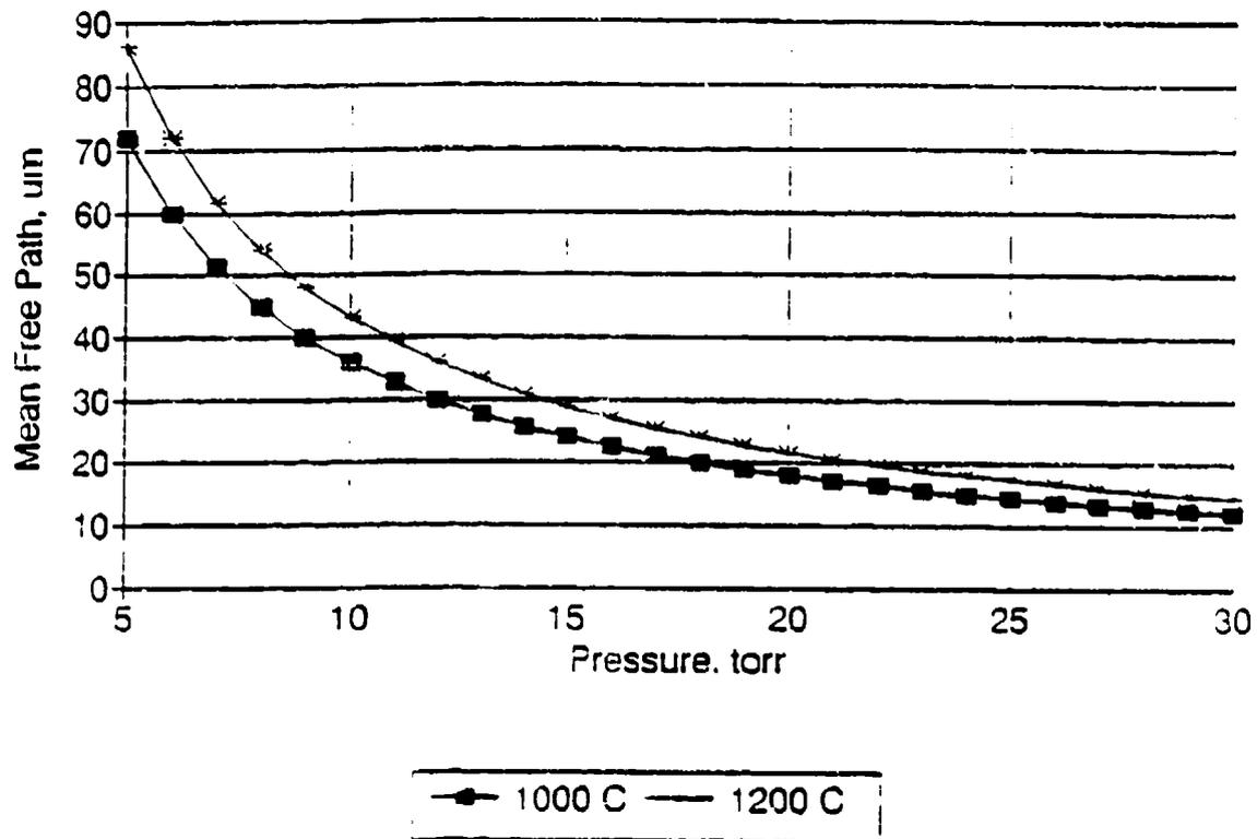
Figure 5-3. Mean-Free-Path of CH<sub>4</sub> Molecules in the CVI Experiment Range
