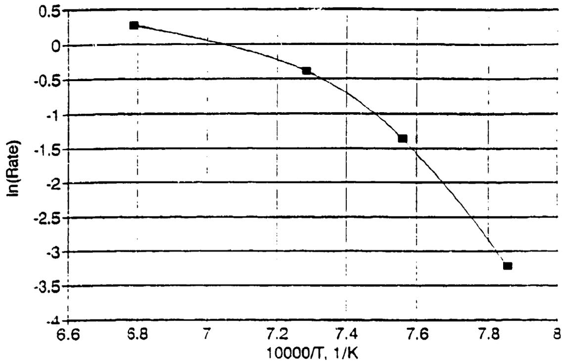
Figure 5-2. Arrhenius Plot of CVI Rate Showing Mixed Mechanism Control as Suggested by Equation 5-
