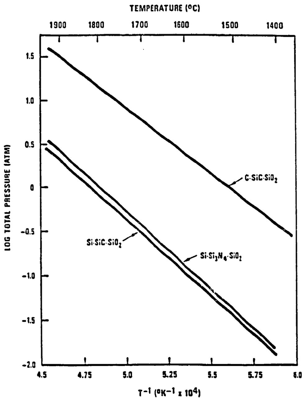
Figure 2-2. Reduction of  $\text{SiO}_2$  by SiC.
