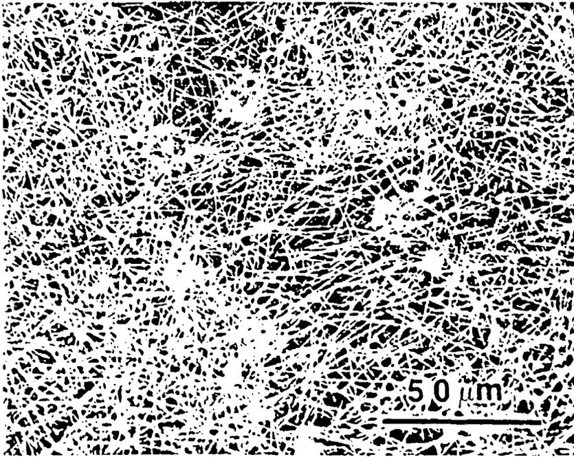
Figure 4-10. SEM micrograph of SiC whisker formed on carbon substrate surface during SiO vapor treatment.
