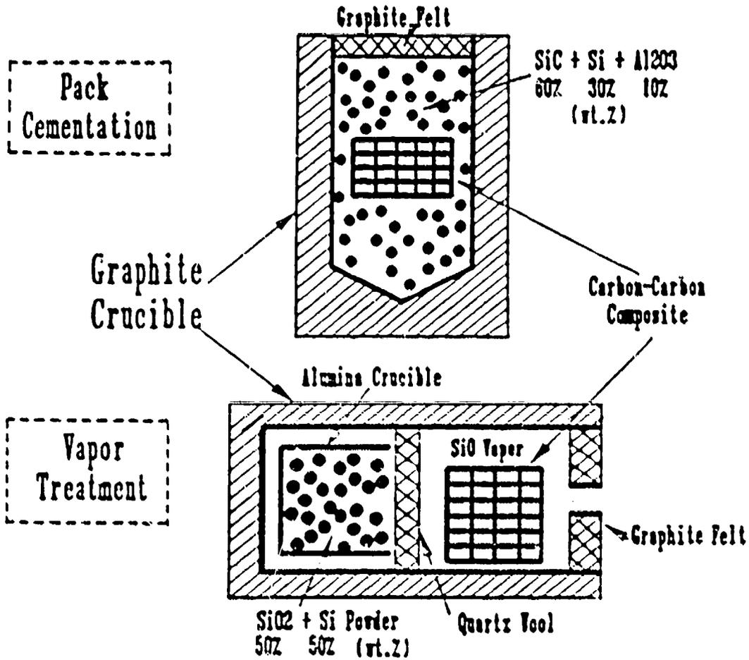
Figure 3-1b. Schematic diagram of reactors for pack cementation and SiO vapor treatment experiments.
