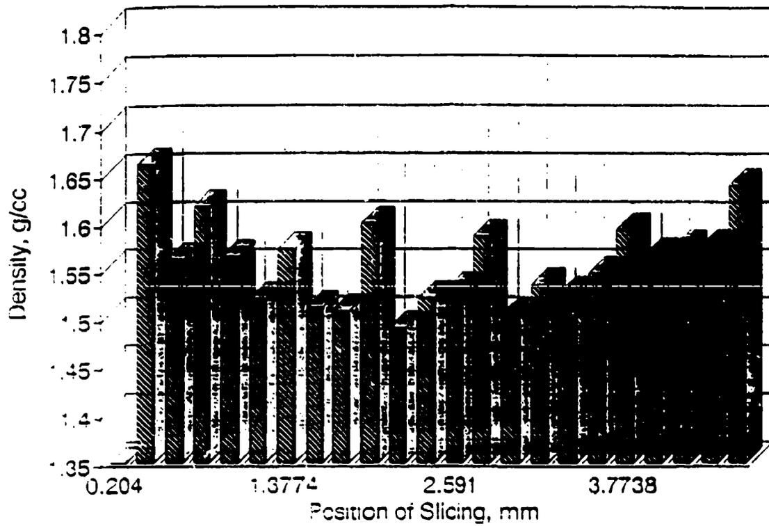
Figure 4-10. Density Profile of the 1050°C/5 torr Processed Specimen
