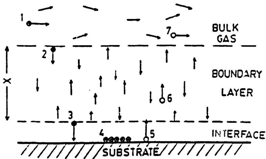
Figure 2-8. Schematic diagram showing the seven steps which occur during a CVD process.
