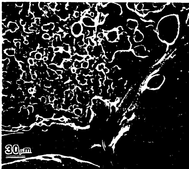
Figure 57b. SEM micrograph of an inhibited matrix composite packed cemented in the  $\text{ZrC}/\text{SiC}/\text{Si}/\text{Al}_2\text{O}_3$  mixture and oxidized at  $1600^\circ\text{C}$ .
