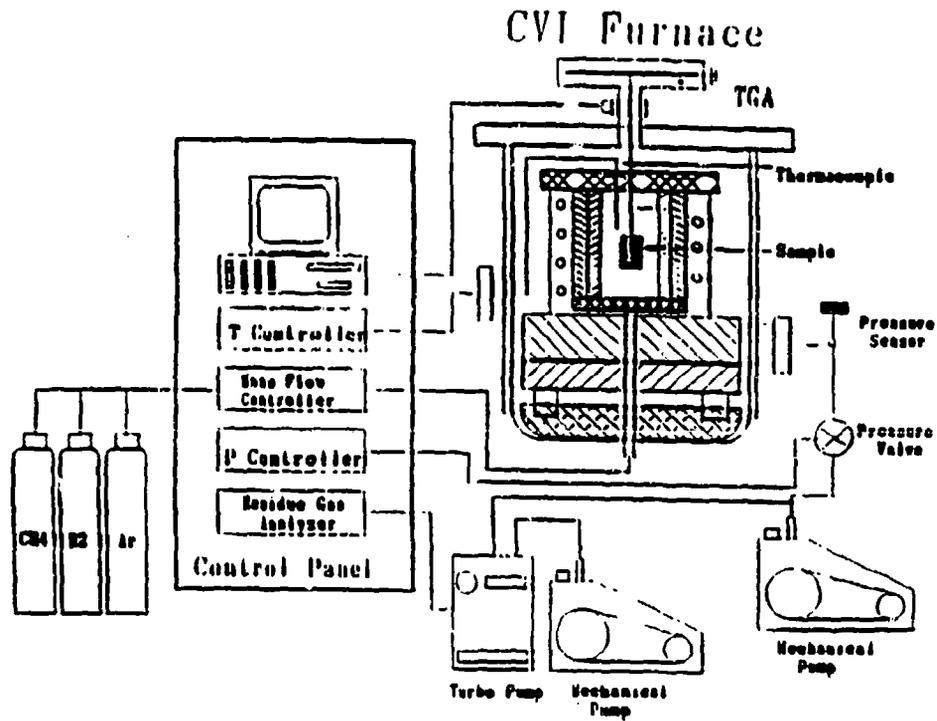
Figure 3-1. Schematic Diagram of CVI Apparatus
