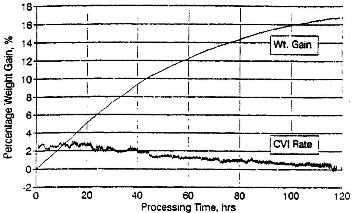
Figure 4-1. CVI Weight Gain and Rate Curves
