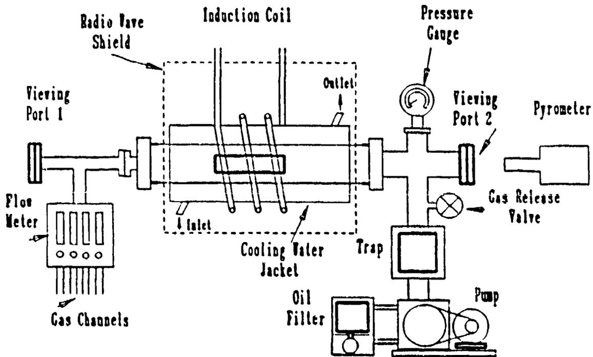
Figure 3-1a. Schematic diagram showing the induction furnace used for pack cementation and SiO vapor treatment. The cooling water jacket around the reactor tube makes heat treatment temperature in excess to 2000°C possible.
