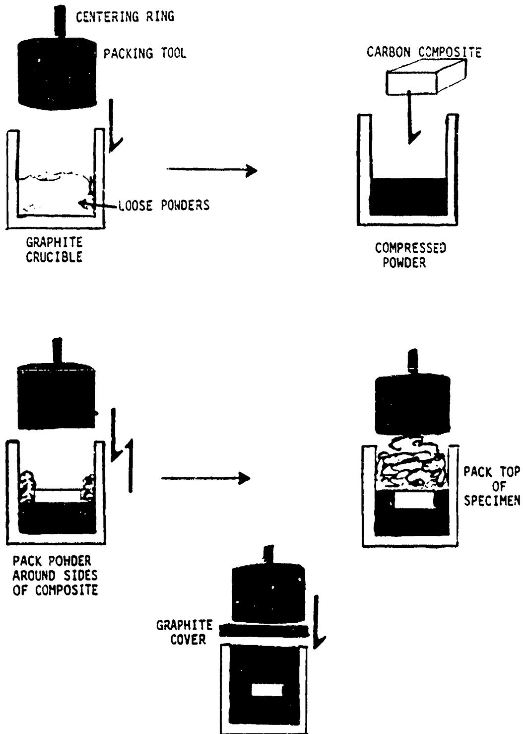
Figure 6. Sample Preparation in Pack Cementation
