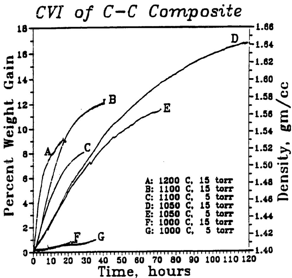
Figure 4-5. Comparison of CVI Weight Gain Curves under Different Experiment Conditions
