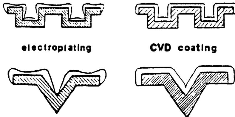
Figure 2-10. Comparison electroplating and CVD coating structures.
