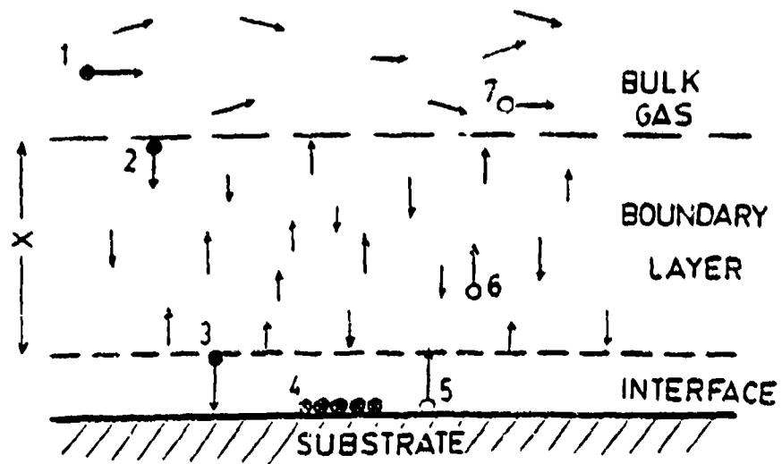
Figure 2-1. The Seven Mechanistic Steps to Describe Heterogeneous Reactions
