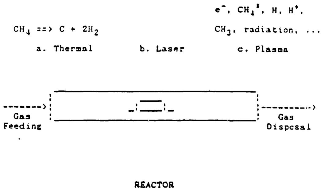
Figure 2-4. Schematic diagram showing various methods which can be used to activate CVD reactions.
