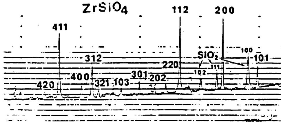
Figure 4-39. X-ray diffraction spectrum of ZrC + SiC graded coating obtained using flow condition shown in Figure 4-34. The oxidized surface was identified as  $ZrSiO_4$  with little amount of  $SiO_2$ .
