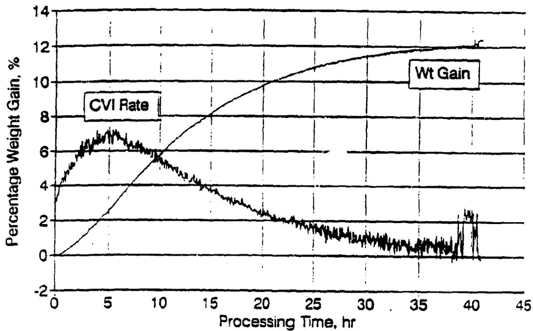
Figure 4-2. CVI Weight Gain and Rate Curves
