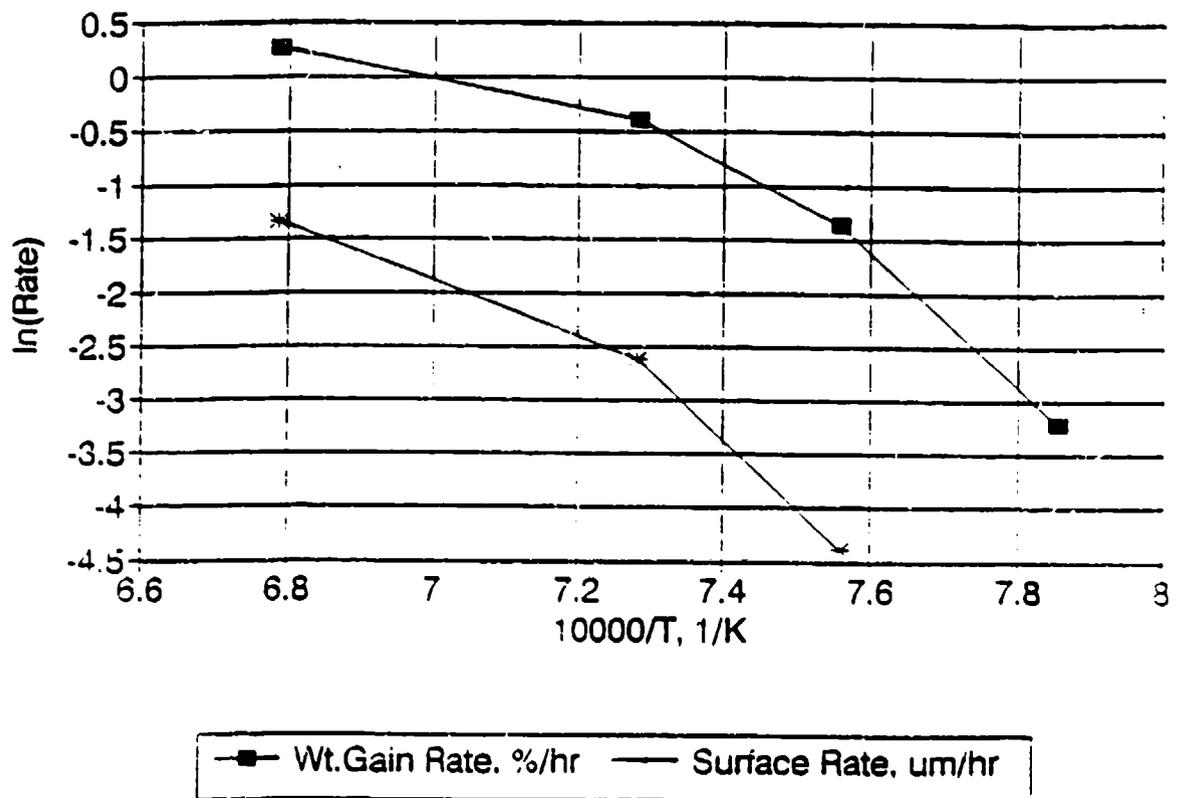
Figure 5-1. Comparison of Arrhenius Relation of CVI Rate Obtained from Weight Gain Measurement and Surface Deposit Thickness Measurement
