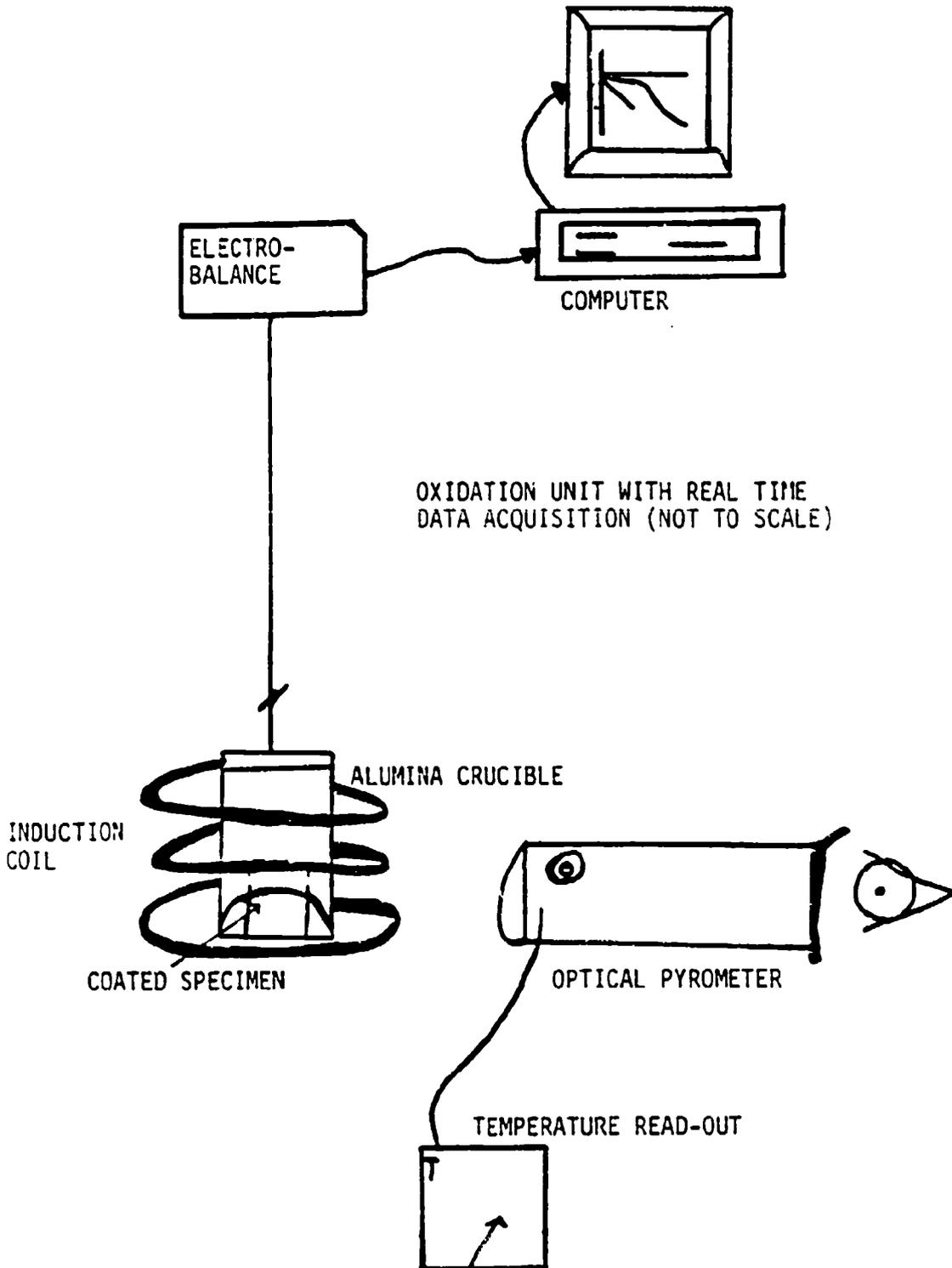
Figure 10. Oxidation Unit.
