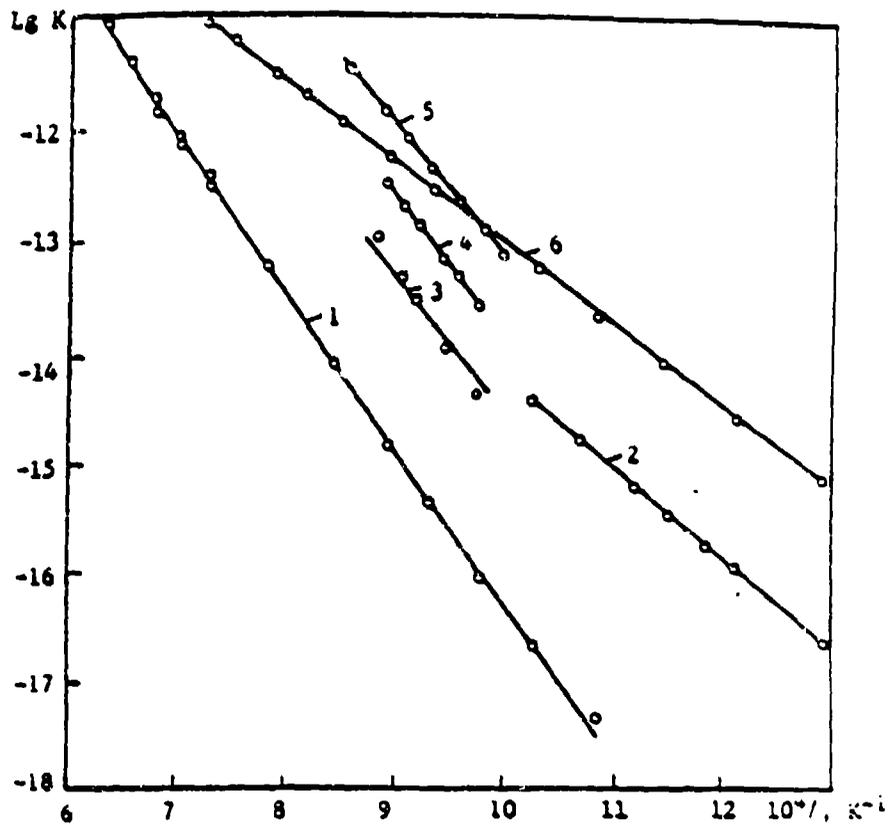
Figure 2-4. Logarithms of rate constants of PyC formation from individual hydrocarbons ( $\text{g cm}^{-2} \text{s}^{-1} \text{Pa}^{-1}$ ): 1, methane; 2, ethylene; 3, benzene; 4, naphthalene; 5, anthracene; 6, acetylene.
