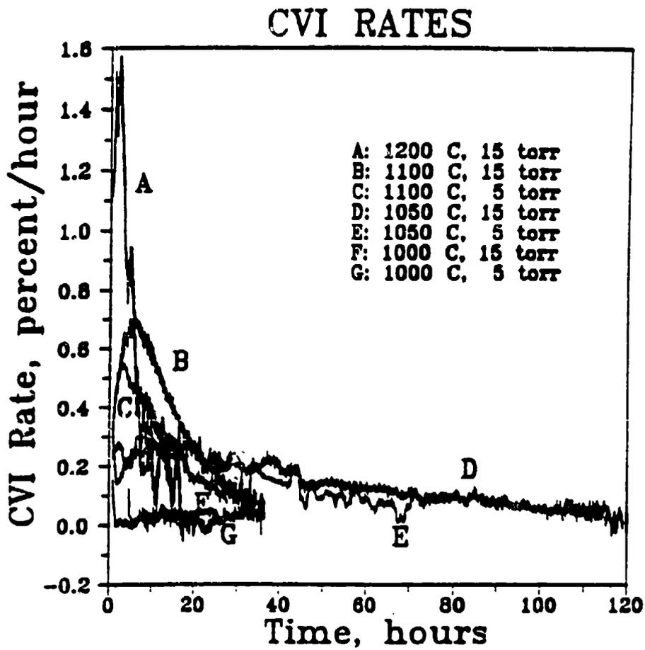
Figure 4-6. Comparison of CVI Rate Curves under Different Experiment Conditions
