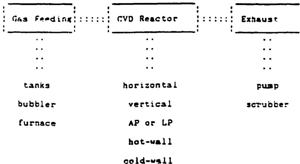
Figure 2-5 Three major components in a CVD system.
