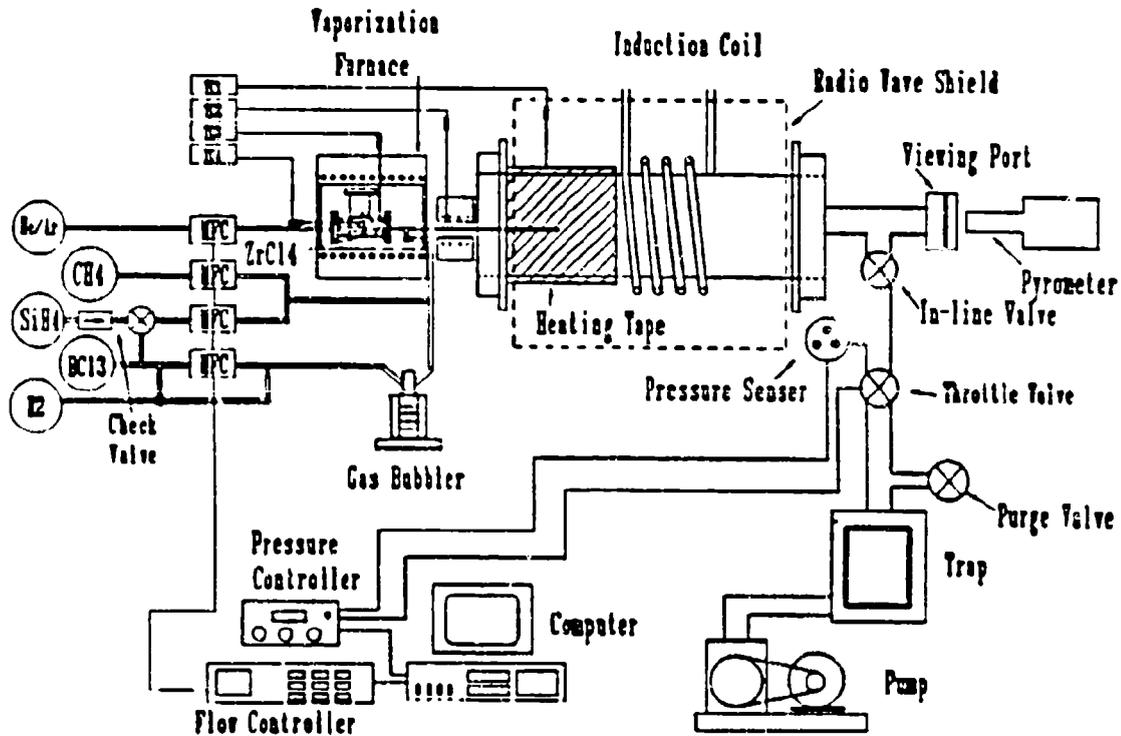
Figure 3-2. Detailed design of the computer-controlled CVD device used in this study. Note that the sensing/control of pressure and flow rates are both interfaced with the computer.
