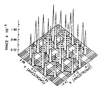
Traces of the elastic modulus tensor for a hexagonal planar array of carbon atoms (after Thacher <u>et al</u>, 1986).
