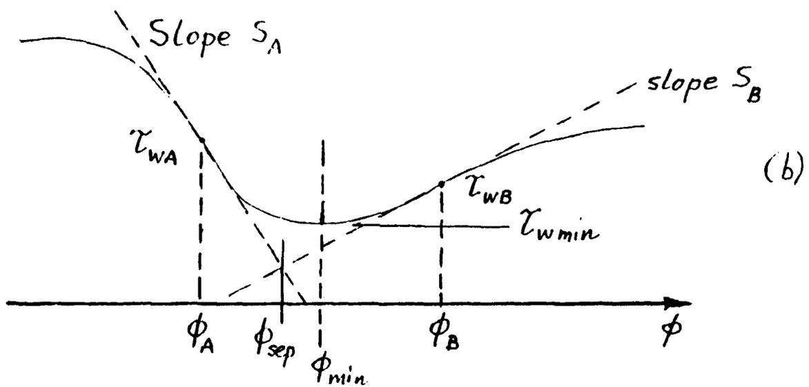
Figure A.3 Examples of variations of the wall shear stress magnitude in the vicinity of a local minimum:
