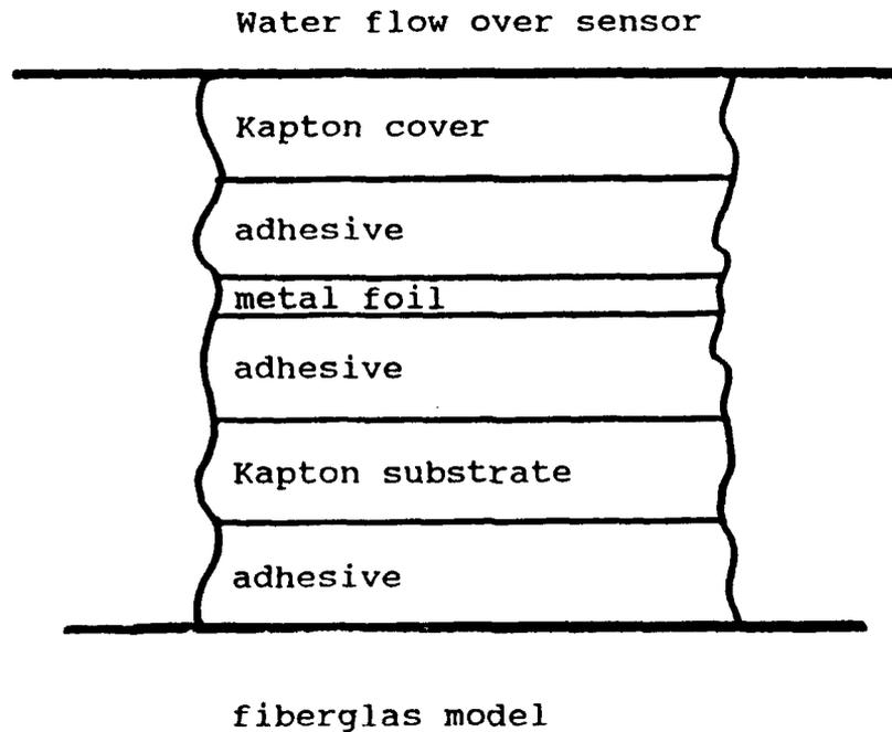
Figure 5. Schematic of the sensor cross-section.
