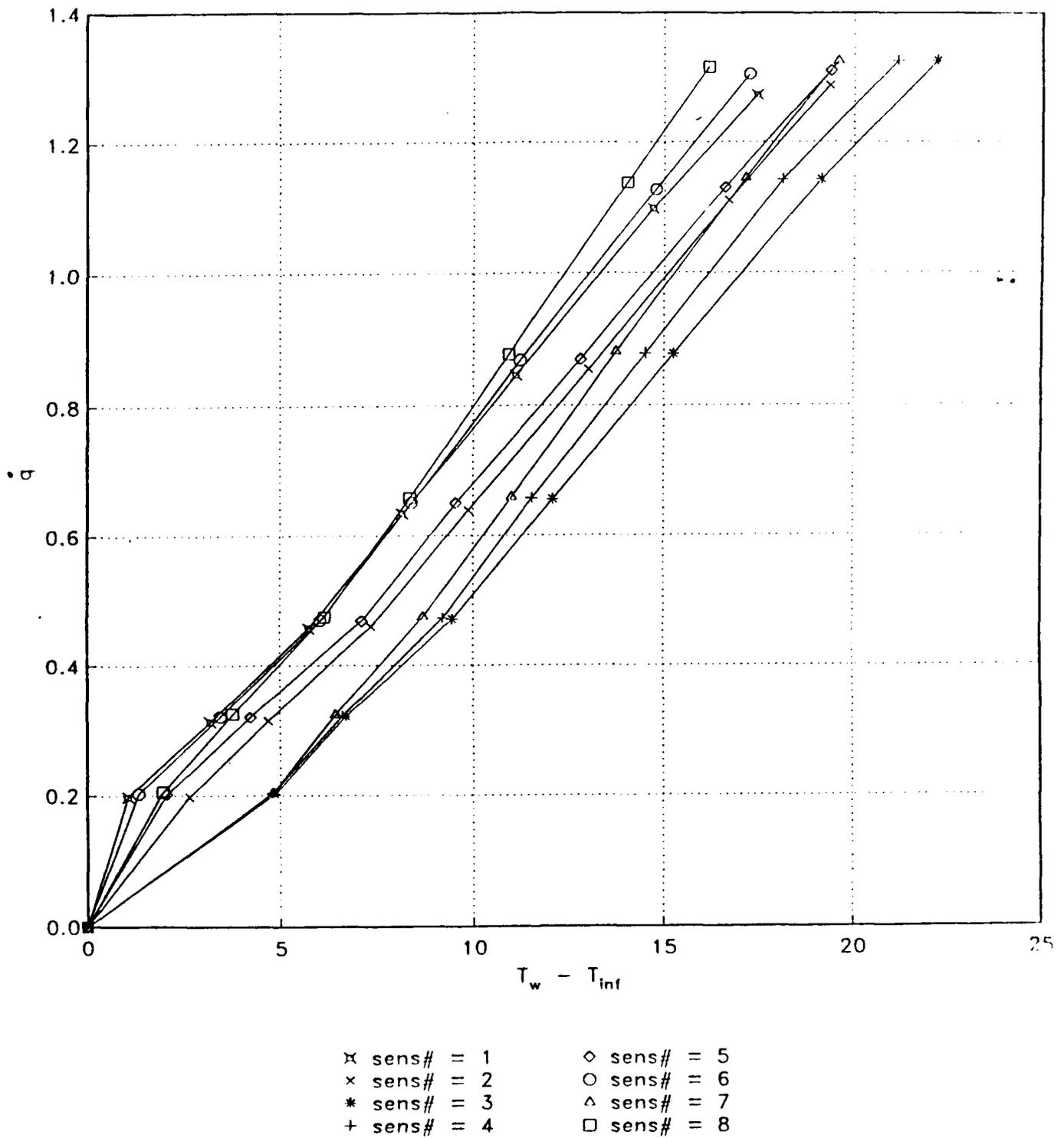
Figure 9. Experimental data for the circular cylinder at 22 degrees angle of attack. Measured heat transfer rate,  $\dot{q}$ , for each of 8 constant current anemometer sensors is plotted versus the sensor cover temperature difference,  $(T_w - T_{\infty})$ , for each of 8 different current settings.
