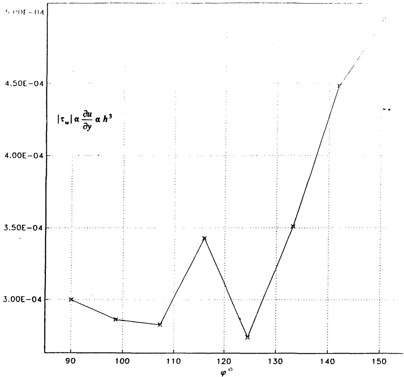
Figure 10. Experimental results of the relative magnitude of the surface shearing stress versus the peripheral angle. Note the location of a separation near  $105^\circ$ , a reattachment near  $115^\circ$ , and a second separation near  $125^\circ$ .
