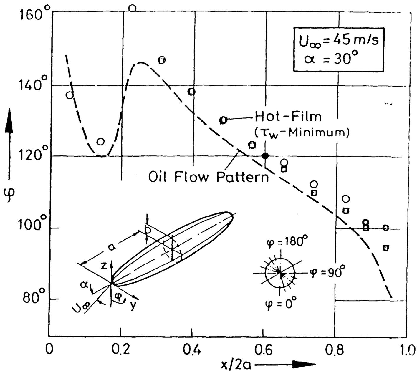
Figure A.2 Comparison of separation regions obtained from oil flow patterns and surface hot film measurements,  $\alpha = 30^\circ$  (Meier and Kreplin, 1980). Circles denote location of local minimum in skin friction magnitude. Squares denote separation locations calculated by equation (A.10) and the method shown schematically in Figure A.3.
