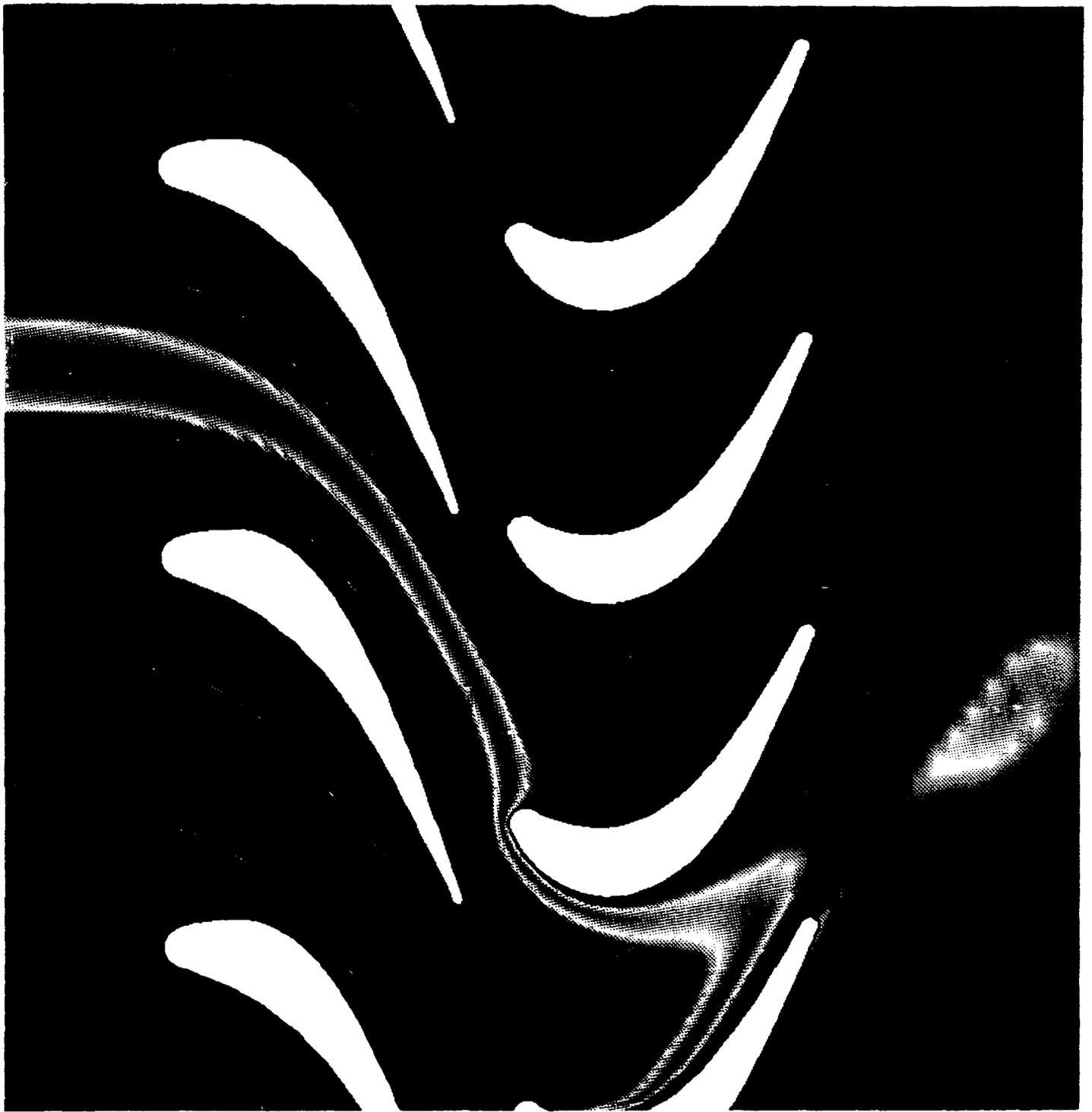
Figure 111: Static temperature contours for 3-stator/4-rotor LSRR simulation with a heat flux and film cooling
