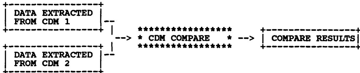
Figure 3-3 Compare Phase Block Diagram
