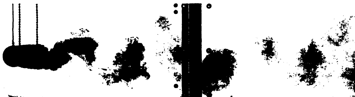
FIGURE 11. Natural (unforced) shedding. Flow visualized with dye issuing as for the data in figures 5, 7-10.
