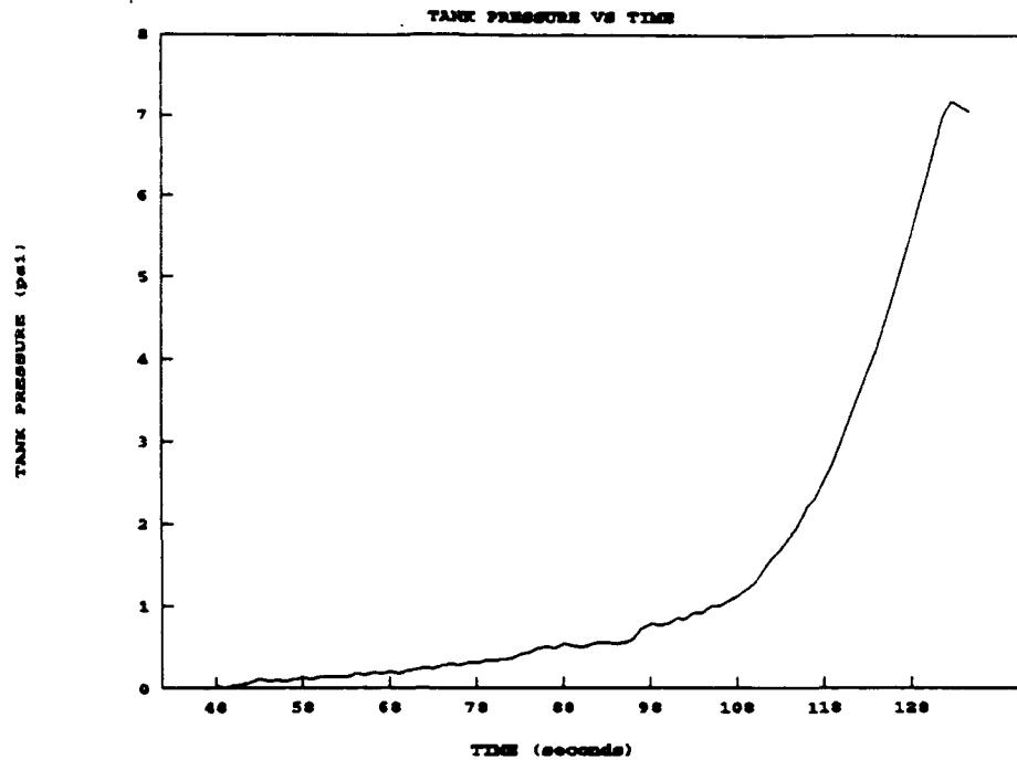
**Figure 13. Internal Tank Pressure During Fill Cycle 4**
