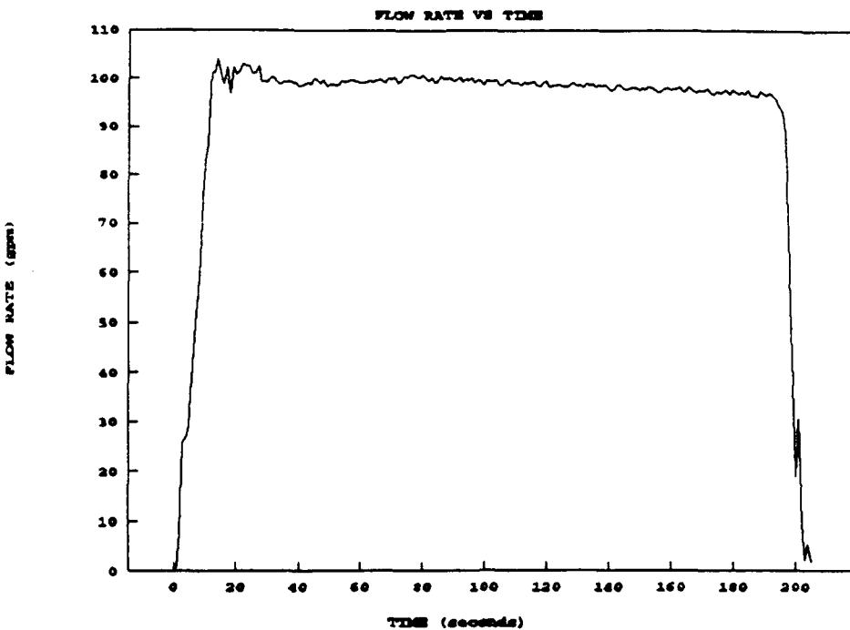
**Figure 14. Defuel Rates for Carter Refuel/Defuel Valves**
