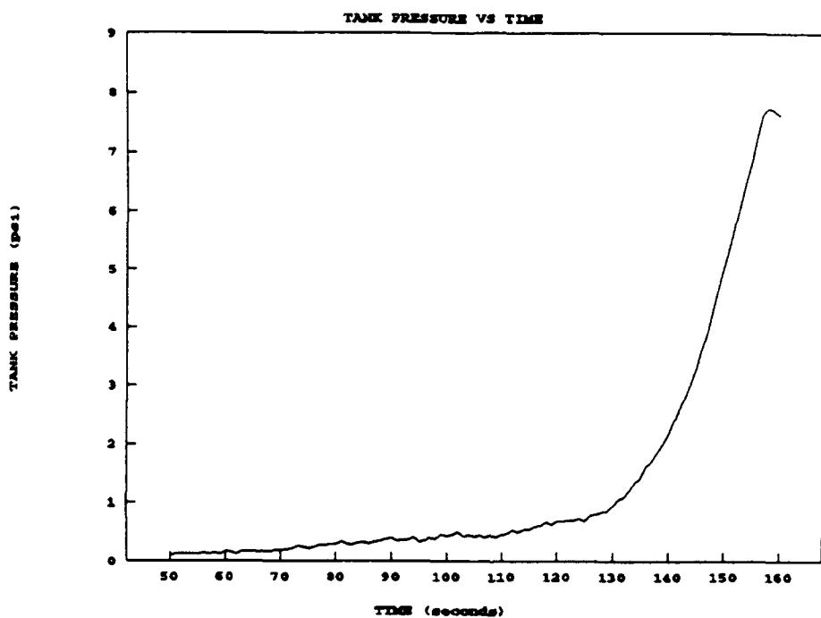
**Figure 12. Internal Tank Pressure During Fill Cycle 3**
