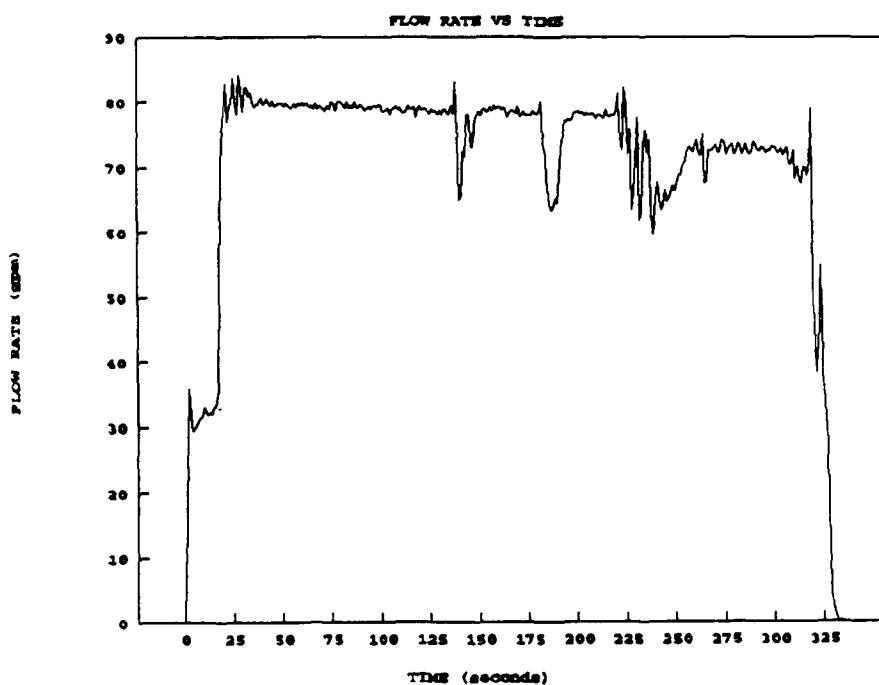
Figure 8. Defuel Rate for Existing Poppet Valve
