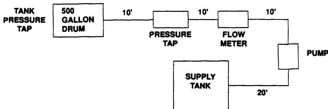
**DEFUEL TEST SET-UP**
