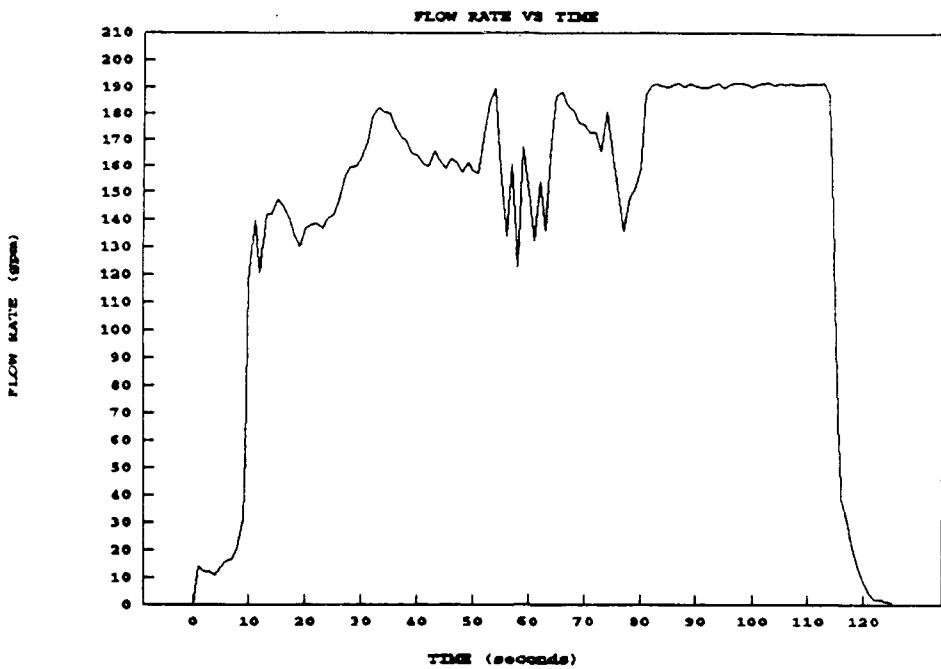
**Figure 19. Defueling Rates for 3-inch Kamvalok**
