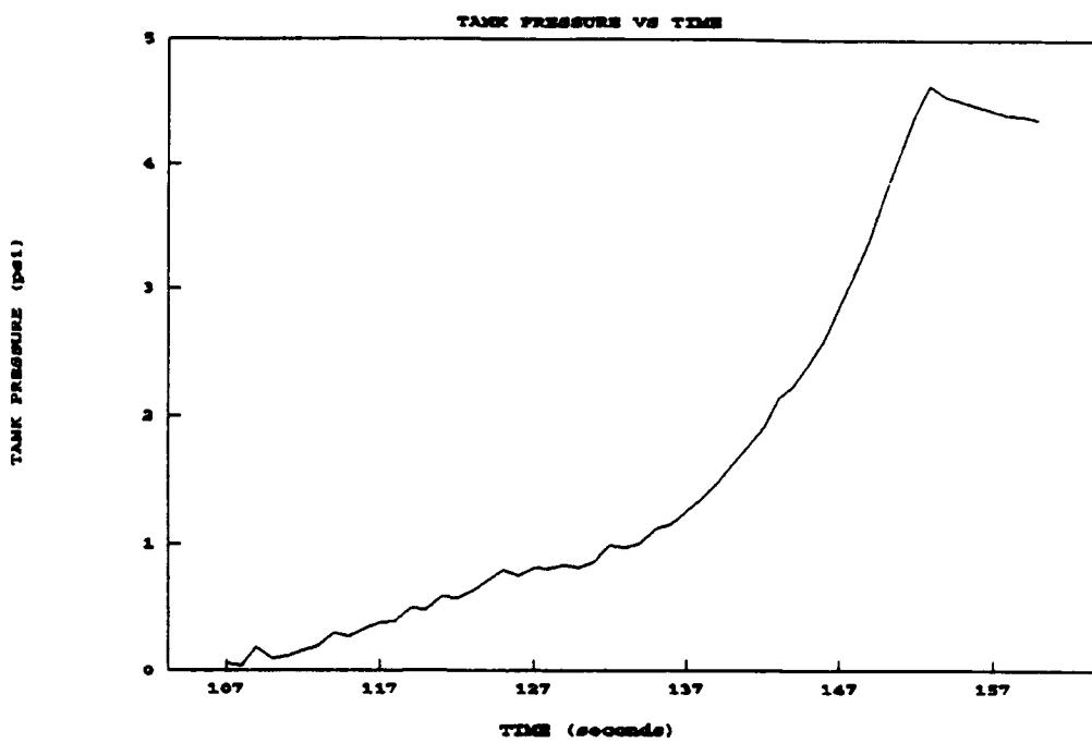
**Figure 10. Internal Tank Pressure During Fill Cycle 1**
