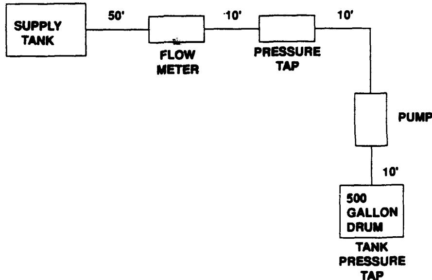
**Figure 6. Hardware Setup for Poppet Valve Testing**
