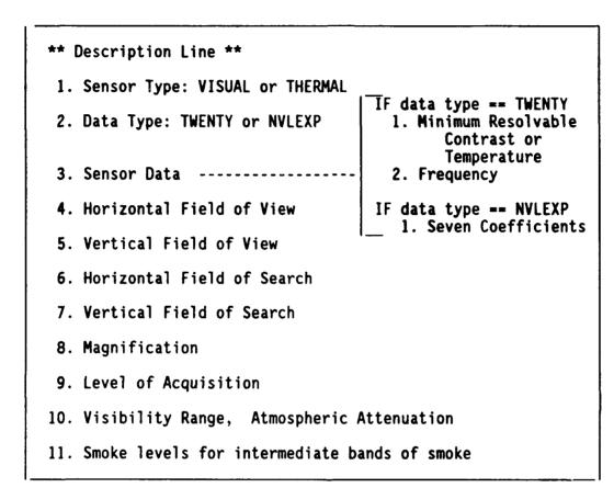
Figure II.E.1 Optical or Thermal Sensor Data.
