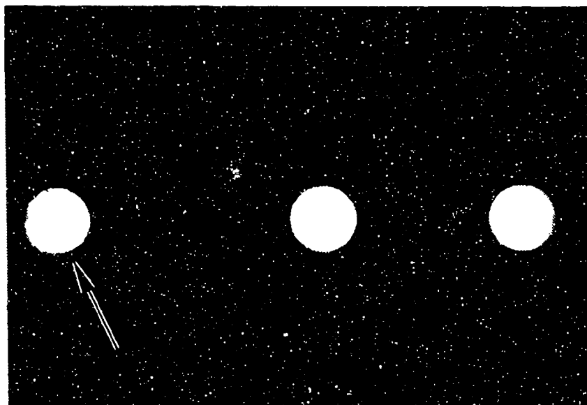
Figure 2-16. Rockwell Flaw Criticality Study Defect 18: Mislocated Hole — Not Repaired
