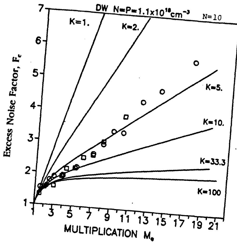
Figure 1. Excess noise factor,  $F_e$ , vs. gain,  $M_e$  for doped quantum well APD.
