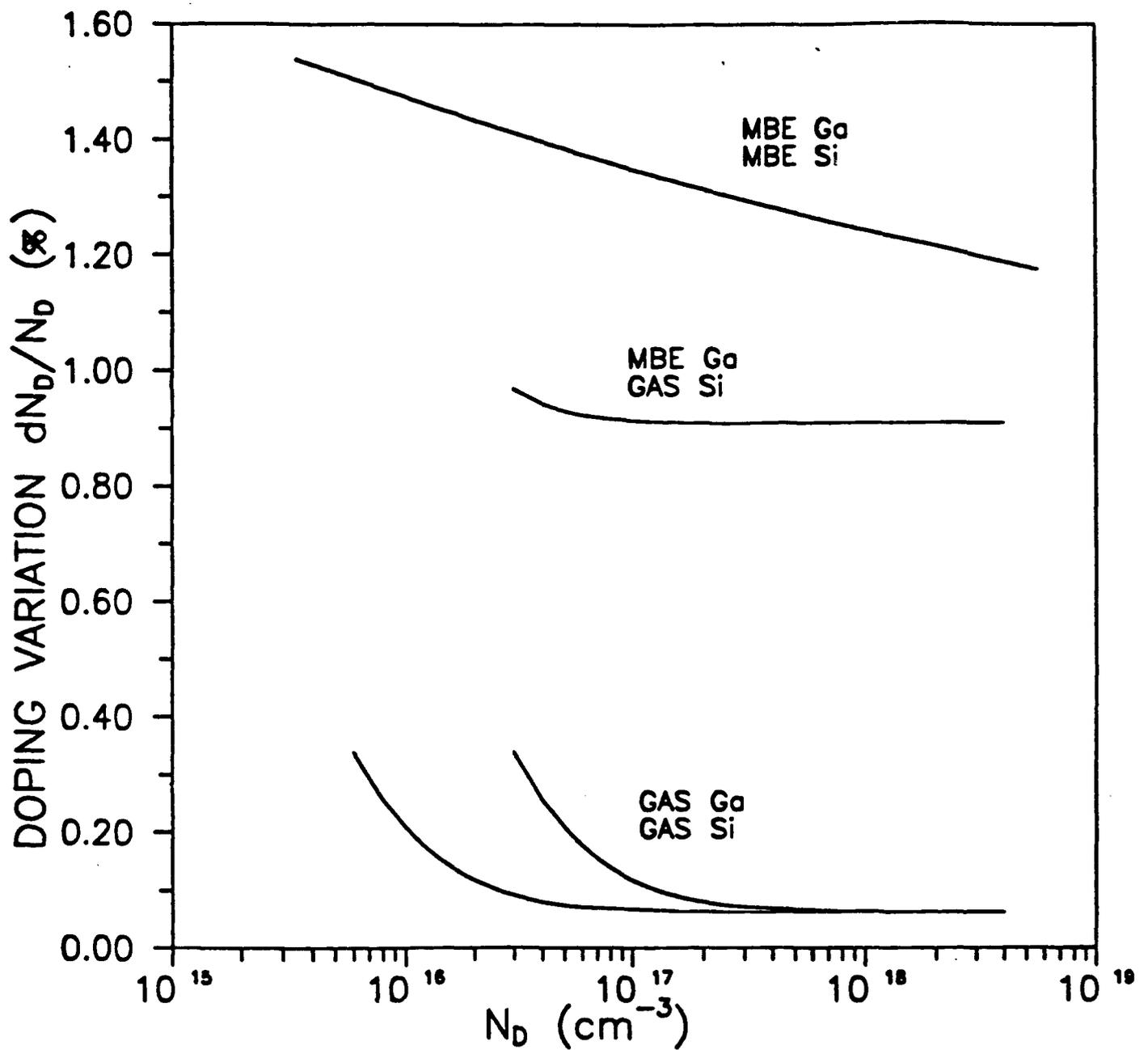
Figure 2. Doping variation vs. doping concentration for Si doped GaAs using conventional MBE thermal sources, gas source doping and CBE growth.
