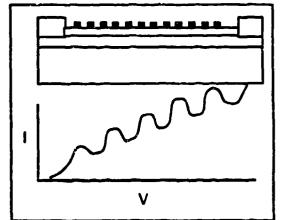
Interference effects observed correspond closely to those expected based on prior knowledge of these devices. Multiple extrema in the current-voltage relationships suggest the possibility of multi-level logical elements, now that such devices can be fabricated and effectively characterized. Further variations involving such devices
