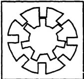
A recent meeting of the Materials Research Society included mention of a new and novel motor drive for micromachines. A ferroelectric lead zirconate-titanate film on silicon over a diaphragm is used to drive a traveling surface flexure wave which, through friction contact with a micro-gear, drives the gear<sup>28</sup>. This micromotor is reportedly about 1 mm in diameter, and has the advantage of providing significant force as a driver for micro-robots
