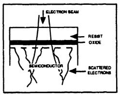
direct write and mask making e-beam lithography as it can be used on bulk substrates.
