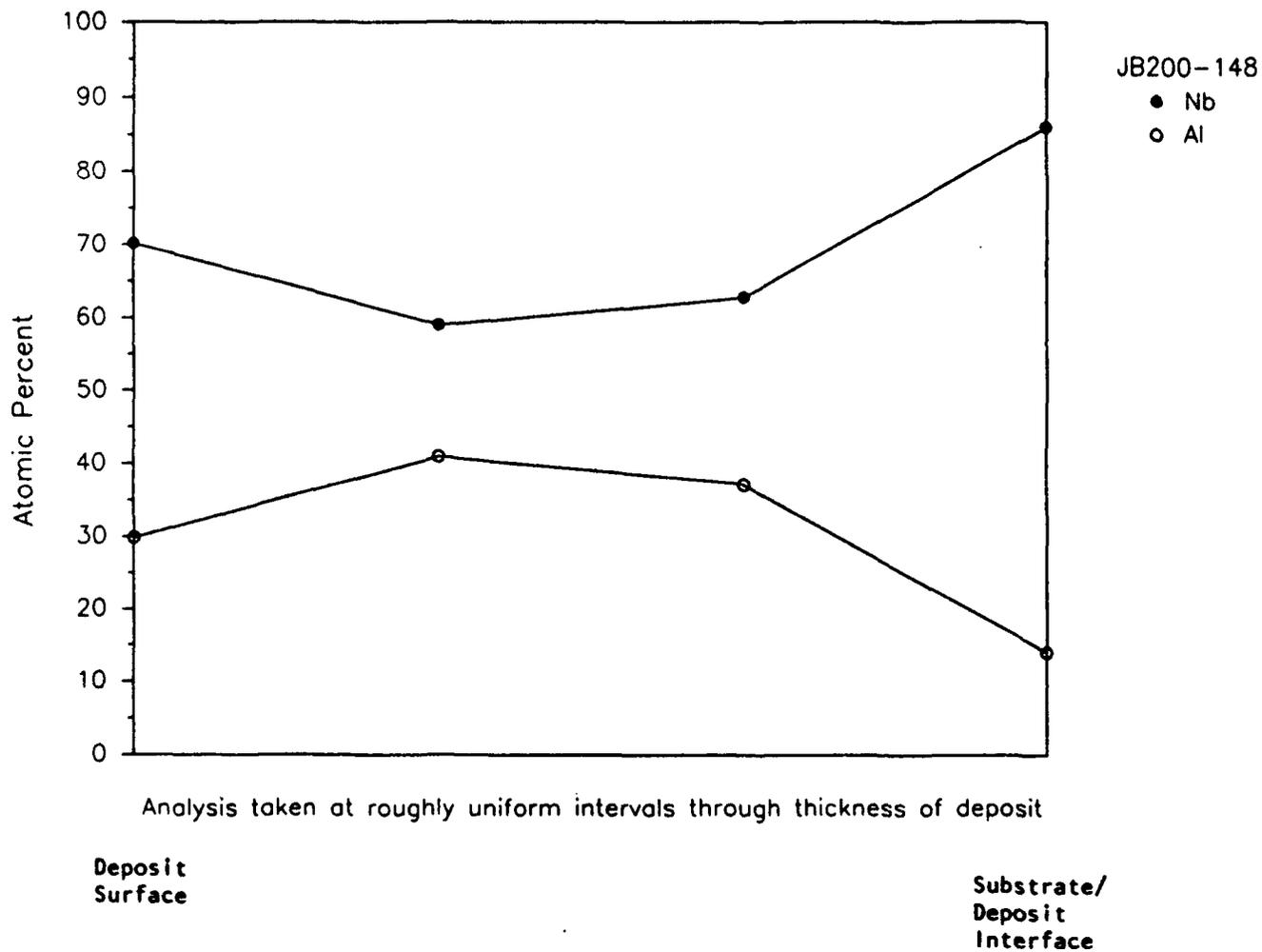
Figure 4-27. Niobium and aluminum contents of deposit JB200-148 taken from the substrate surface to the deposit surface.
