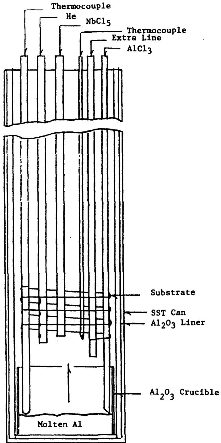
Figure 5-3. Schematic diagram of the experimental setup used for vapor infiltration of alumina tow.
