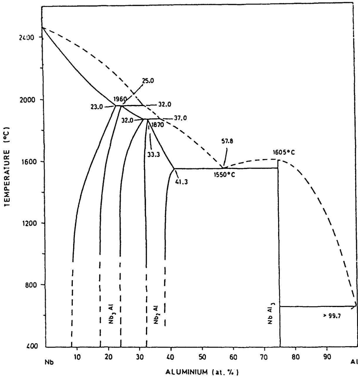
Figure 3-1. Phase diagram of the Nb-Al system.
