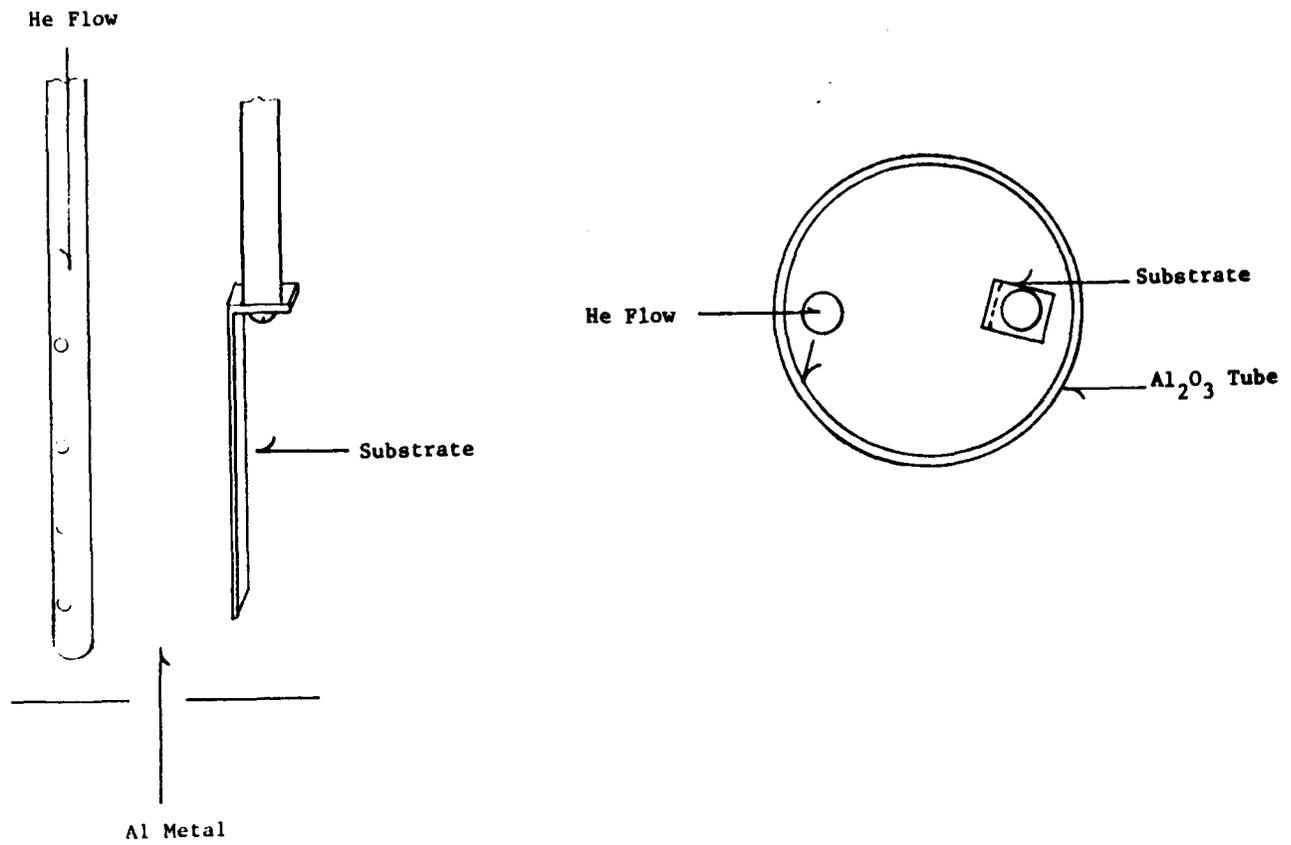
Figure 4-16. Schematic diagram of the added helium gas injection system, directed at right angles to the substrate, showing its relationship to the deposition chamber.
