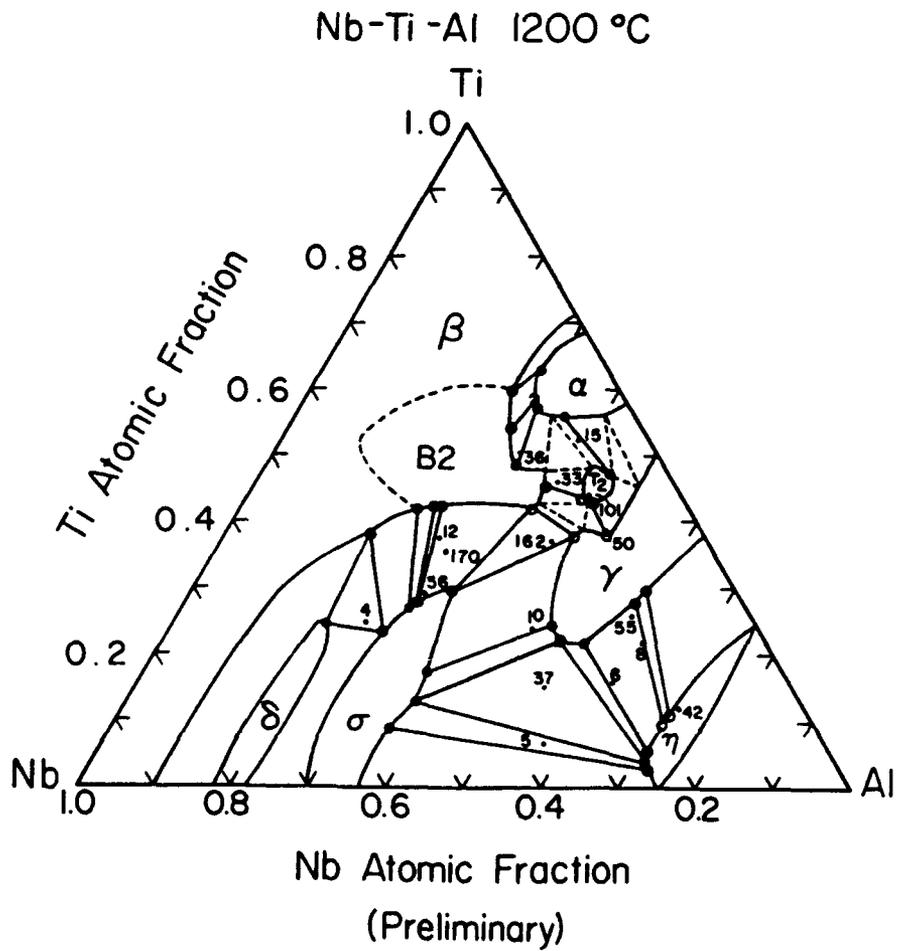
Figure 4-42. The 1200°C section of the Nb-Ti-Al system phase diagram (Ref. 4-1).
