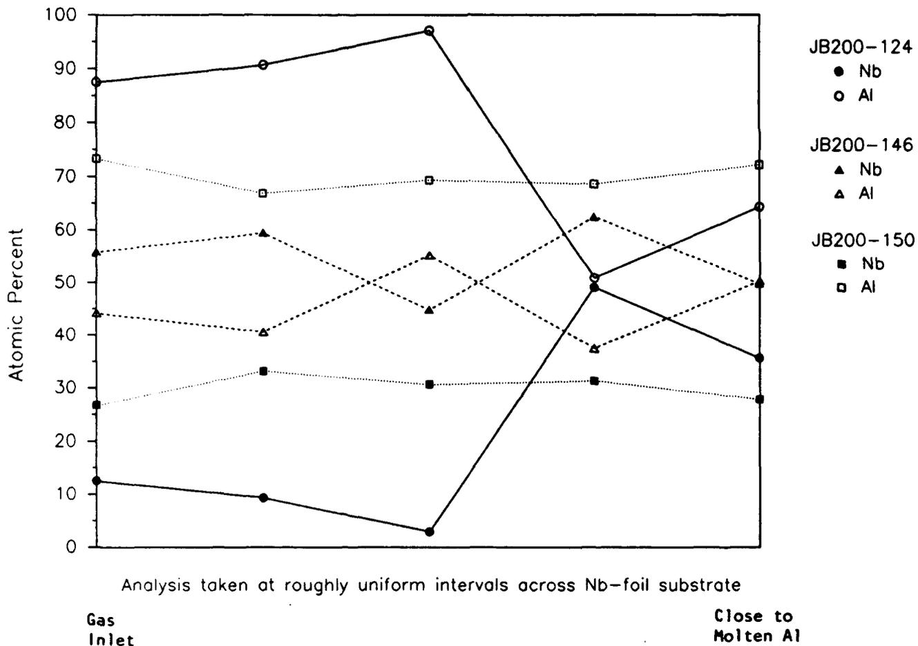
Figure 4-26. Niobium and aluminum contents, end to end, of deposits formed (1) without auxiliary helium in the reactive gas (sample JB200-124), (2) with auxiliary helium directed at the molten aluminum (sample JB200-146), and (3) with auxiliary helium parallel to the substrate (sample JB200-150).
