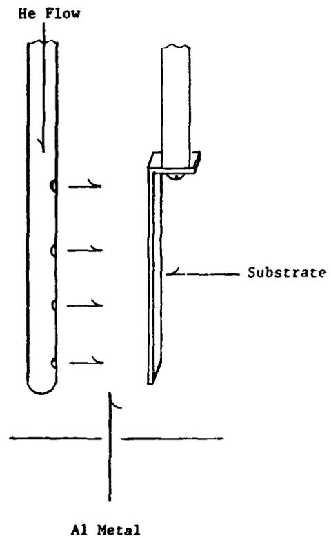
Figure 4-15. Schematic diagram of the inert gas injection system showing the added helium inlets directed at the molten aluminum or at the substrate.
