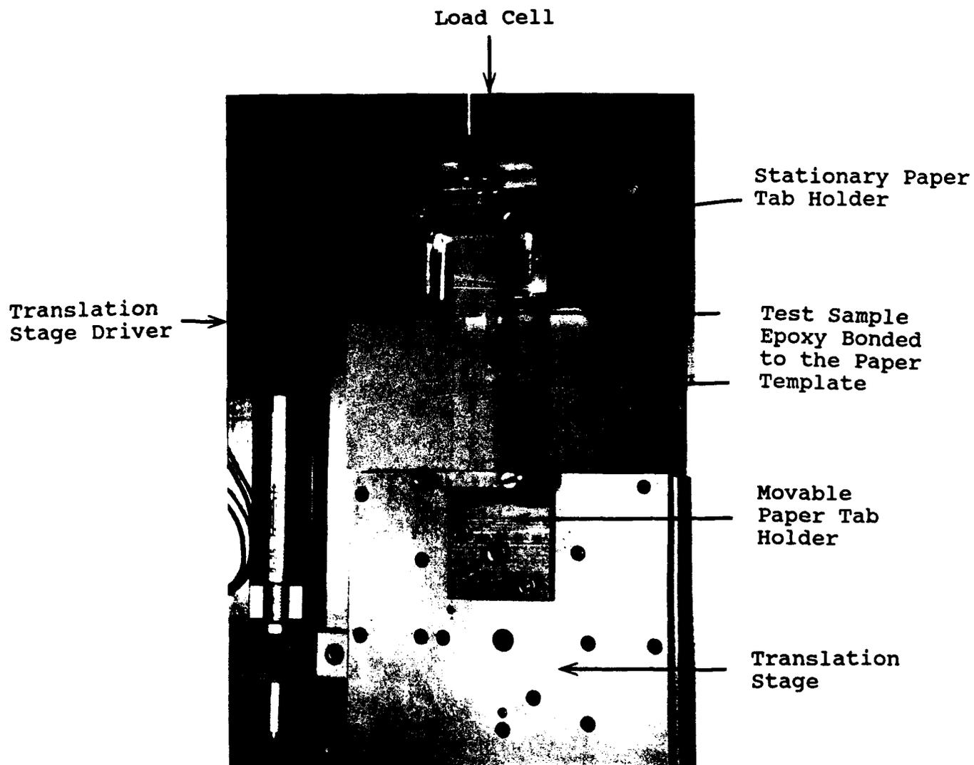
Figure 6-3. Test sample epoxy bonded to a paper template and mounted in the test fixture.
