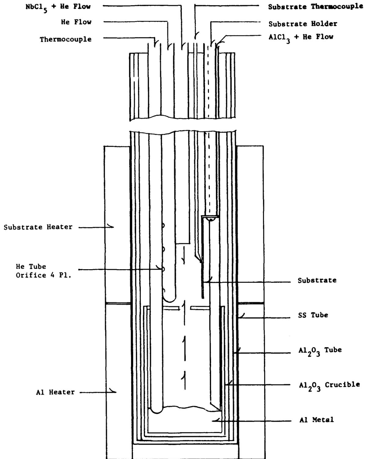
Figure 4-14. Schematic diagram of the molten aluminum system deposition chamber with a tube furnace heated substrate.
