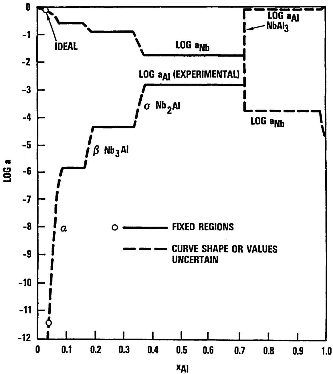
Figure 3-2. Al-Nb activity diagram according to Malets' data (900 K).
