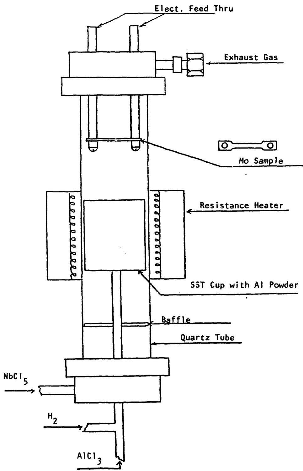
Figure 4-28. Schematic diagram of the resistance heated reactor used for  $NbAl_x$  deposition from  $NbCl_5 + AlCl_3 + H_2$ .
