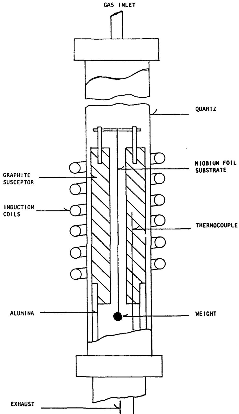
Figure 4-30. Schematic diagram of the isothermal CVD deposition system used for the formation of  $Nb_xAl_y$  by the hydrogen reduction of the halides.
