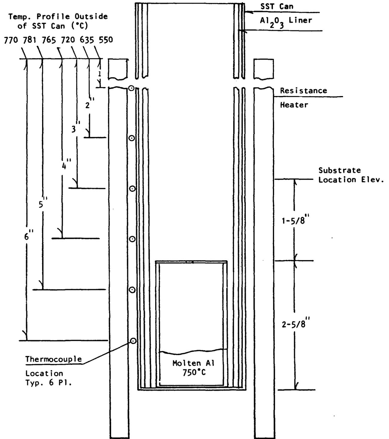
Figure 4-3. Typical temperature distribution in the molten aluminum system deposition chamber.
