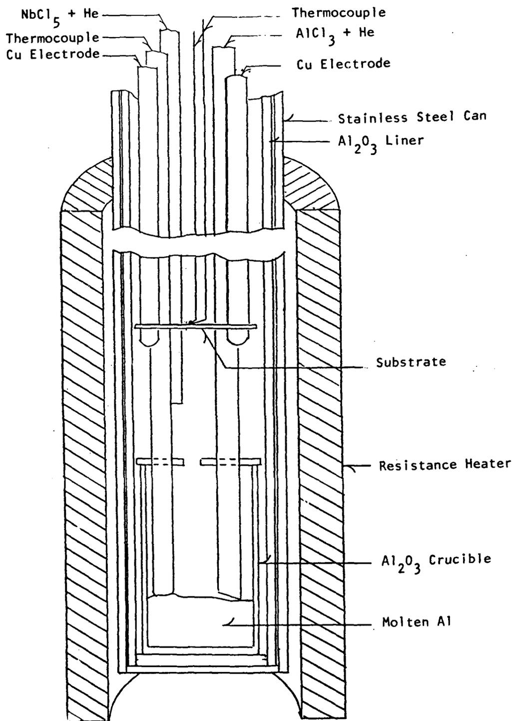
Figure 4-1. Schematic diagram of the molten aluminum system chamber.
