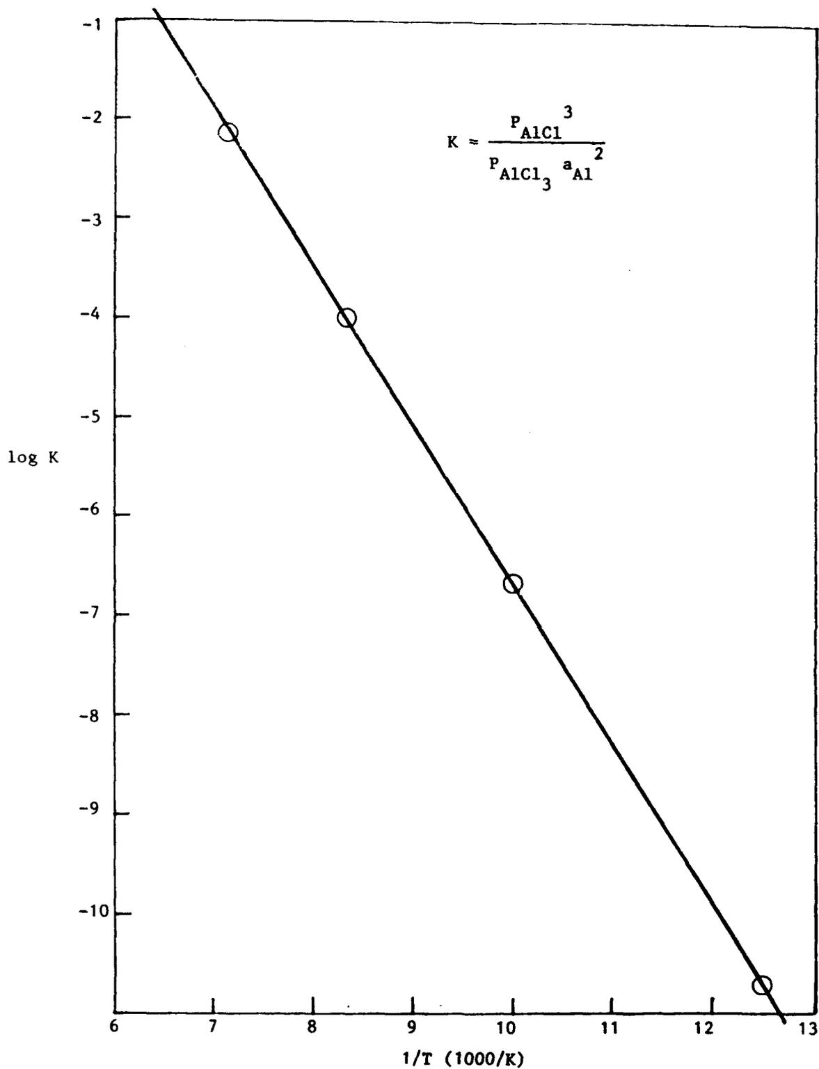
Figure 3-3. Equilibrium constant for  $\text{AlCl}(\text{g})$  formation from  $\text{Al}(\text{l}) + \text{AlCl}_3(\text{g})$ .
