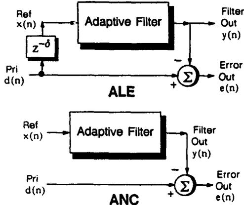
Figure 3: Adaptive Line Enhancer (ALE) and Adaptive Noise Canceller (ANC) Filters.
