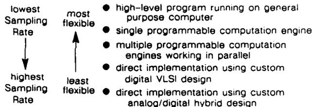
Figure 1: Adaptive Filter Implementation Methods and their Tradeoffs.
