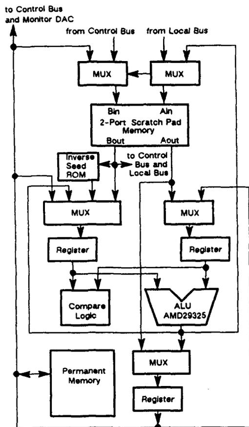
Figure 7: The Computation Engine's Microengine Data Path.
