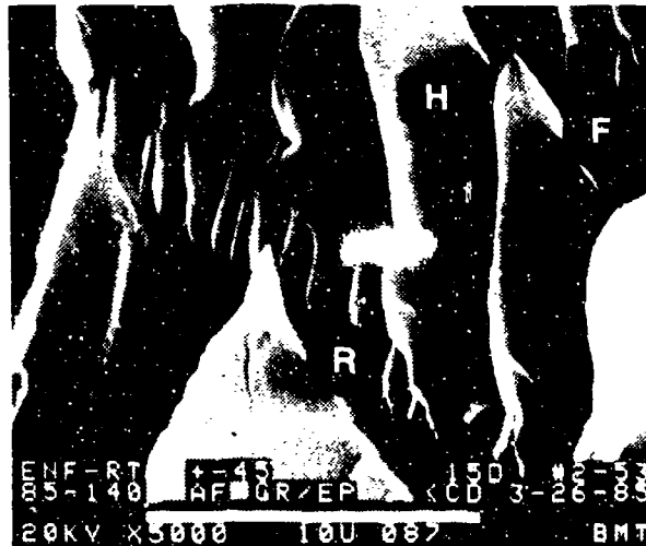
Figure 2-67. SEM Photographs of Interlaminar Mode II Shear, +45/-45 Fracture, 70 F/Dry
