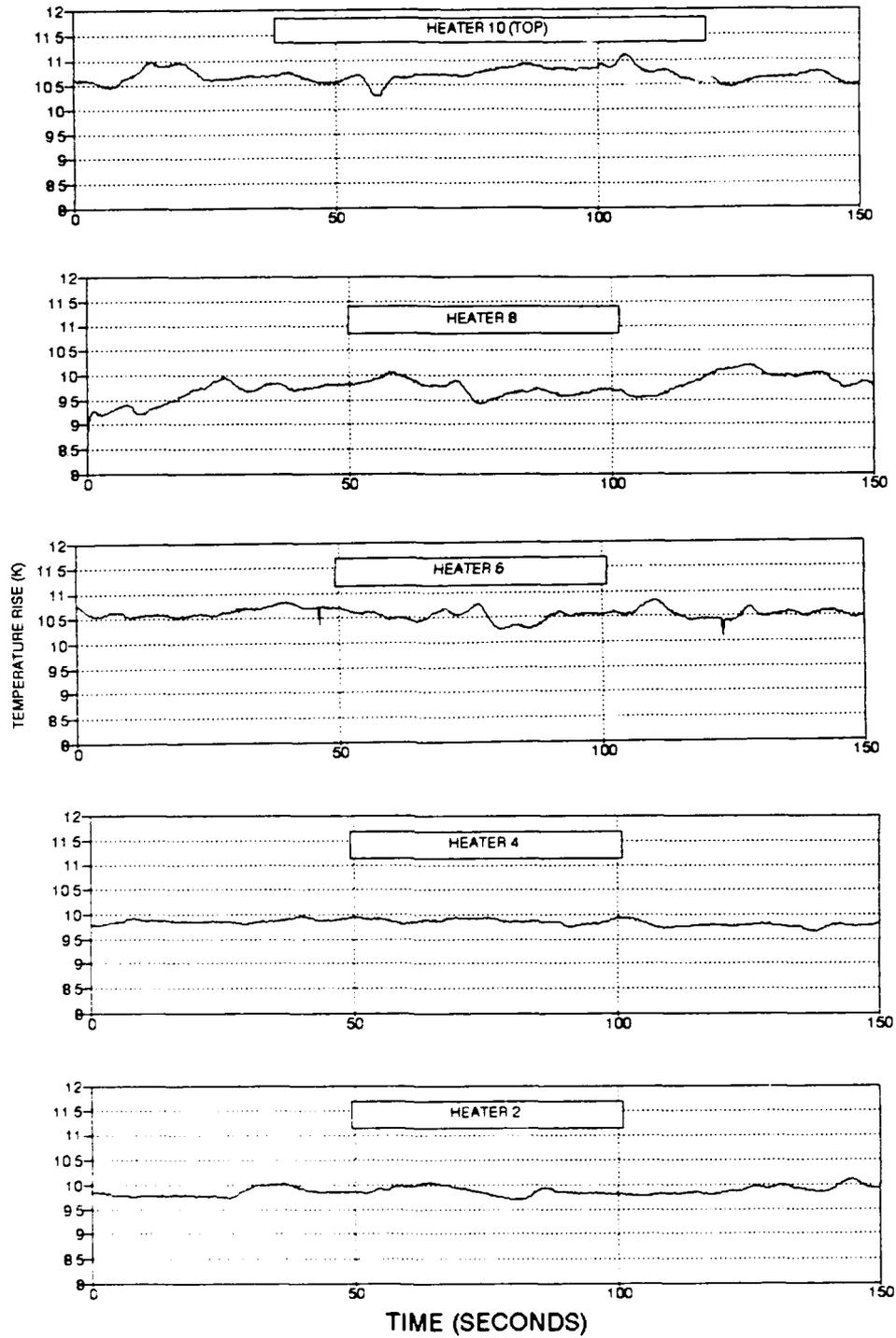
Figure 17. Temperature Rise versus Time. Heat flux=  $2510\text{W}/\text{m}^2$  ;  $\text{Re}=1000$ .
