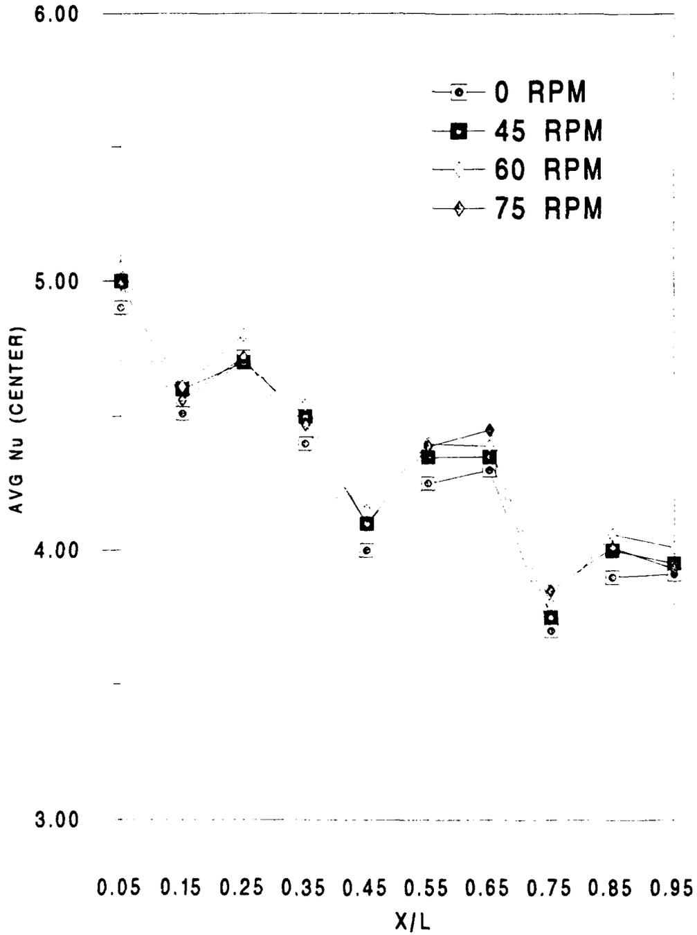
Figure 8. Average Nusselt number versus X/L. Heat flux=505 W/m<sup>2</sup> ; Re=3000.
