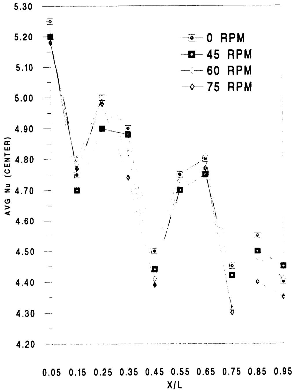
Figure 9. Average Nusselt number versus X/L. Heat flux=505 W/m<sup>2</sup> ; Re=5000.
