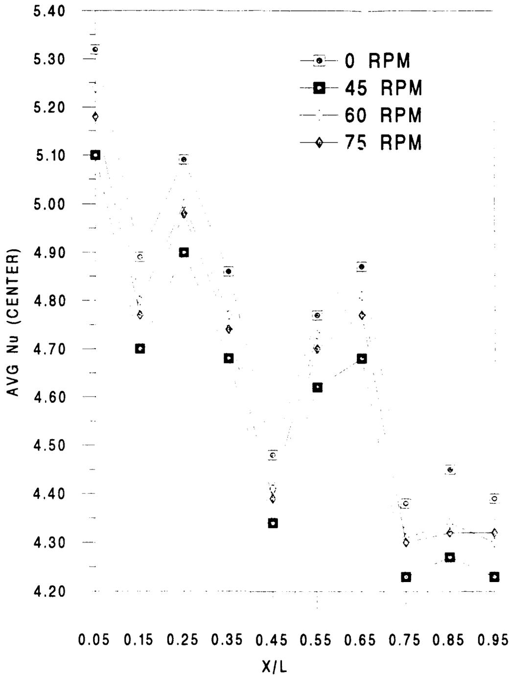
Figure 14. Average Nusselt number versus X/L. Heat flux = 1050 W/m<sup>2</sup> ; Re=5000.
