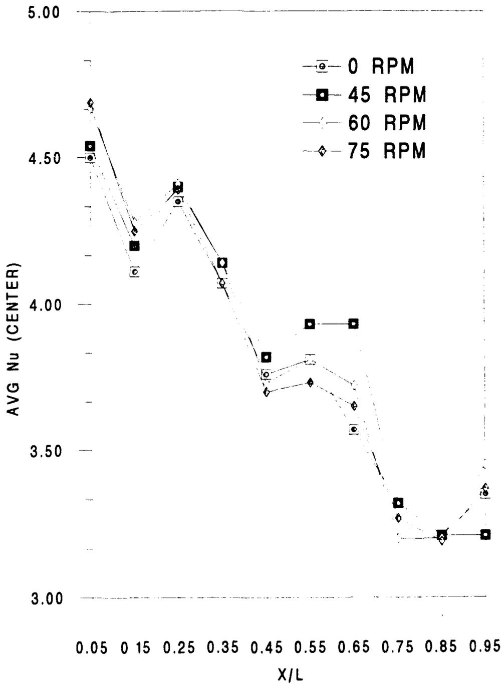
Figure 12. Average Nusselt number versus X/L. Heat flux=
