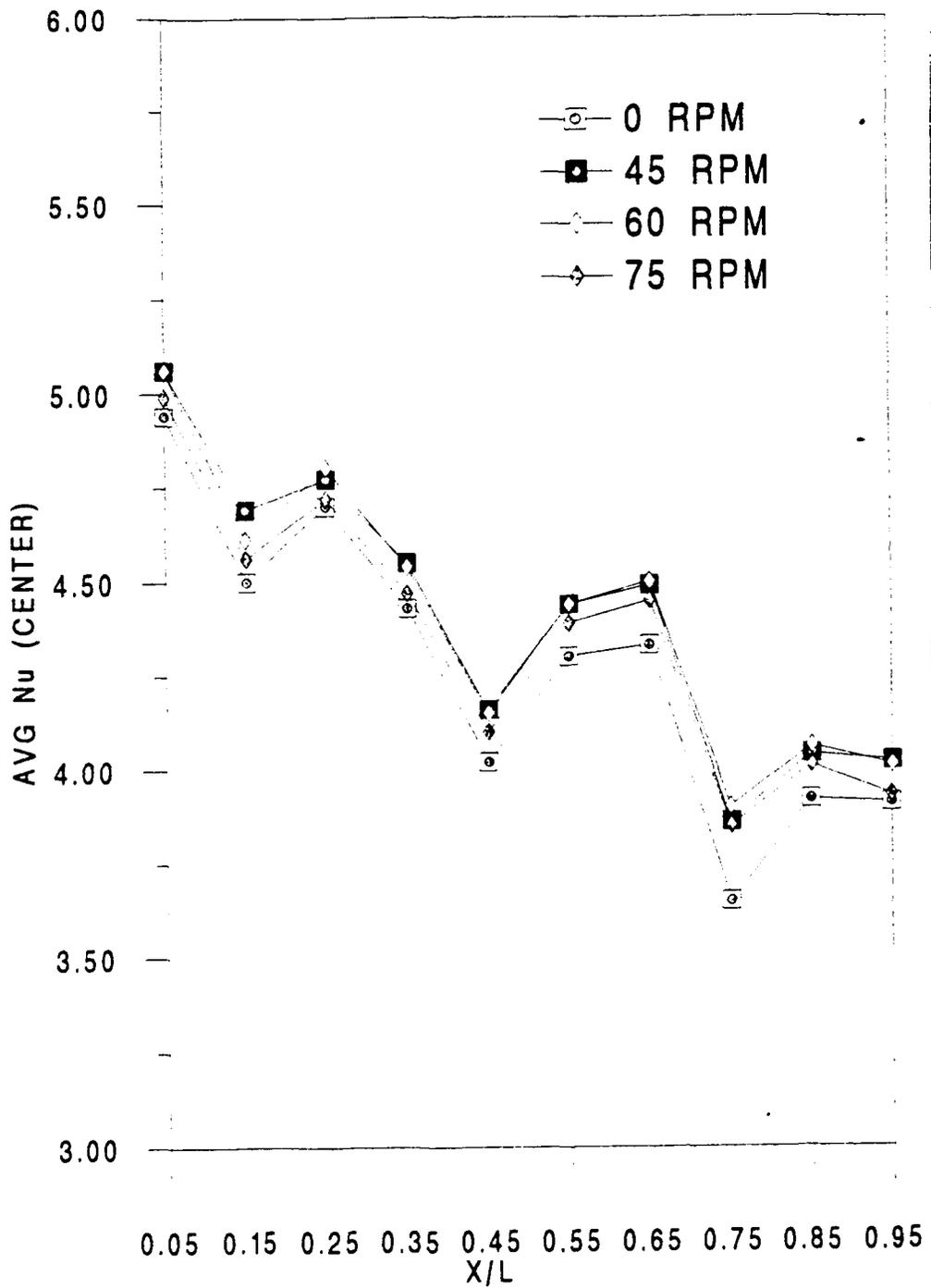
Figure 13. Average Nusselt number versus X/L. Heat flux= 1050 W/m<sup>2</sup> ; Re=3000.
