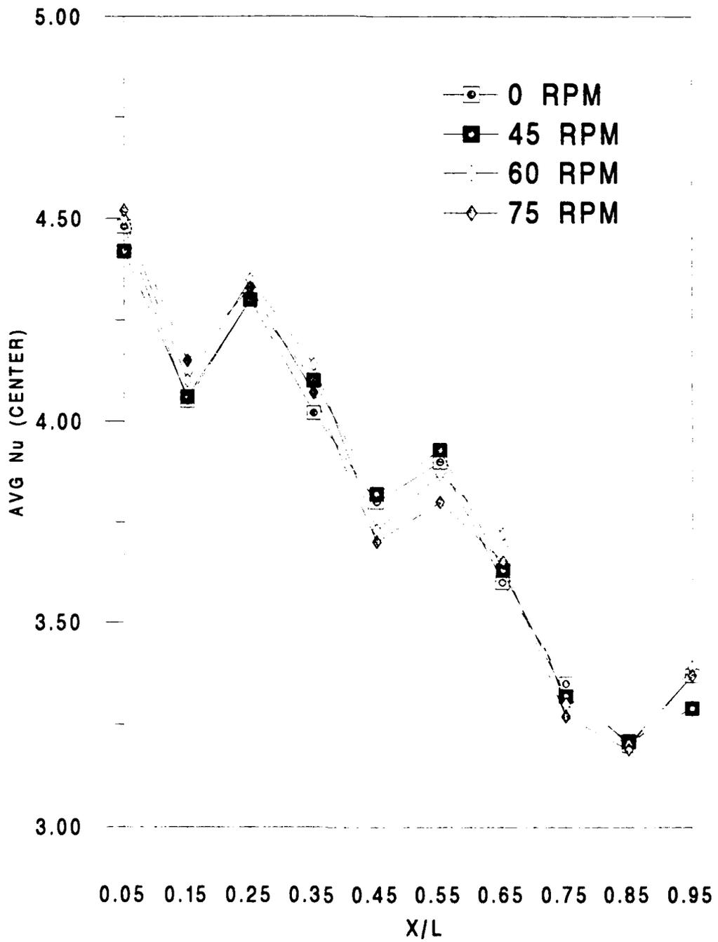
Figure 7. Average Nusselt number versus X/L. Heat flux =505 W/m<sup>2</sup> ; Re=2000.
