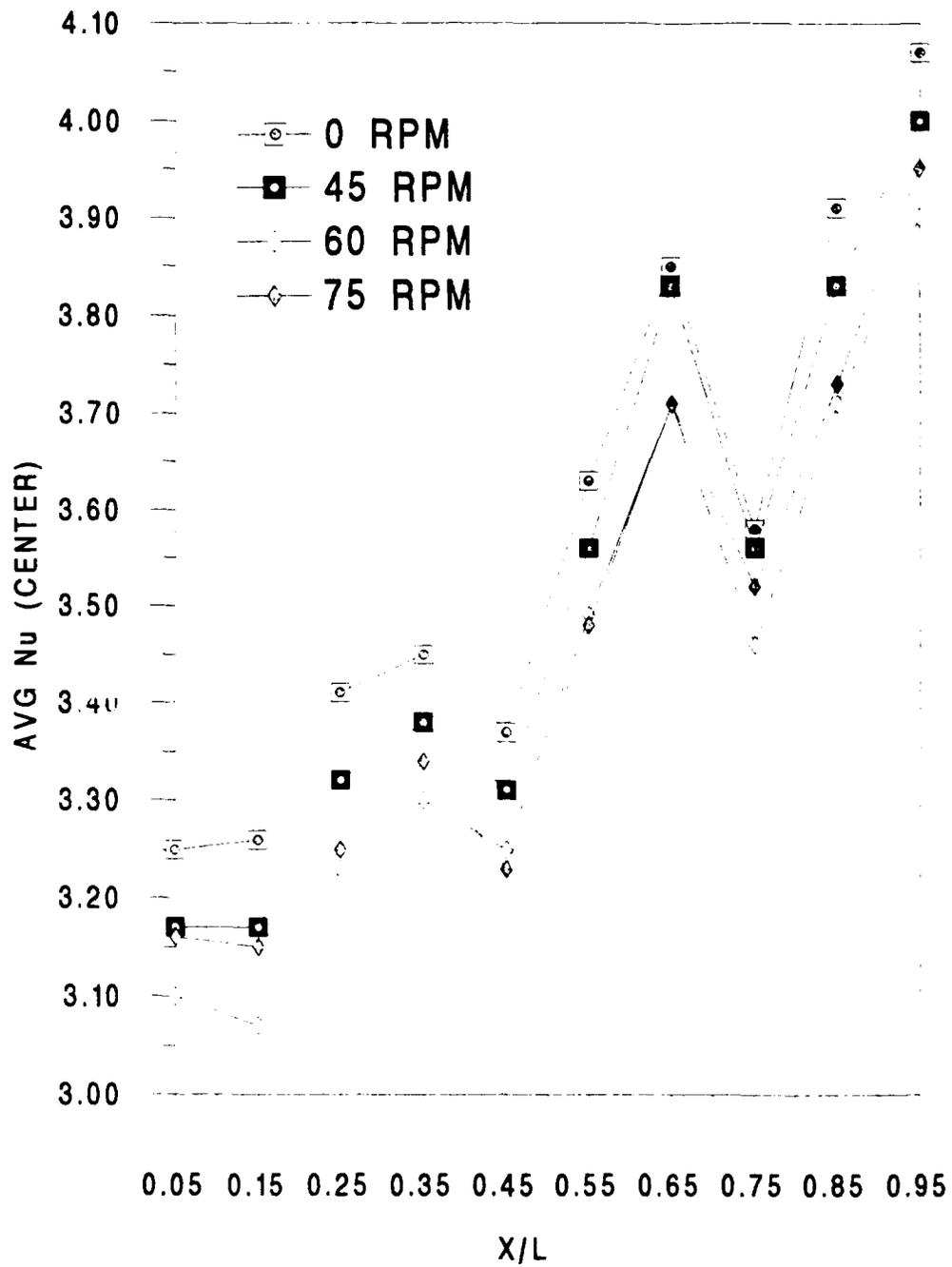
Figure 11. Average Nusselt number versus X/L. Heat flux=
