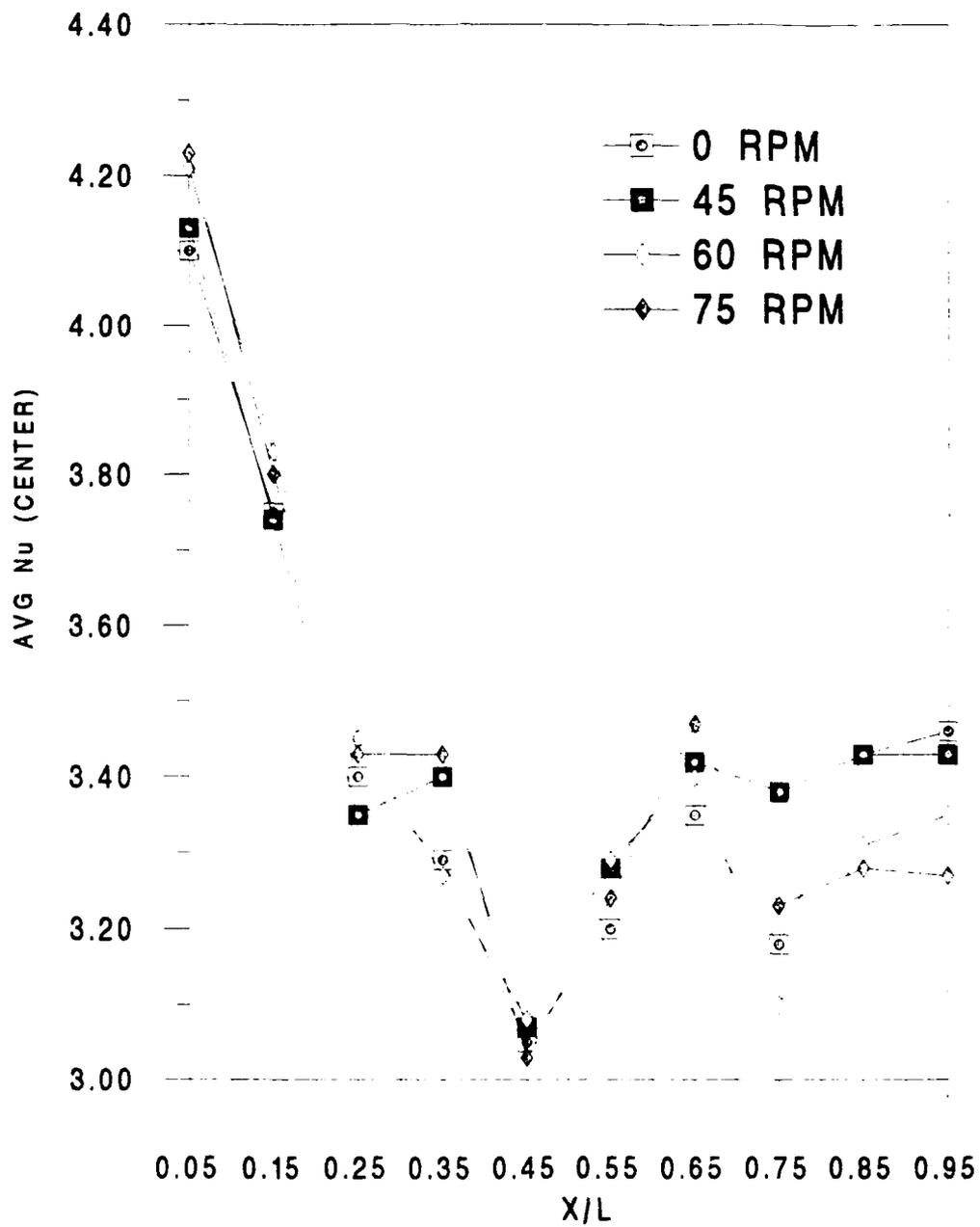
Figure 15. Average Nusselt number versus X/L. Heat flux =  $1600 \text{ W/m}^2$  ;  $\text{Re}=2000$ .
