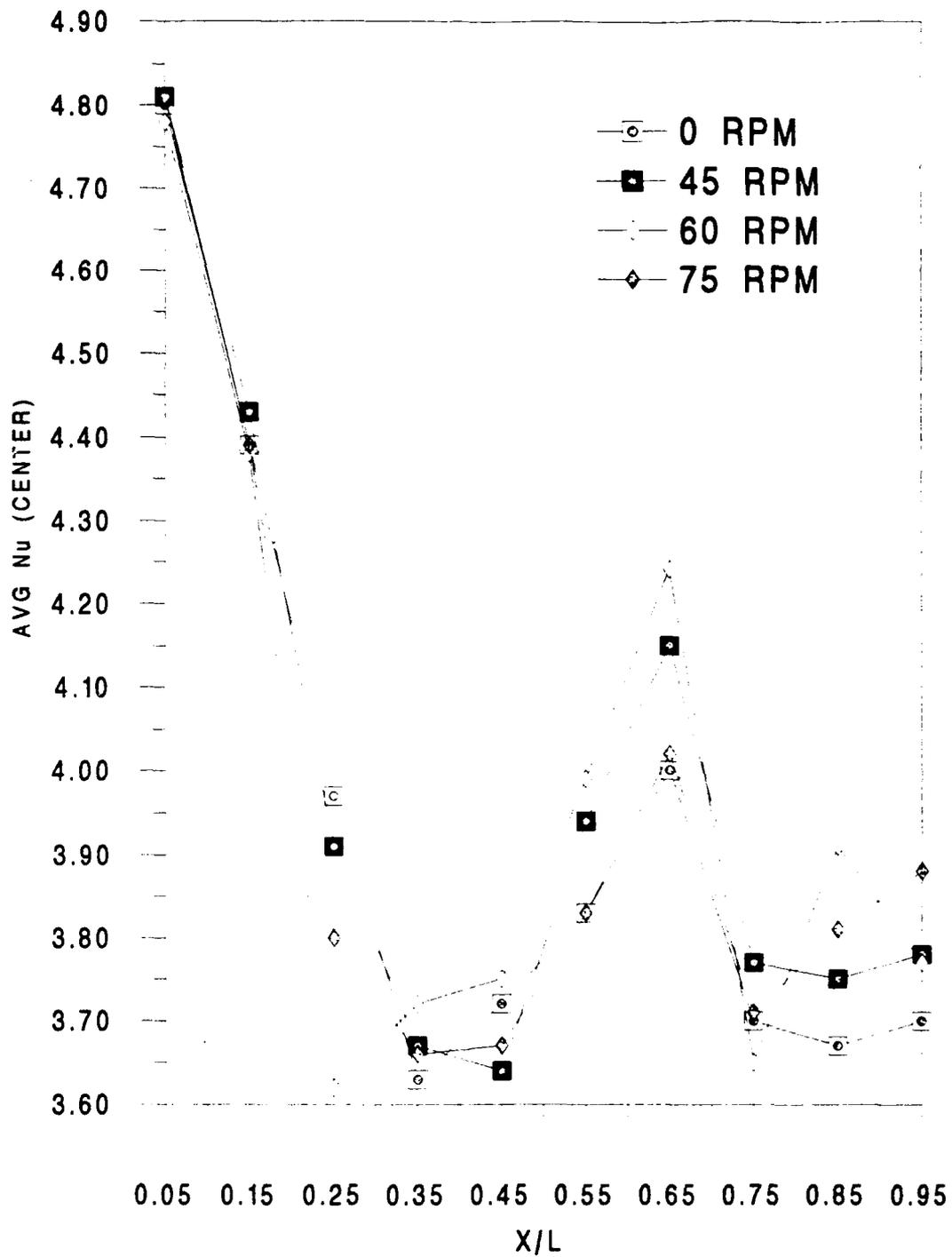
Figure 16. Average Nusselt number versus X/L. Heat flux=
