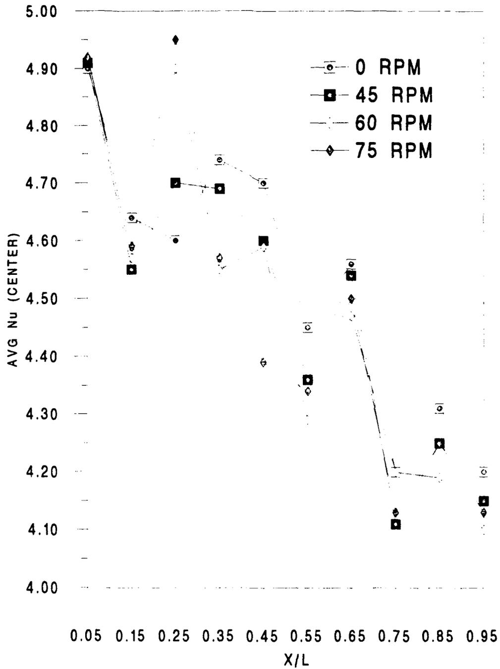
Figure 10. Average Nusselt number versus X/L. Heat flux=505 W/m<sup>2</sup> ; Re=8000
