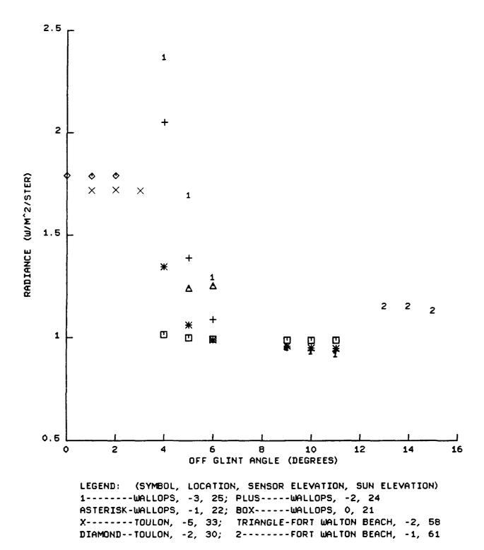
FIGURE 3. AVERAGE RADIANCE VERSUS GLINT ANGLE FOR HORIZONTAL SCANS
