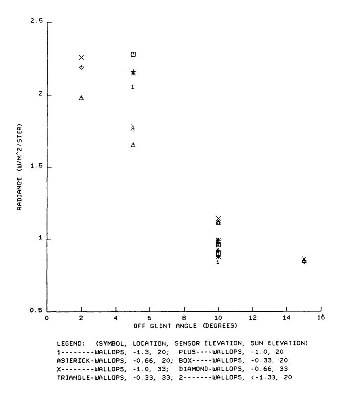
FIGURE 4. AVERAGE RADIANCE VERSUS GLINT ANGLE FOR VERTICAL SCANS
