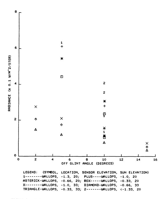
FIGURE 6. STANDARD DEVIATION RADIANCE VERSUS GLINT ANGLE FOR VERTICAL SCANS
