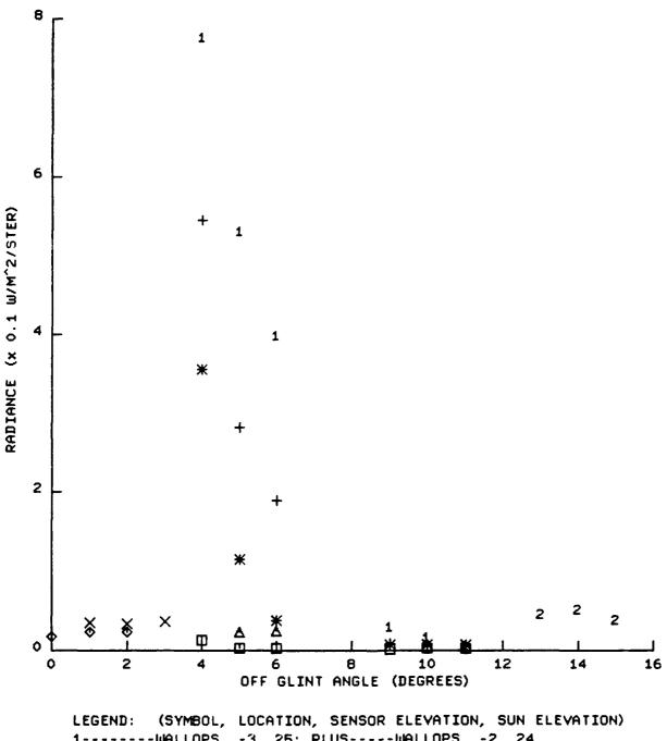
FIGURE 5. STANDARD DEVIATION RADIANCE VERSUS GLINT ANGLE FOR HORIZONTAL SCANS
