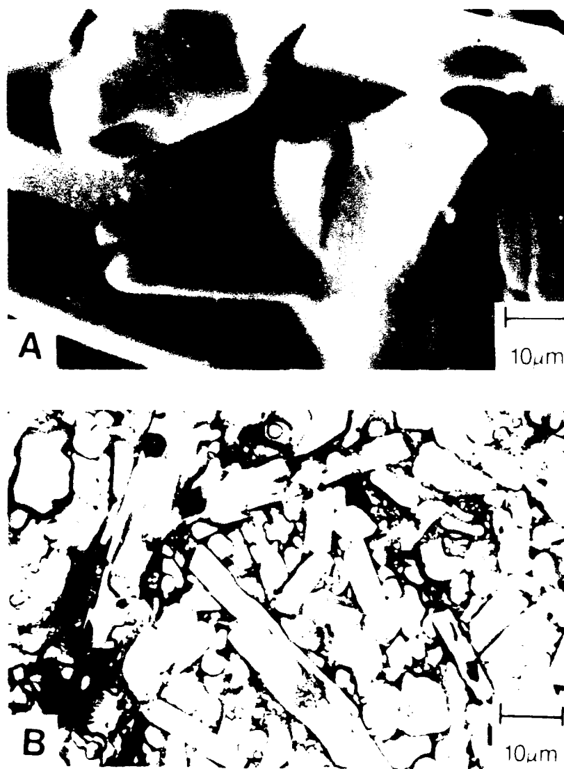
Figure 1. Morphology of sintered \text{YBa}_2\text{Cu}_3\text{O}_{6+x} superconducting ceramic material. (A) Secondary and (B) back scattered electron image.
