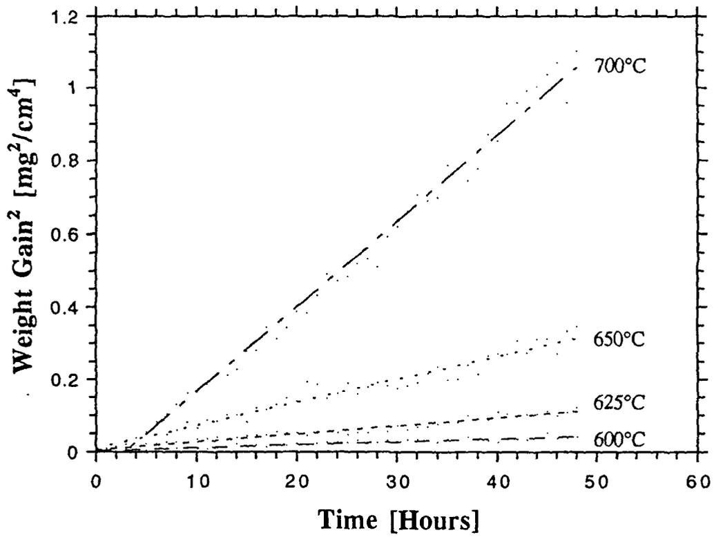
Figure 10. TGA results of Ti-23Nb-11Al oxidized in air for 48 hours between 600°C and 700°C. Note curve is plotted in parabolic coordinates; i.e. weight gain<sup>2</sup> vs. time.
