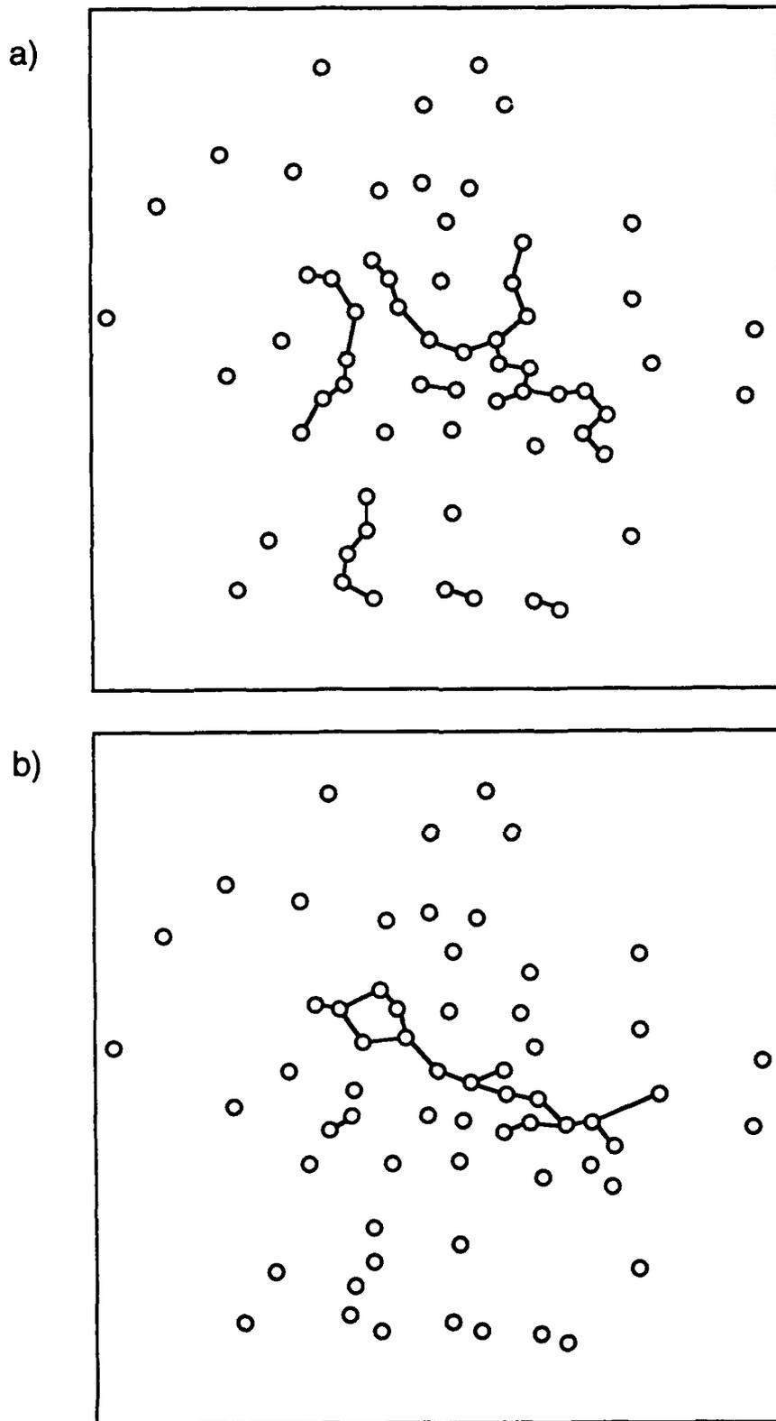
**Figure 1:** Schematic diagram of the localization paths developed in specimens with a minimum allowable hole spacing of 1.6 mm tested in either a) equal-biaxial tension or b) uniaxial tension. The tensile axis is vertical for the uniaxial case.
