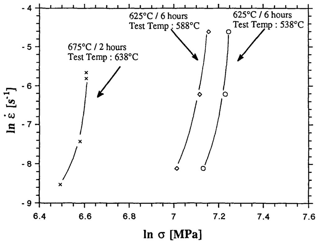
Figure 9. Summary of initial elevated compression tests. Illustrated are results from a sample in the 675°C / 2 hours condition, and two in the 625°C / 6 hours condition tested at 638°C, 588°C and 538°C, respectively.
