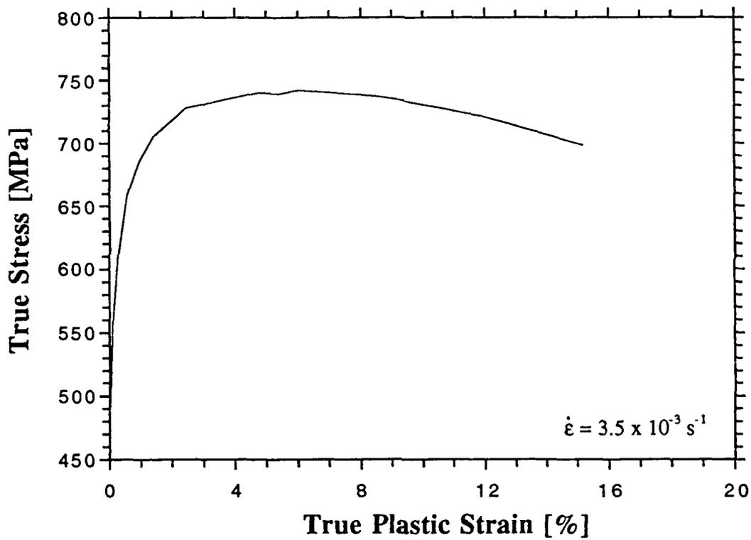
Figure 8. True stress-true strain response of the Ti-23Nb-11Al alloy tested in the 675°C / 2 hours condition. Deformation was in slow strain rate compression ( $3.5 \times 10^{-3} \text{ s}^{-1}$ ) at 638°C.
