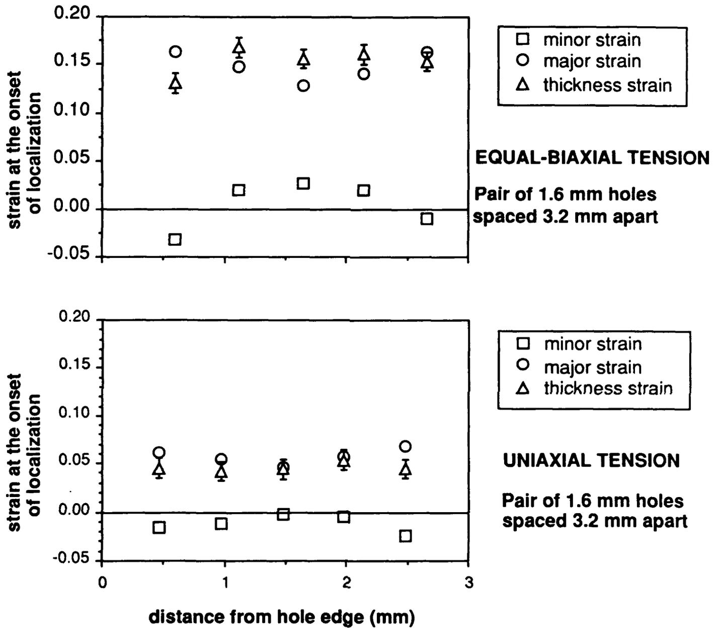
Figure 3: The dependence of the local principal strain components at the onset of ligament localization as a function of the distance from the hole edge for specimens tested in either uniaxial or equal-biaxial tension.
