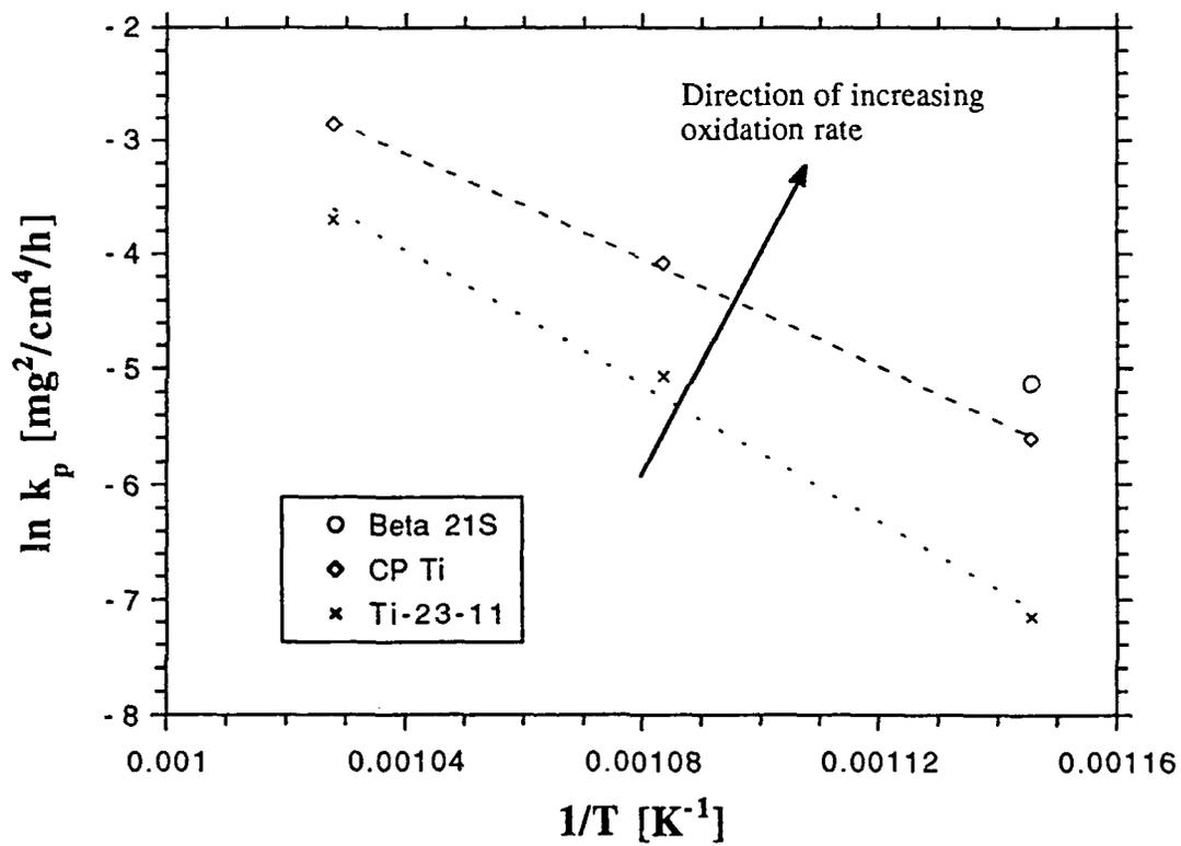
Figure 11. Arrhenius plot of parabolic rate constants of Beta21S, CP Ti, and Ti-23Nb-11Al. Note: Slopes yield the apparent activation energy for oxidation.
