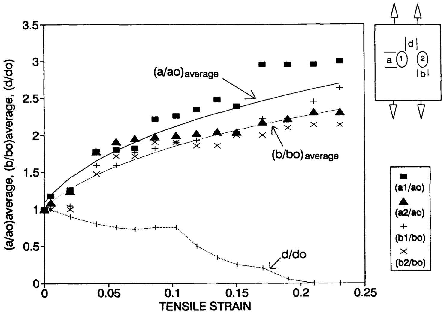
Figure 6. The effect of increasing plastic strain on the principal diameters (a,b) of an initially spherical void ( $a_0=b_0=c_0$ ) and on spacing ligament (d) between voids with an initially intervoid spacing ( $d_0$ ). The solid and dot lines represent the fitted curves of the average values " $a/a_0$  and  $b/b_0$ " respectively.
