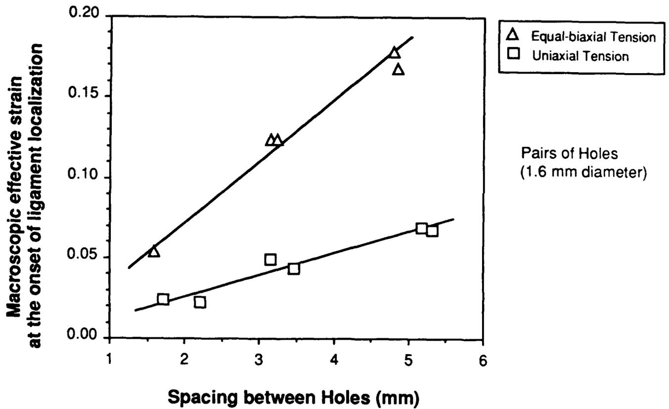
Figure 4: The dependence of the macroscopic, effective strain at the onset of ligament localization on the spacing between holes. Data is shown for both uniaxial and equal-biaxial tension.
