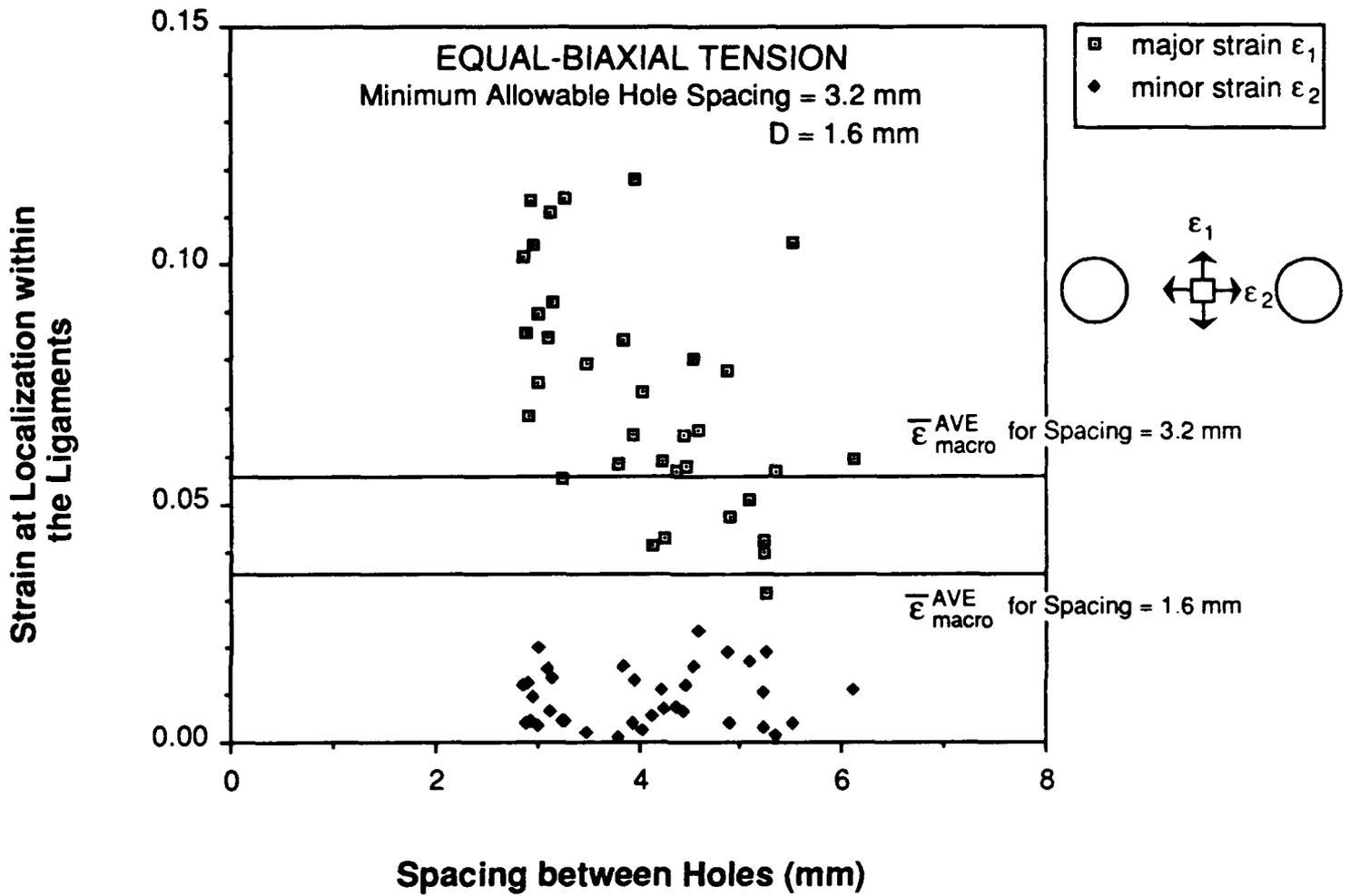
Figure 2: The dependence of the major and minor principal strains within the ligaments at localization as a function of interhole spacing for a "pseudo"-random array of 1.6 mm holes characterized by a minimum allowable hole spacing of 3.2 mm. The macroscopic, effective strains are also shown for specimens with both minimum allowable hole spacings used in the study.
