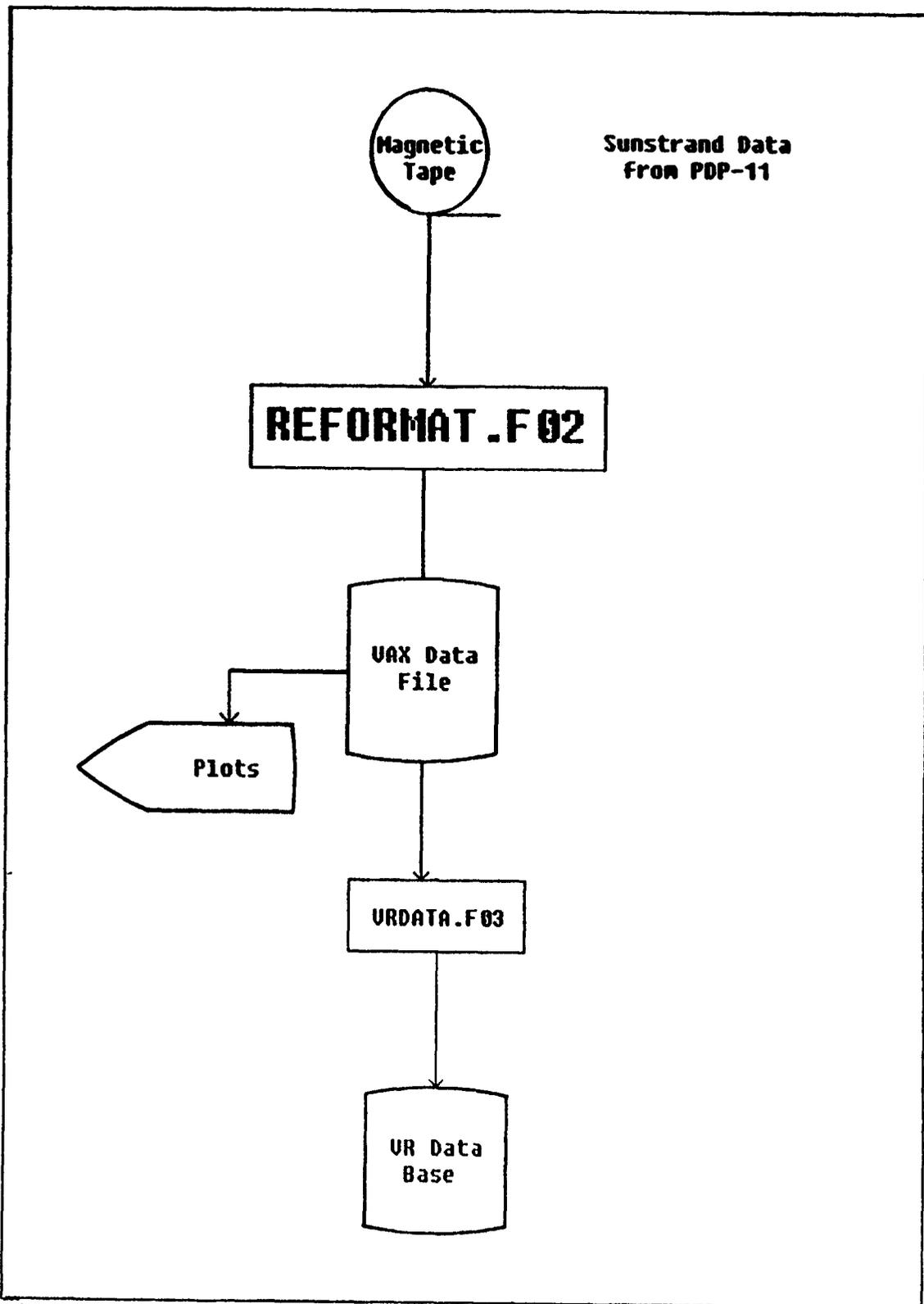
**Figure 4 - Flowchart of Visual Radiometer Database Generation**
