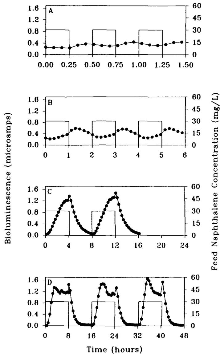
Figure 14. Bioluminescence response to square-wave perturbations in naphthalene feed concentration (rate): (A) 0.5-hour cycle; (B) 2-hour cycle; (C) 8-hour cycle; and (D) 16-hour cycle. (●) Bioluminescence and (—) Naphthalene feed concentration. Perturbation cycles were repeated at each frequency to demonstrate the reproducibility of the bioluminescent response. The results are representative of two independent experiments.
