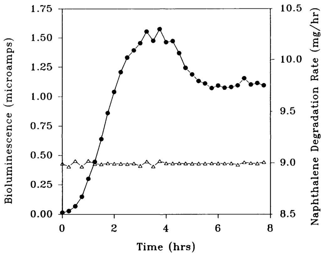
Figure 13. Induction of bioluminescence of strain HK44(pUTK21) in continuous culture: (●) bioluminescence and (Δ) naphthalene degradation rate. Data represents single time-point determinations and three results are representative of three independent experiments.
