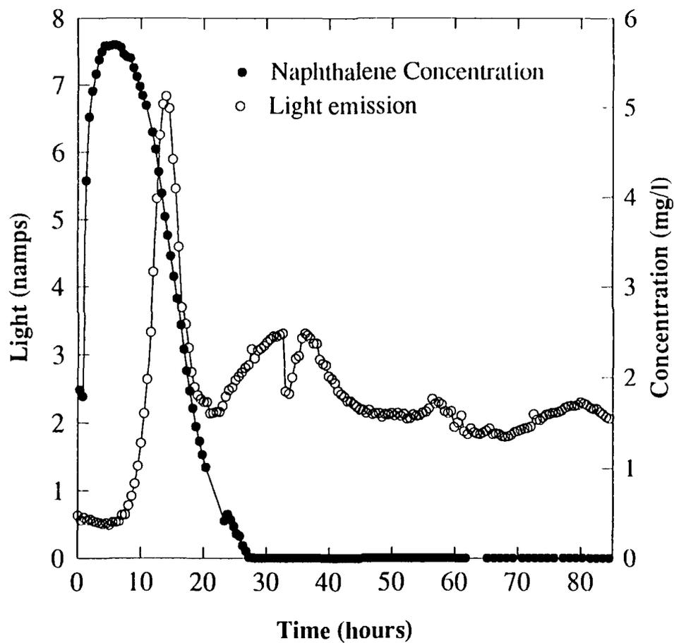
Figure 18. Light emission from strain HK44 and naphthalene effluent concentration from the differential volume reactor.
