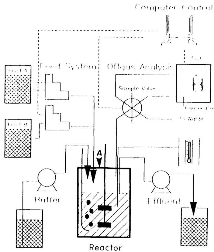
Figure 1. A schematic drawing of the bioreactor system for on-line studies of naphthalene degradation and light production by bioluminescent reporter strains. The port for liquid light pipe detection of bioluminescence is shown in A.
