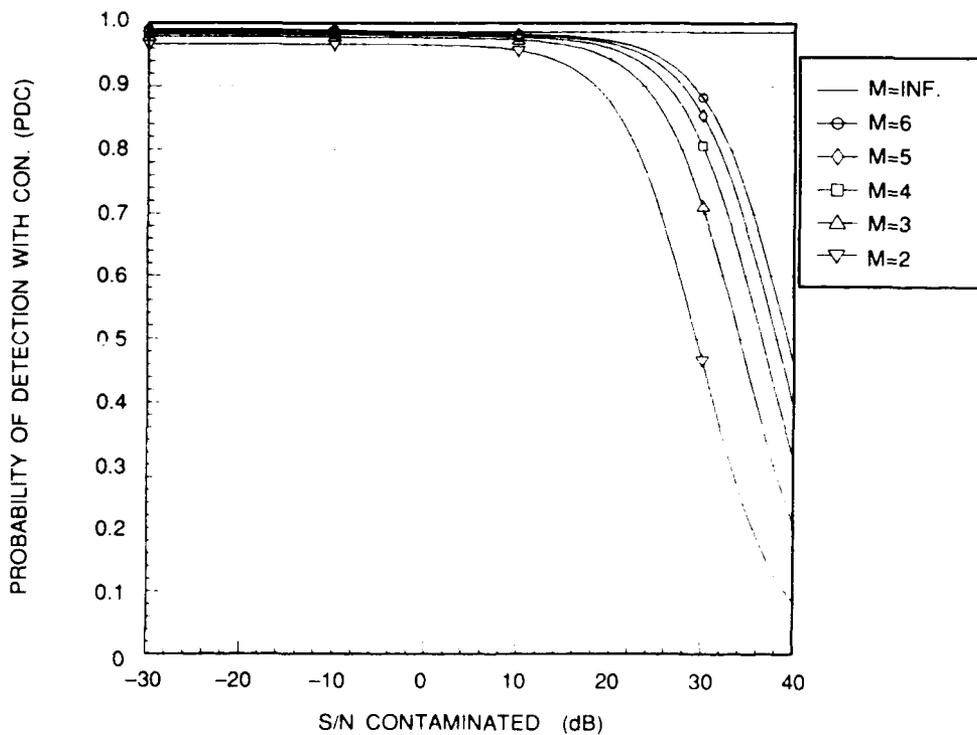
Fig. 13 -- Kelly detector:  $PD$  contaminated  $N = 30$ ,  $PF = 1.D-6$ ,  $S/N$  opt = 30 dB
