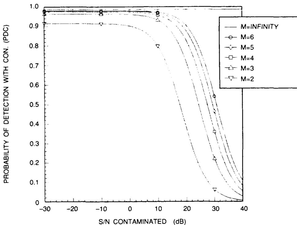
Fig. 12 -- Kelly detector:  $PD$  contaminated  $N = 5$ ,  $PF = 1.D-6$ ,  $S/N$  opt = 30 dB
