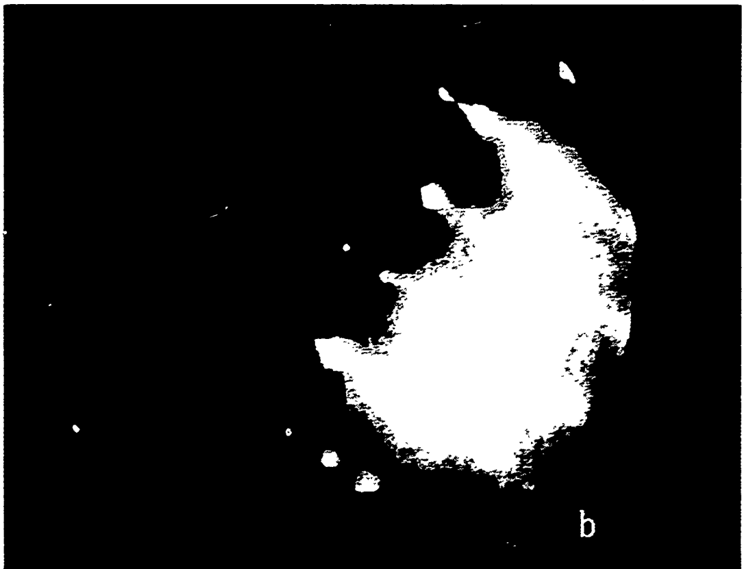
Figure 8. RHEED pattern of a GaN film grown on (0001) a-SiC by ALE. a) [01\bar{1}0] , b) [2\bar{1}10]
