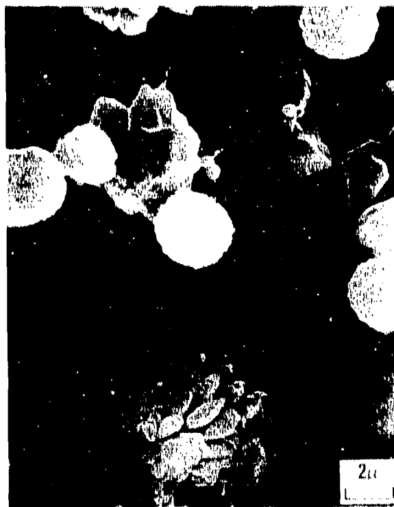
Figure 2. Residue of Pyrolyzed TATB Shows Similar Morphology and Chemistry as the Products Developed in Shocked TATB
