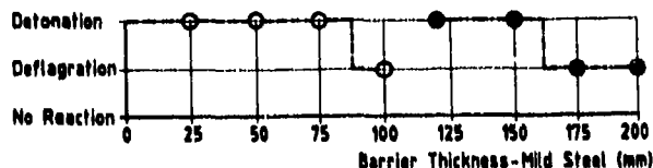
Figure 10. Type of Reaction as a Function of Barrier Thickness for Unconfined \circ and Confined \bullet Acceptor Charges
