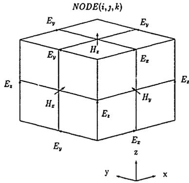
Figure 1: Field components in the FDTD unit cell.
