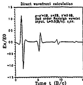
b) received signal constructed by multiple wavefront (ray field) tracking; multiple reflections are clearly resolved, with phase reversal after each reflection at the PEC.
