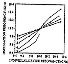
As the number of devices in the combiner increases, the oscillation frequency depends more on the devices and less on the periodicity
