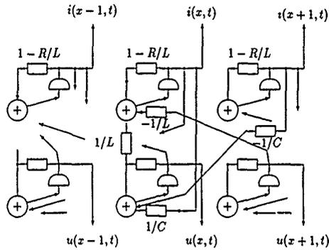
Figure 4: Digital model of the lossy transmission line.
