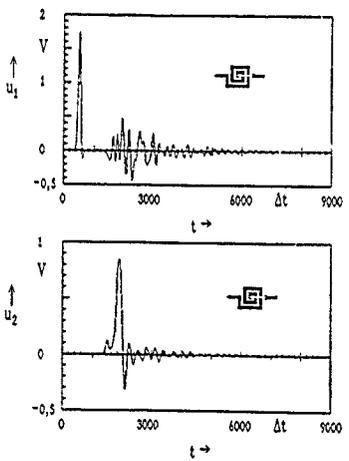
Voltage history at port 1 (left port) and port 2 (right port) of the spiral inductor.  $Al_2O_3$ ,  $\epsilon_r = 9.8$ , height = .635 mm, width = .625 mm, gap = .3125 mm, air-bridge diameter = .3125 mm.
