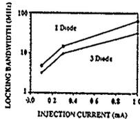
Multiple diode combiners require higher injection currents to obtain a given locking bandwidth
