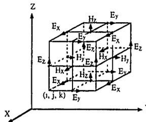
Fig 2b Yee's Finite Difference - Time Domain grid [2]
