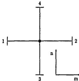
Figure 1: A two-dimensional TLM shunt node four-port.
